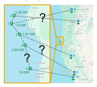
Figure 26: Location of buses, wind farm rated power, and candidate MTDC cables are shown. The wind farm area is enlarged on the left half.
