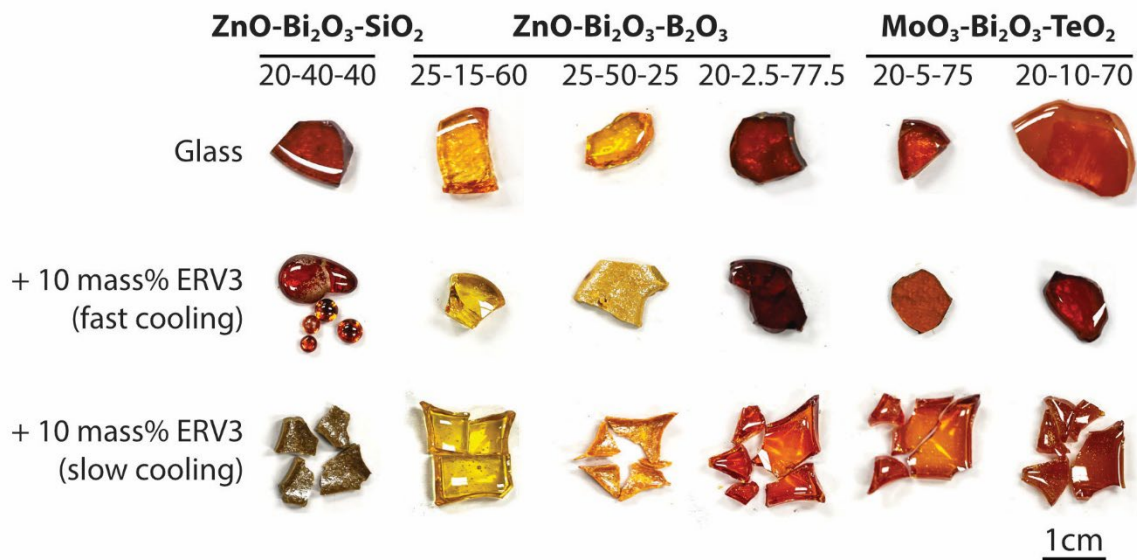
Figure 4-2. Images of glasses and samples with salt addition. Glass compositions are in mol%.
