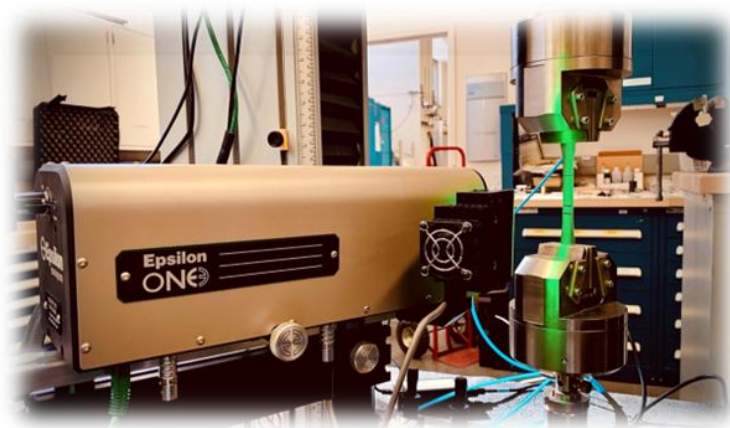
Figure 4. Noncontact extensometer setup.
