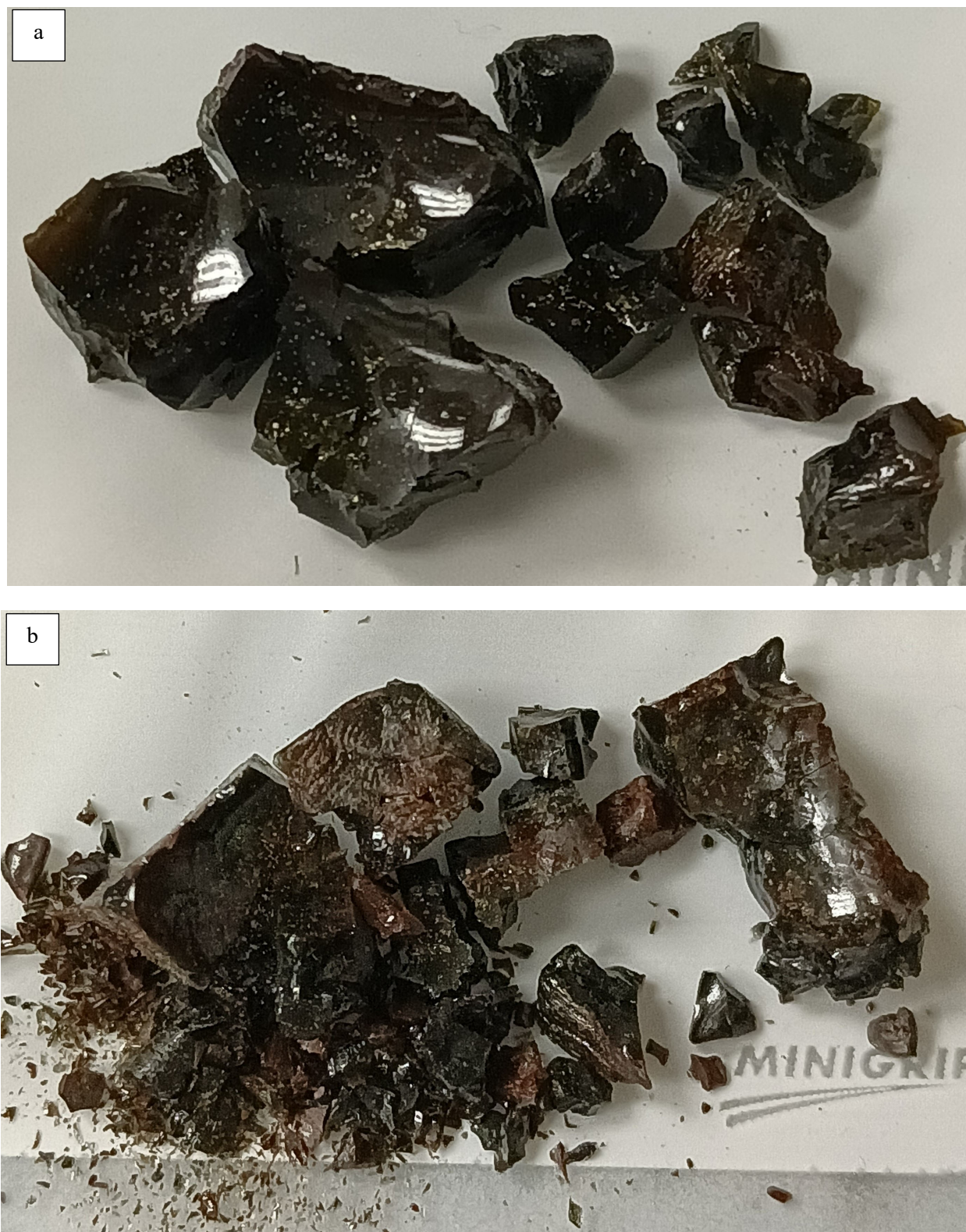
Figure H.2. Glass HAIG-02 after CF Heat Treatment at a) 950 °C for 24 h and b) 850 °C for 48 h
