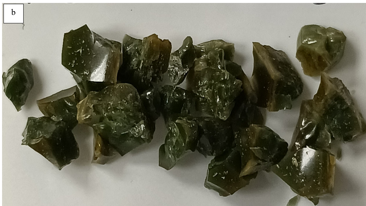
Figure H.22. Glass HAIG-23 after CF Heat Treatment at a) 950 °C for 24 h and b) 850 °C for 48 h
