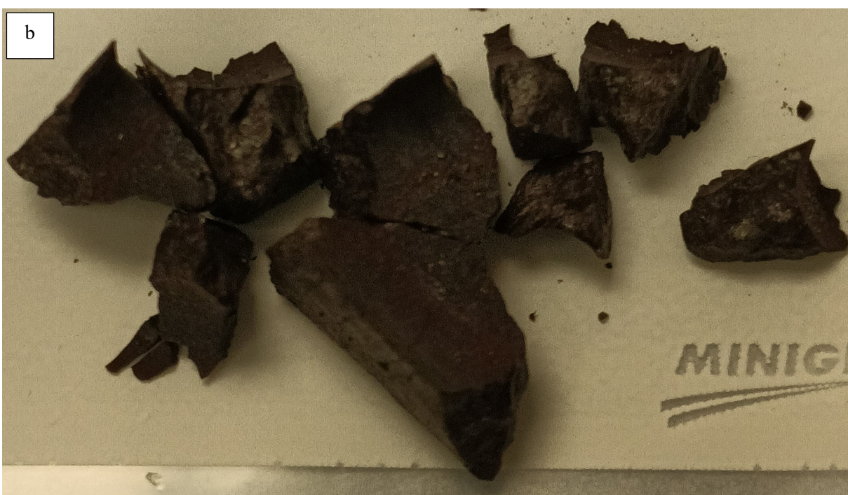
Figure H.12. Glass HAIG-13 after CF Heat Treatment at a) 950 °C for 24 h and b) 850 °C for 48 h
