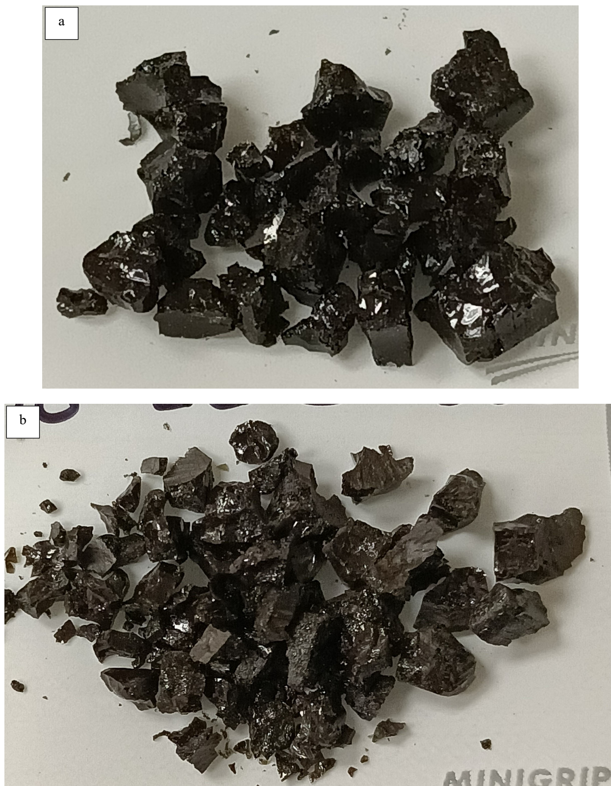
Figure H.21. Glass HAIG-22 after CF Heat Treatment at a) 950 °C for 24 h and b) 850 °C for 48 h
