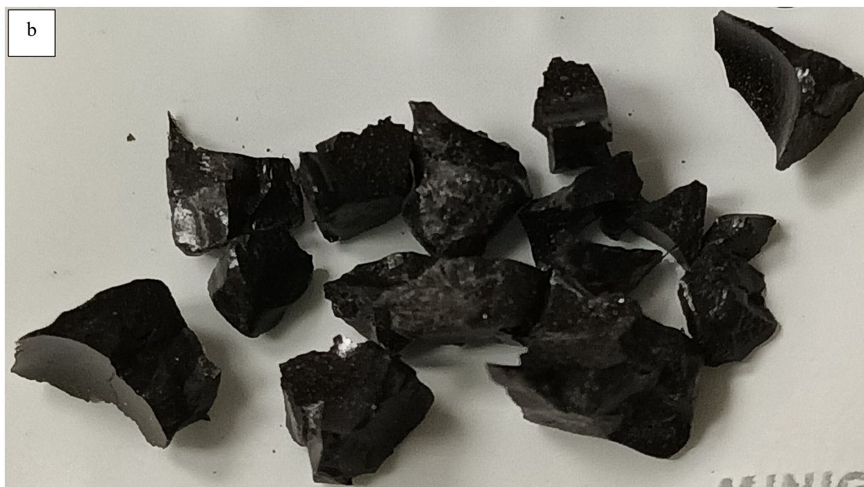
Figure H.5. Glass HAIG-05 after CF Heat Treatment at a) 950 °C for 24 h and b) 850 °C for 48 h
