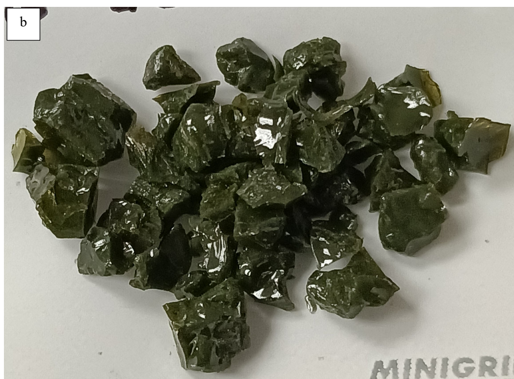
Figure H.19. Glass HAIG-20 after CF Heat Treatment at a) 950 °C for 24 h and b) 850 °C for 48 h
