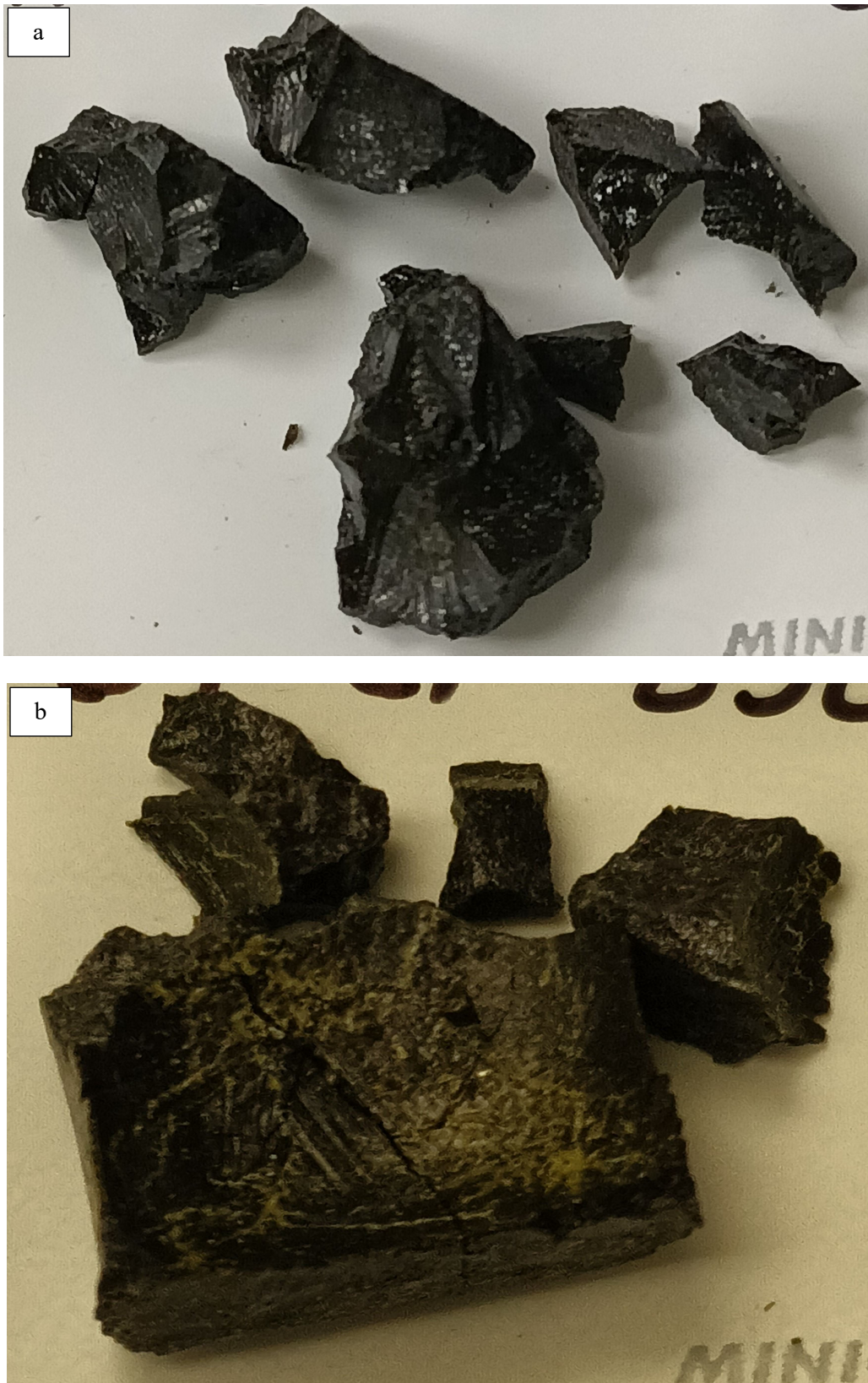
Figure H.4. Glass HAIG-04 after CF Heat Treatment at a) 950 °C for 24 h and b) 850 °C for 48 h
