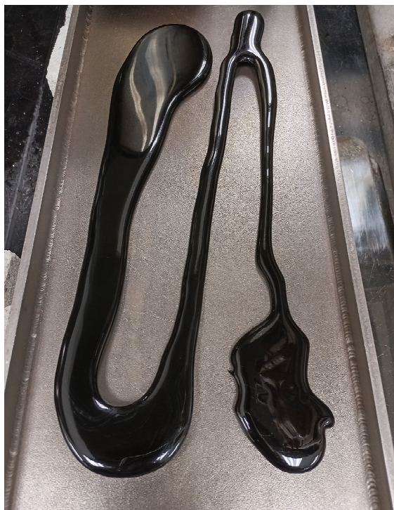
Figure A.24. Photo of Glass HAIG-24 Morphology of Second Melt Stirred at 1150 °C for 1 h
