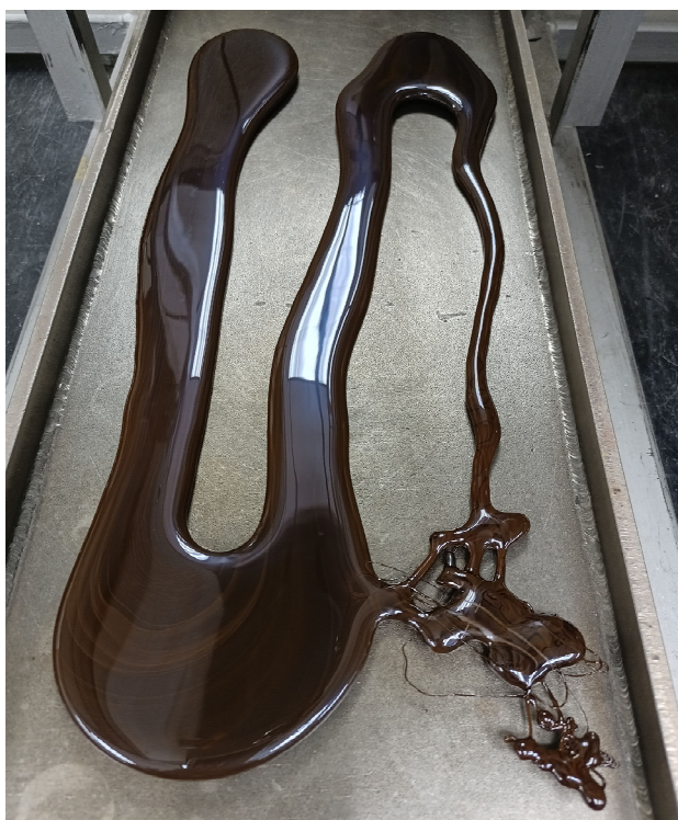
Figure A.19. Photo of Glass HAIG-19 Morphology of Second Melt Stirred at 1300 °C for 1 h
