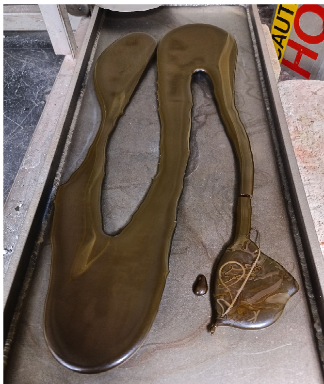
Figure A.11. Photo of Glass HAIG-11 Morphology of Third Melt at 1350 °C for 1 h
