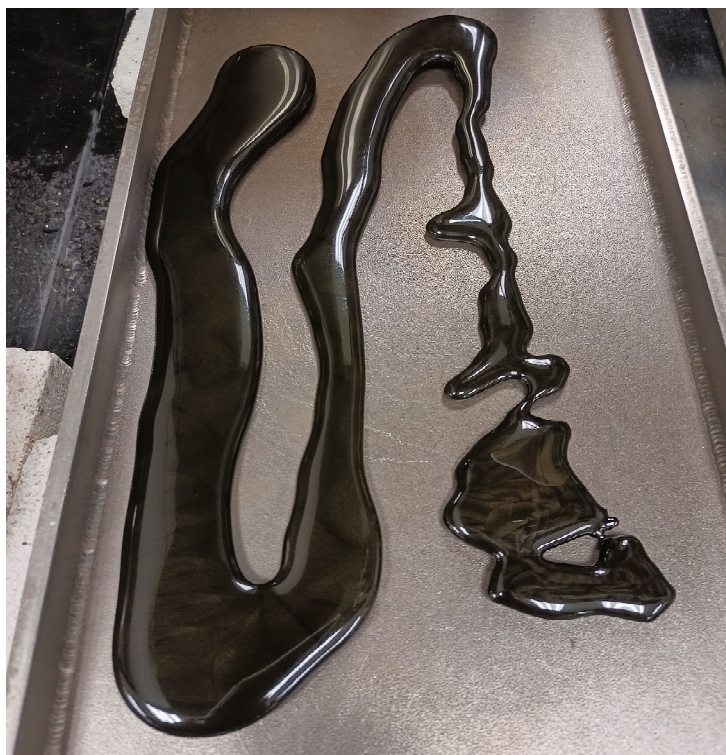
Figure A.25. Photo of Glass HAIG-25 Morphology of Second Melt Stirred at 1150 °C for 1 h
