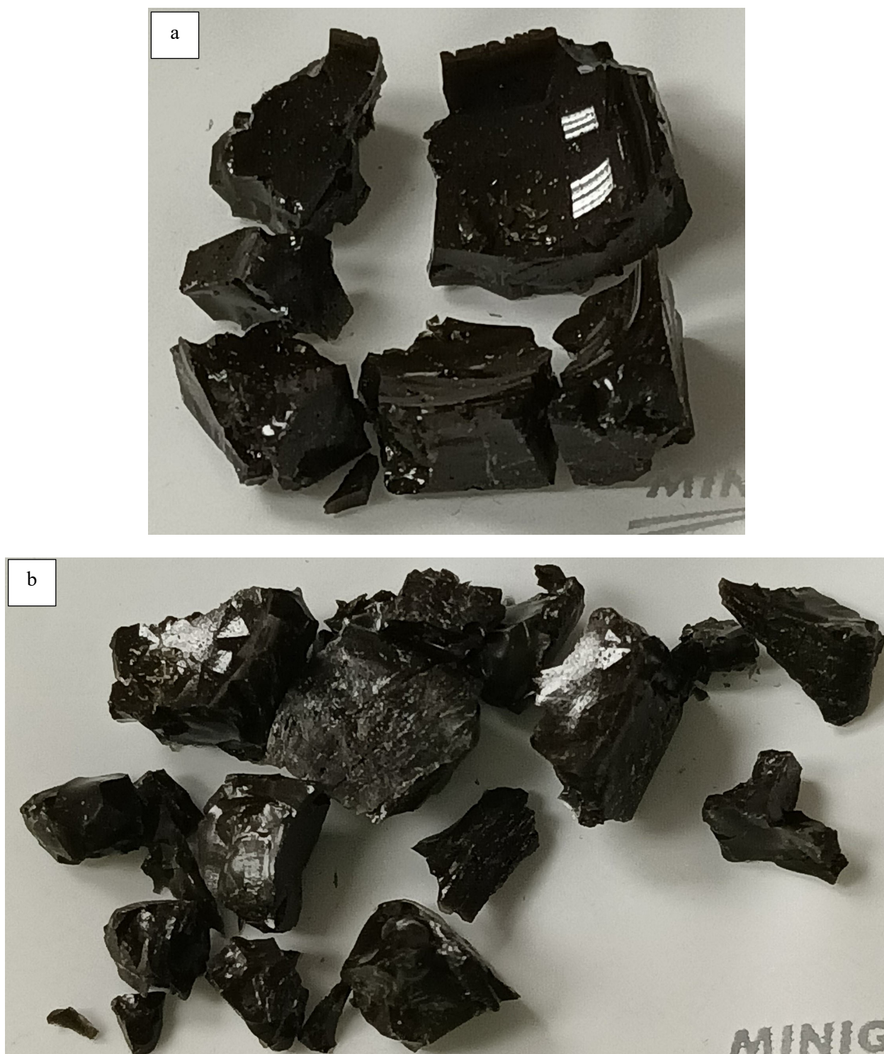
Figure H.6. Glass HAIG-06 after CF Heat Treatment at a) 950 °C for 24 h and b) 850 °C for 48 h
