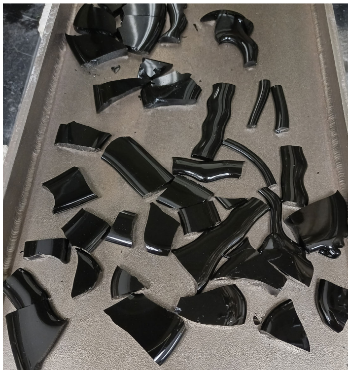
Figure A.4. Photo of Glass HAIG-04 Morphology of Second Melt at 1200 °C for 1 h
