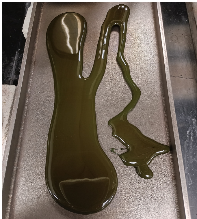
Figure A.20. Photo of Glass HALG-20 Morphology of Second Melt at 1150 °C for 1 h
