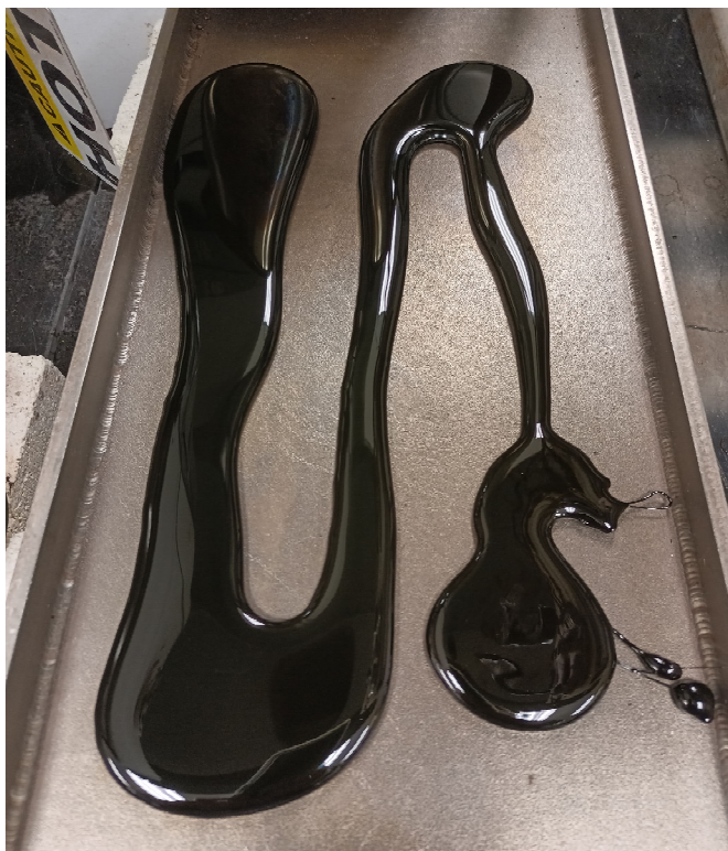
Figure A.14. Photo of Glass HAIG-14 Morphology of Second Melt Stirred at 1150 °C for 1 h
