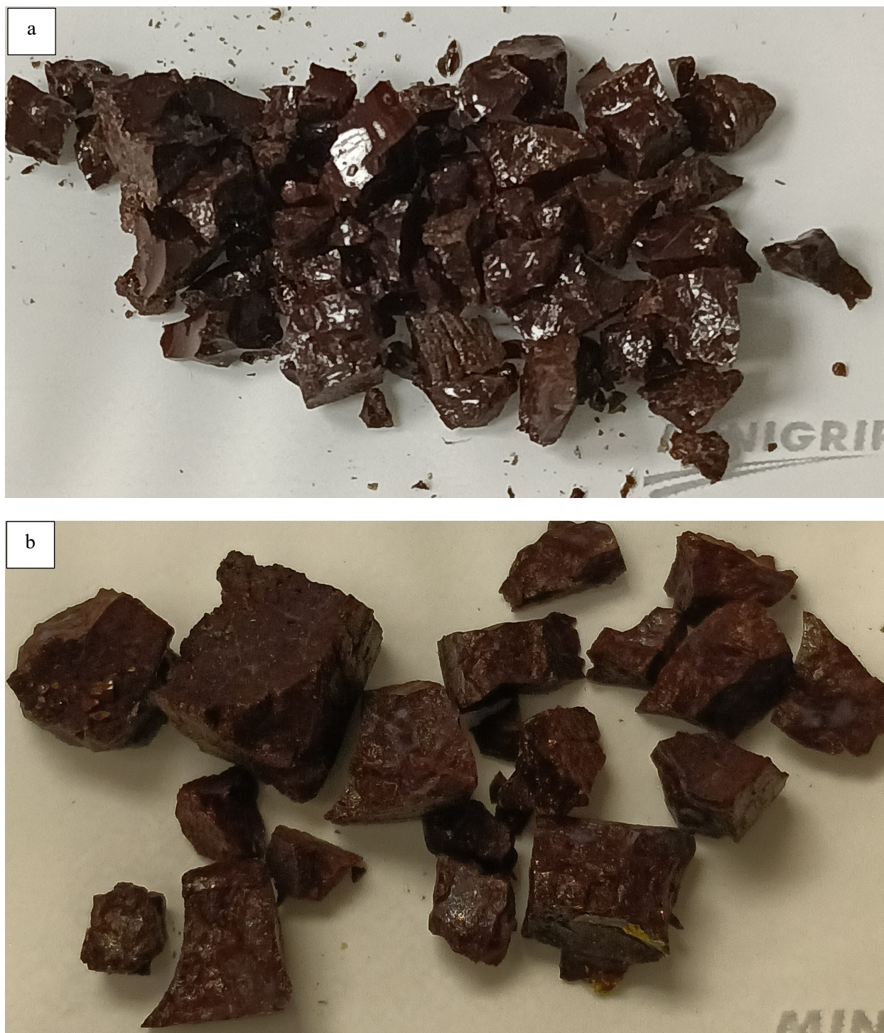
Figure H.18. Glass HAIG-19 after CF Heat Treatment at a) 950 °C for 24 h and b) 850 °C for 48 h
