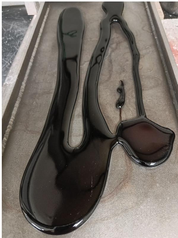
Figure A.1. Photo of Glass HAIG-01 Morphology of Third Melt at 1250 °C for 1 h
