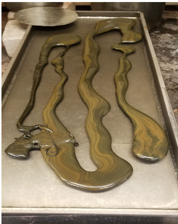
Figure A.18. Photo of Glass HAIG-18 Morphology of Third Melt at 1250 °C for 1 h
