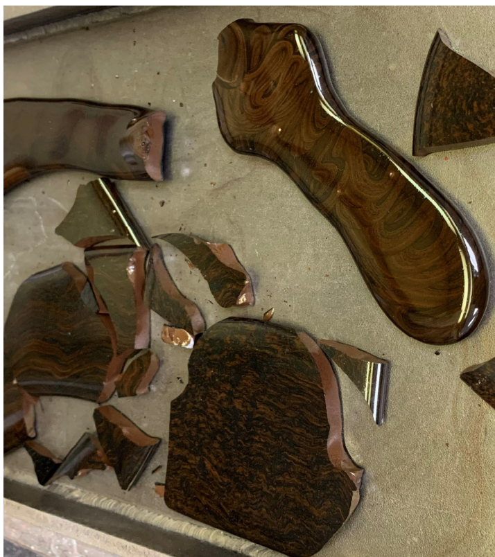
Figure A.5. Photo of Glass HAIG-05 Morphology of Second Melt at 1150 °C for 1 h
