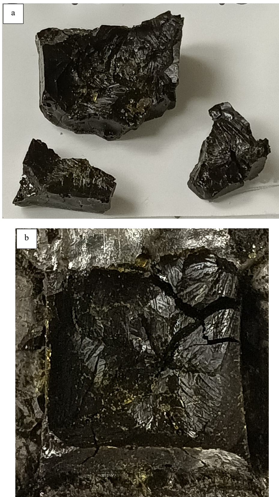
Figure H.14. Glass HAIG-15 after CF Heat Treatment at a) 950 °C for 24 h and b) 850 °C for 48 h
