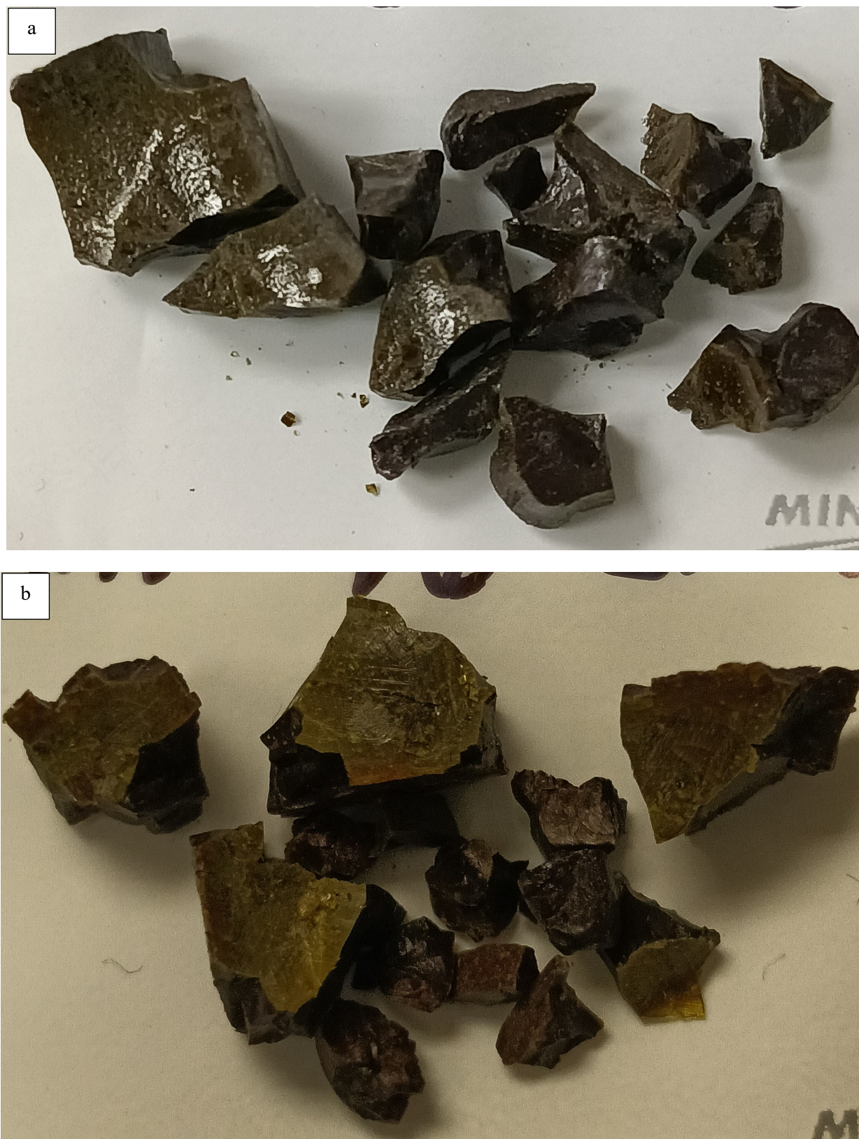
Figure H.15. Glass HAIG-16 after CF Heat Treatment at a) 950 °C for 24 h and b) 850 °C for 48 h
