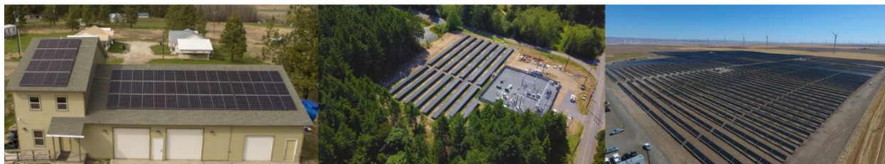
Figure 8. Residential solar installation on housing on the Spokane Indian reservation (left), community-scale solar that is part of the Decatur Island Microgrid project (504 kW; middle), and Lund Hill, a utility-scale photovoltaic plant in Klickitat, Washington (194 MW; right). Photo credits from left to right: DOE Office of Indian Energy Policy and Programs 2019, ( https://www.energy.gov/indianenergy/articles/doe-funded-solar-project-helps-spokane-tribe-reduce-homeowners-monthly-energy ), Opalco Energy, ( https://www.opalco.com/save/community-solar/decatour-island-microgrid-project/ ), and Iberdrola ( https://www.iberdrola.com/about-us/what-we-do/solar-photovoltaic-energy/lund-hill-photovoltaic-plant ).
