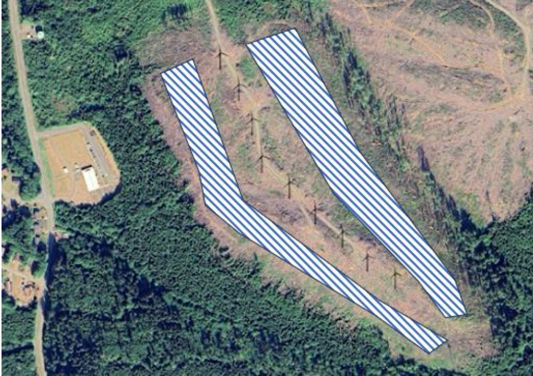
Figure 18. A potential layout for nine NPS 100C-21 turbines and 2-4 MW of ground-mount solar PV
