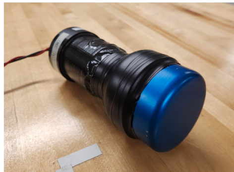
Figure 23. Photo of a CLYC detector used in pNRTA measurements at MIT.
