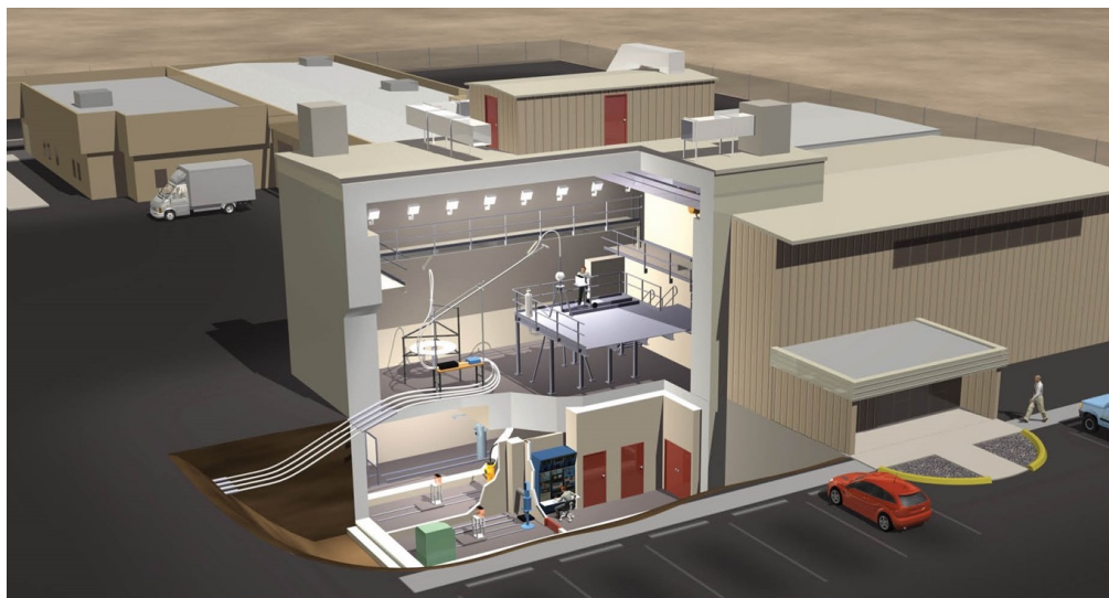
Figure 2. Cutaway view of the 318 Building REM Lab. The pNRTA experiments were setup on the raised platform near the center of the rendering.
