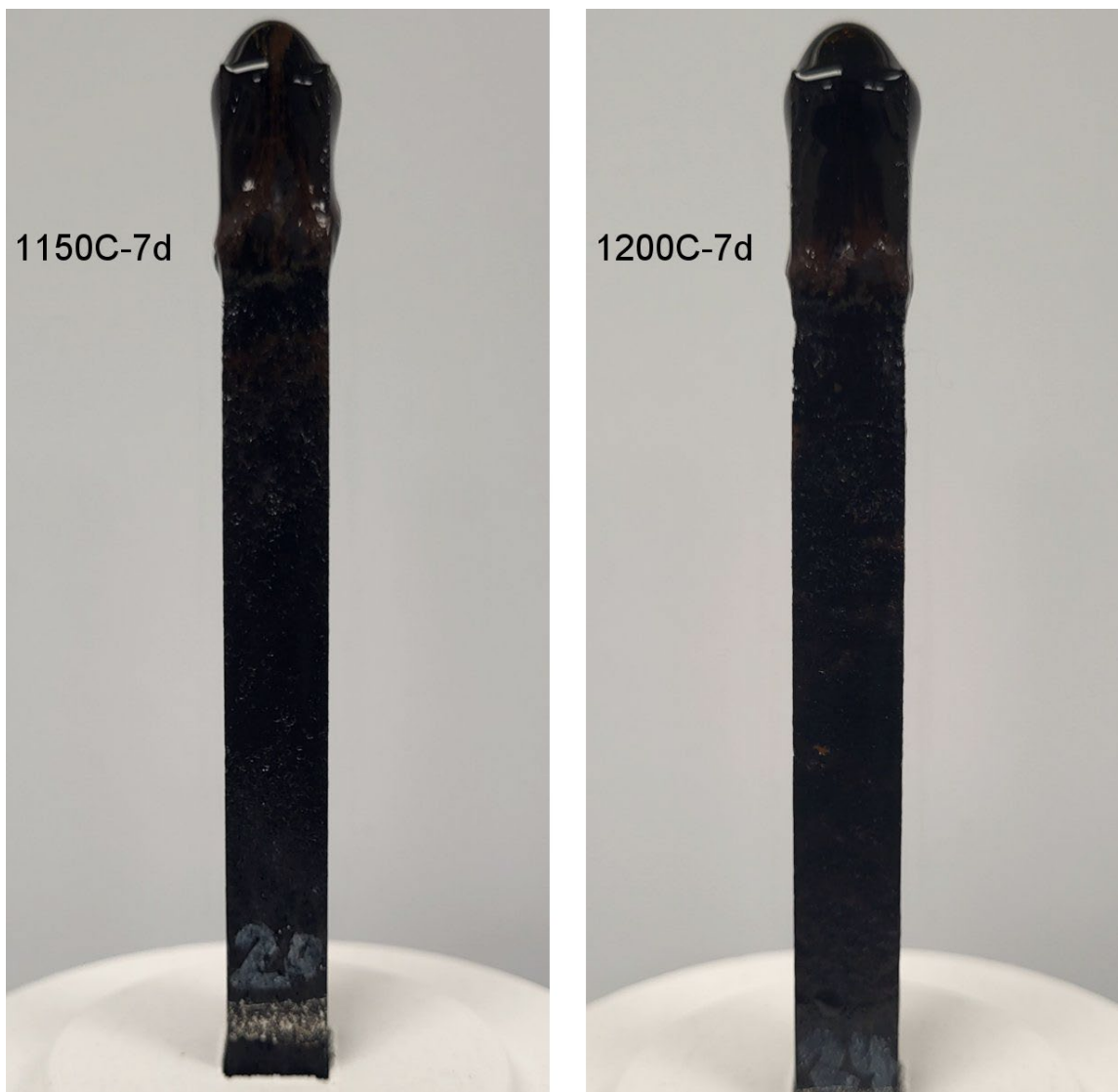
Figure A.12. K-3 coupons after refractory corrosion test, HAL24M2-12.
