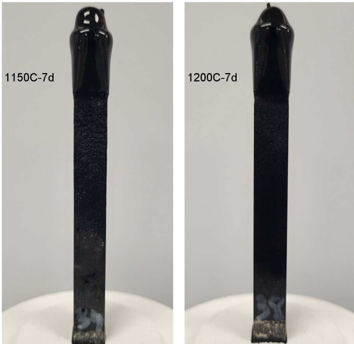
Figure A.18. K-3 coupons after refractory corrosion test, HAL24M2-18.
