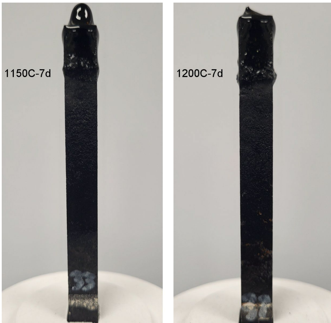
Figure A.17. K-3 coupons after refractory corrosion test, HAL24M2-17.
