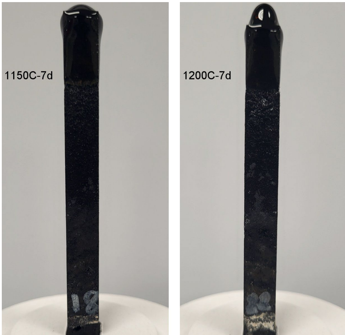
Figure A.10. K-3 coupons after refractory corrosion test, HAL24M2-10.
