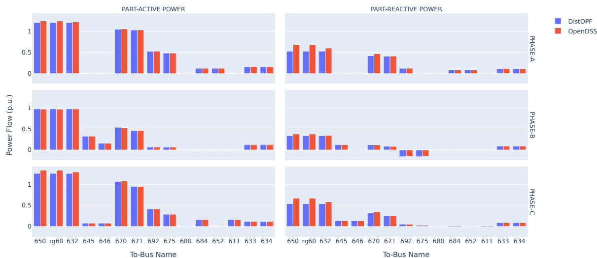
Figure 9. DistOPF branch power flow comparison with OpenDSS solutions for IEEE 13-Bus.
