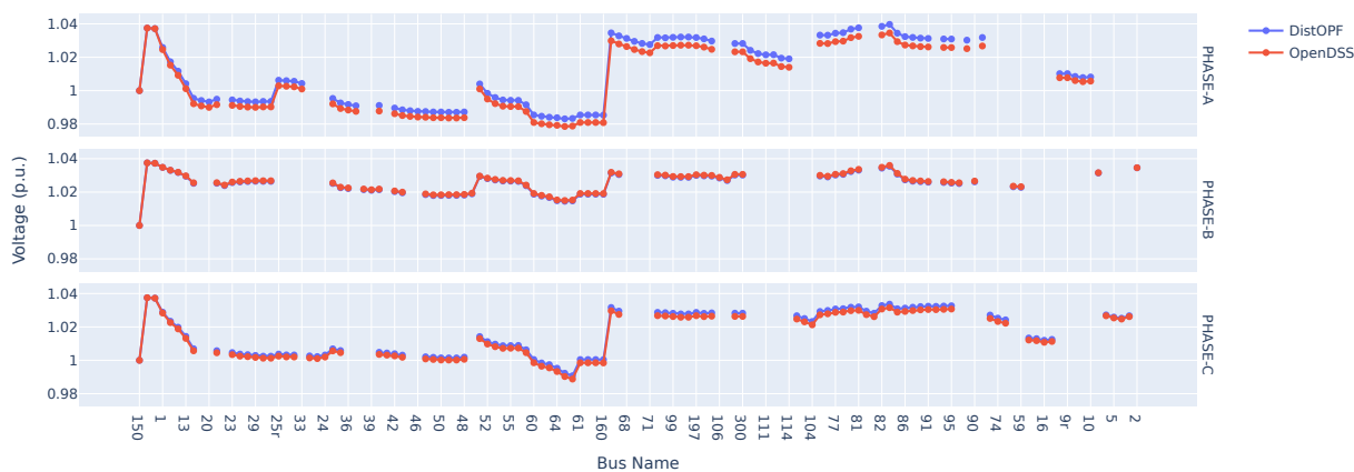
Figure 10. DistOPF voltage comparison with OpenDSS solutions for IEEE 123-Bus.
