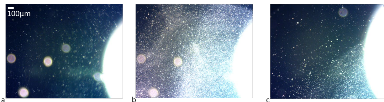
Figure 2. a) Darkfield micrograph, 500X, of micelles in deionized water. b) Darkfield micrograph, 500X, of the micelles mixed with the target particles. c) Darkfield micrograph, 500X, of the residual polymer/particle mixture adhered to the glass slide.
