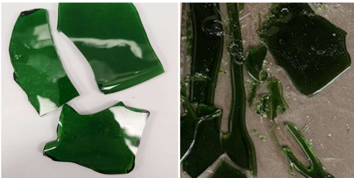
Figure A.2. Photographs of (left) APPS2-02 (1-kg batch) after the second melt using a Deltech furnace; (right) APPS2-02 (2-kg batch) after the second melt using a tilt-pour furnace.
