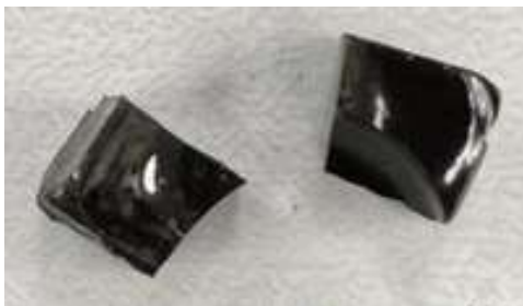
Figure E.9. Glass APPS2-09 after isothermal heat treatment at 950 °C for 24 h.
