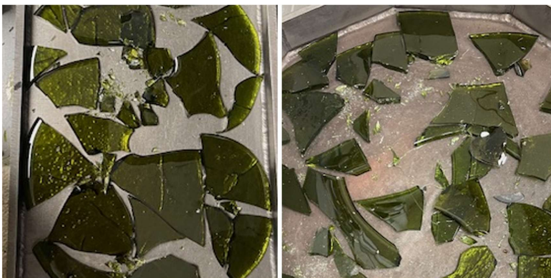
Figure A.6. Photographs of (left) APPS2-06 (1-kg batch) after the second melt using a Deltech furnace; (right) APPS2-06-1 (2-kg batch) after the first melt using a tilt-pour furnace.
