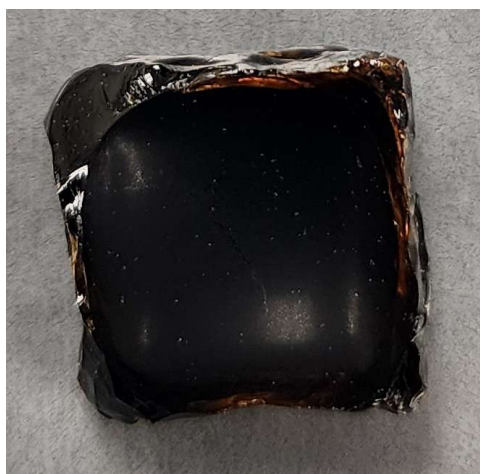
Figure E.7. Glass APPS2-07 after isothermal heat treatment at 900 °C for 24 h.
