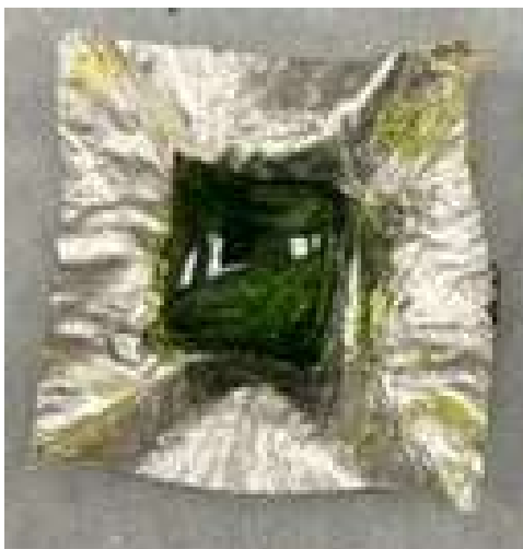
Figure E.11. Glass APPS2-11 after isothermal heat treatment at 900 °C for 24 h.
