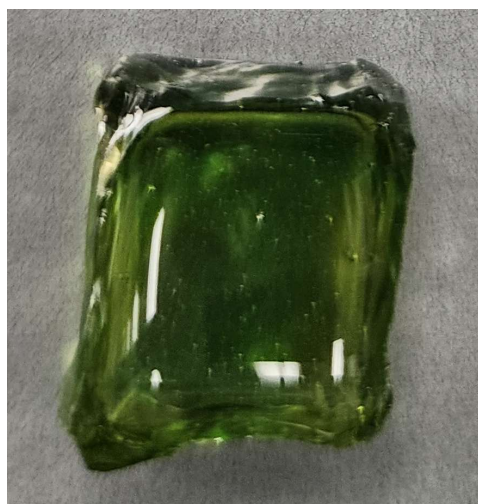
Figure E.2. Glass APPS2-02 after isothermal heat treatment at 900 °C for 24 h.
