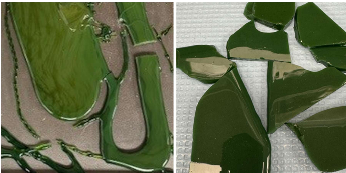
Figure A.11. Photographs of (left) APPS2-11 (1-kg batch) after the second melt using a Deltech furnace; (right) APPS2-11 (2-kg batch) after the first melt using a tilt-pour furnace.
