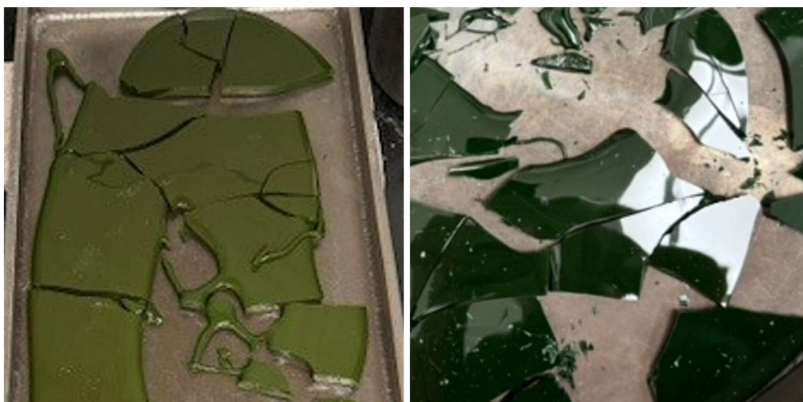
Figure A.10. Photographs of (left) APPS2-10 (1-kg batch) after the second melt using a Deltech furnace; (right) APPS2-10 (2-kg batch) after the first melt using a tilt-pour furnace.
