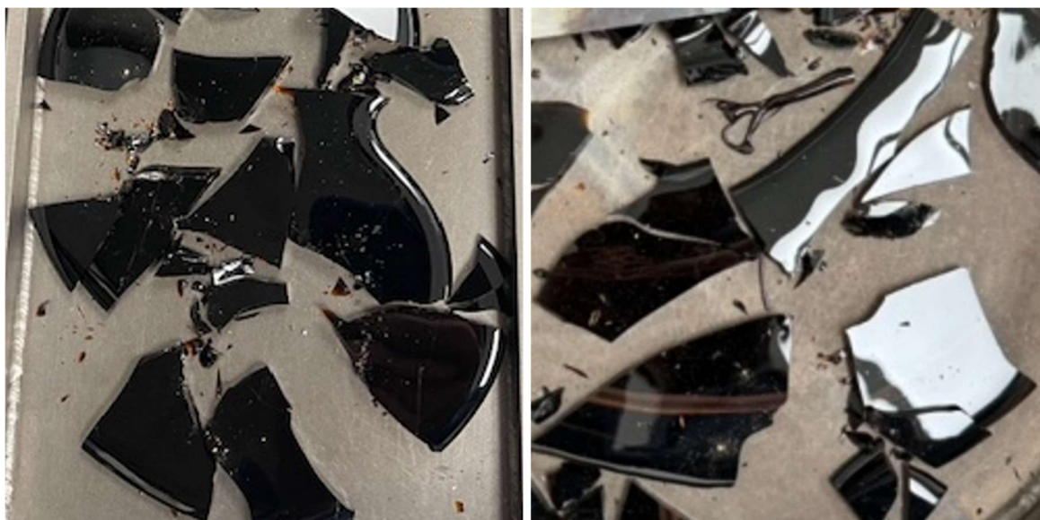
Figure A.9. Photographs of (left) APPS2-09 (1-kg batch) after the third melt using a Deltech furnace; (right) APPS2-09 (2-kg batch) after the first melt using a tilt-pour furnace.
