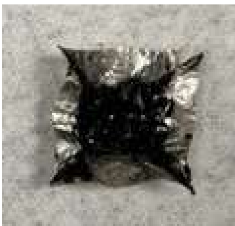
Figure E.4. Glass APPS2-04 after isothermal heat treatment at 900 °C for 24 h.
