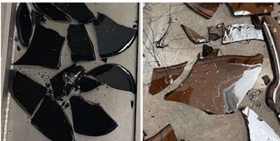
Figure A.8. Photographs of (left) APPS2-08 (1-kg batch) after the second melt using a Deltech furnace; (right) APPS2-08 (2-kg batch) after the first melt using a tilt-pour furnace.
