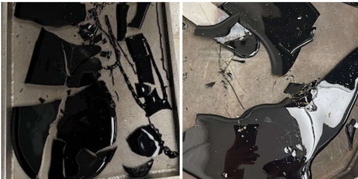
Figure A.7. Photographs of (left) APPS2-07 (1-kg batch) after the third melt using a Deltech furnace; (right) APPS2-07 (2-kg batch) after the first melt using a tilt-pour furnace.
