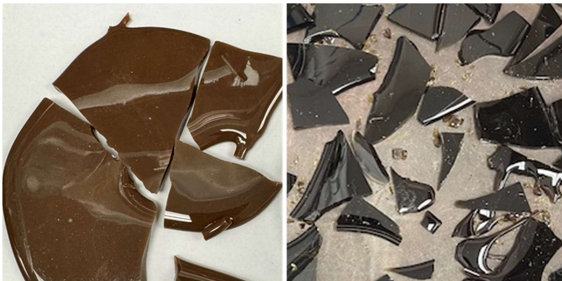
Figure A.3. Photographs of (left) APPS2-03 (1-kg batch) after the third melt using a Deltech furnace; (right) APPS2-03 (2-kg batch) after the first melt using a tilt-pour furnace.
