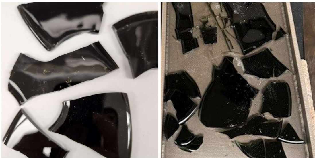
Figure A.5. Photographs of (left) APPS2-05 (1-kg batch) after the second melt using a Deltech furnace; (right) APPS2-05-1 (2-kg batch) after the second melt using a Deltech furnace.
