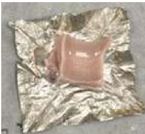
Figure E.12. Glass APPS2-12 after isothermal heat treatment at 900 °C for 24 h.
