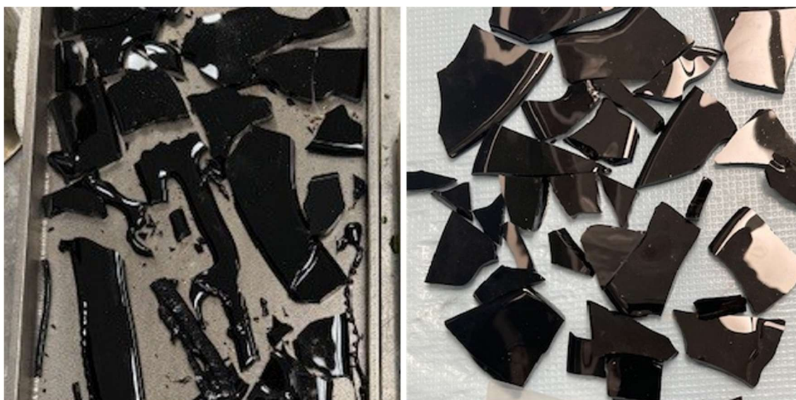
Figure A.4. Photographs of (left) APPS2-04 (1-kg batch) after the second melt using a Deltech furnace; (right) APPS2-04 (2-kg batch) after the first melt using a tilt-pour furnace.
