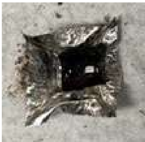
Figure E.5. Glass APPS2-05 after isothermal heat treatment at 900 °C for 24 h.
