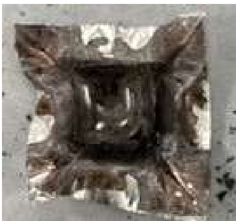
Figure E.14. Glass APPS2-14-1 after isothermal heat treatment at 900 °C for 24 h.
