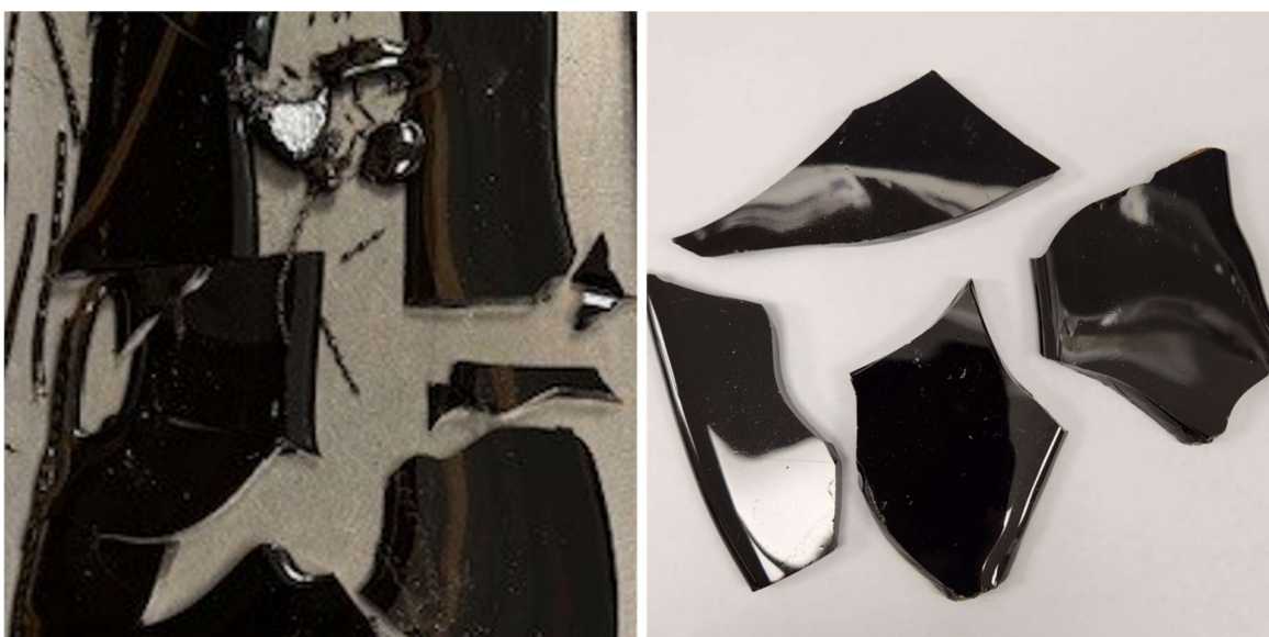
Figure A.14. Photographs of (left) APPS2-14-1 (1-kg batch) after the third melt using a Deltech furnace; (right) APPS2-14-1 (2-kg batch) after the first melt using a tilt-pour furnace.
