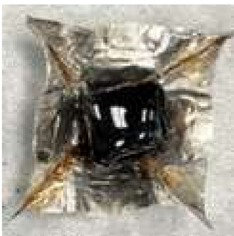
Figure E.16. Glass APPS2-16 after isothermal heat treatment at 900 °C for 24 h.
