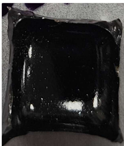
Figure E.8. Glass APPS2-08 after isothermal heat treatment at 900 °C for 24 h.
