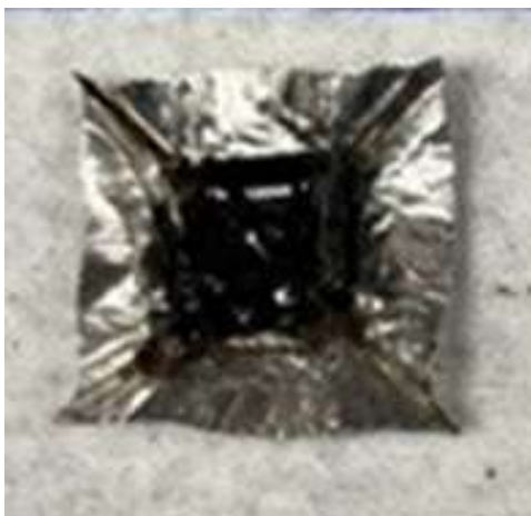
Figure E.1. Glass APPS2-01 after isothermal heat treatment at 900 °C for 24 h.
