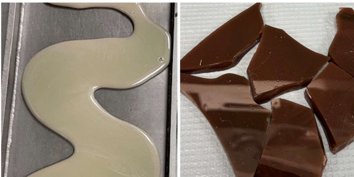
Figure A.12. Photographs of (left) APPS2-12 (1-kg batch) after the second melt using a Deltech furnace; (right) APPS2-12 (2-kg batch) after the first melt using a tilt-pour furnace.
