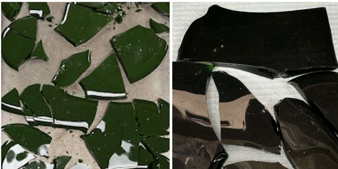
Figure A.15. Photographs of (left) APPS2-15 (1-kg batch) after the second melt using a Deltech furnace; (right) APPS2-15 (2-kg batch) after the first melt using a tilt-pour furnace.
