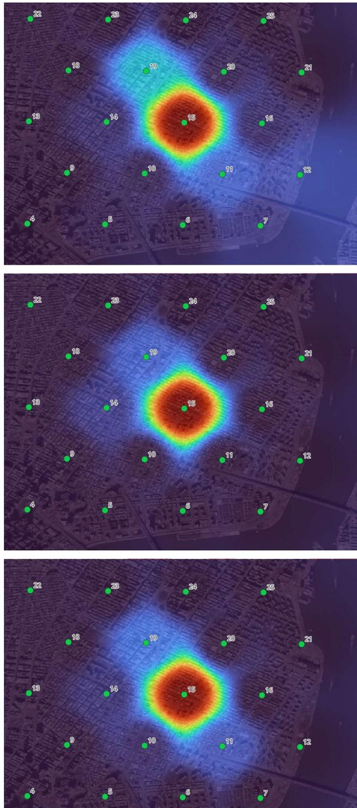
Figure 5.22. Systematic Sensor Placement, Ground Level, 41.5 Minutes after Release, At ground level (top), 12.5 meters (middle) and 37.5 meters (bottom)
