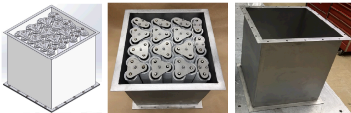
Figure 6-7. Lawrence Livermore National Laboratory ceramic high-efficiency particulate absorbing (HEPA) filter design and prototype showing the as-fabricated Class 9 ceramic HEPA filter prototype including (left) design model, (middle) top of filter elements, and (right) side view of the housing prior to assembly (Haslam 2019).
