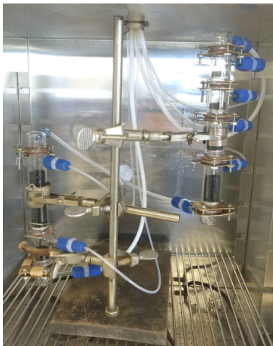
Figure 4-4. Picture of solid sorbent testing column at Oak Ridge National Laboratory for evaluating capture of long-chain organic iodides on silver mordenite ( \text{Ag}^0\text{Z} ) (Bruffey et al. 2019).
