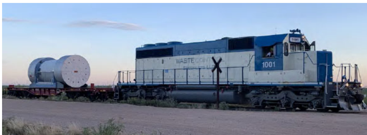
Figure 2-16: MP197HB Transportation Cask on Rail at WCS Low Level Radioactive Waste Disposal Facility (Photo Courtesy of Orano)
