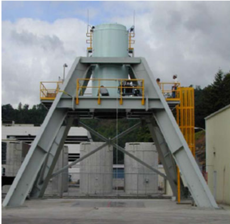
Figure 2-26: Example of a Transfer Station (used at Trojan with modified HI-TRAC) [13]
