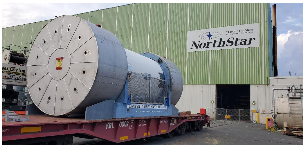
Figure 3-2: MP197HB Used to Make Shipments to WCS (Orano Provided)
