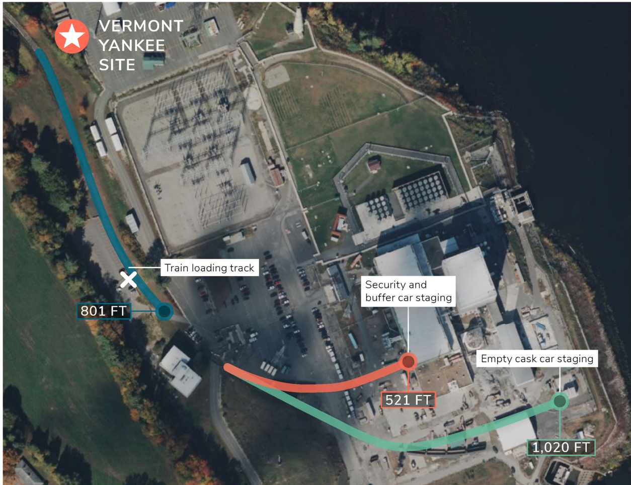
Figure 3-3: VY On-Site Rail
