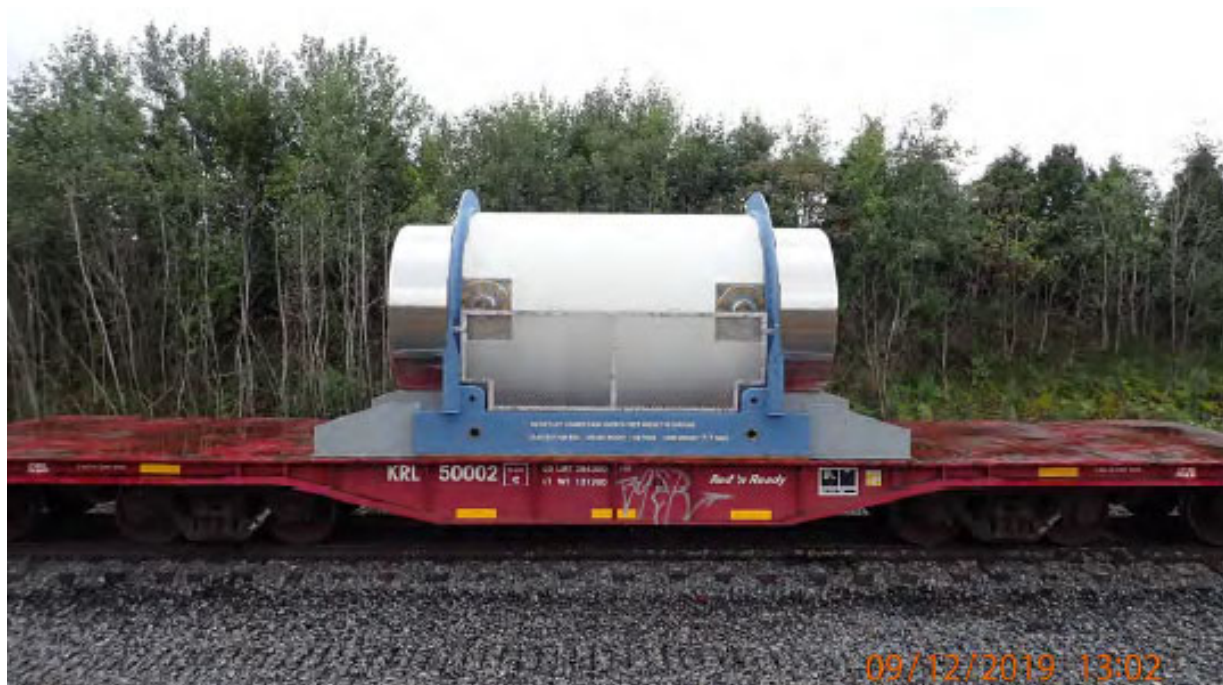
Figure 2-15: MP197HB Transportation Cask without Impact Limiters on Rail Prior to Shipping at VYNPS (Photo Courtesy of Orano)
