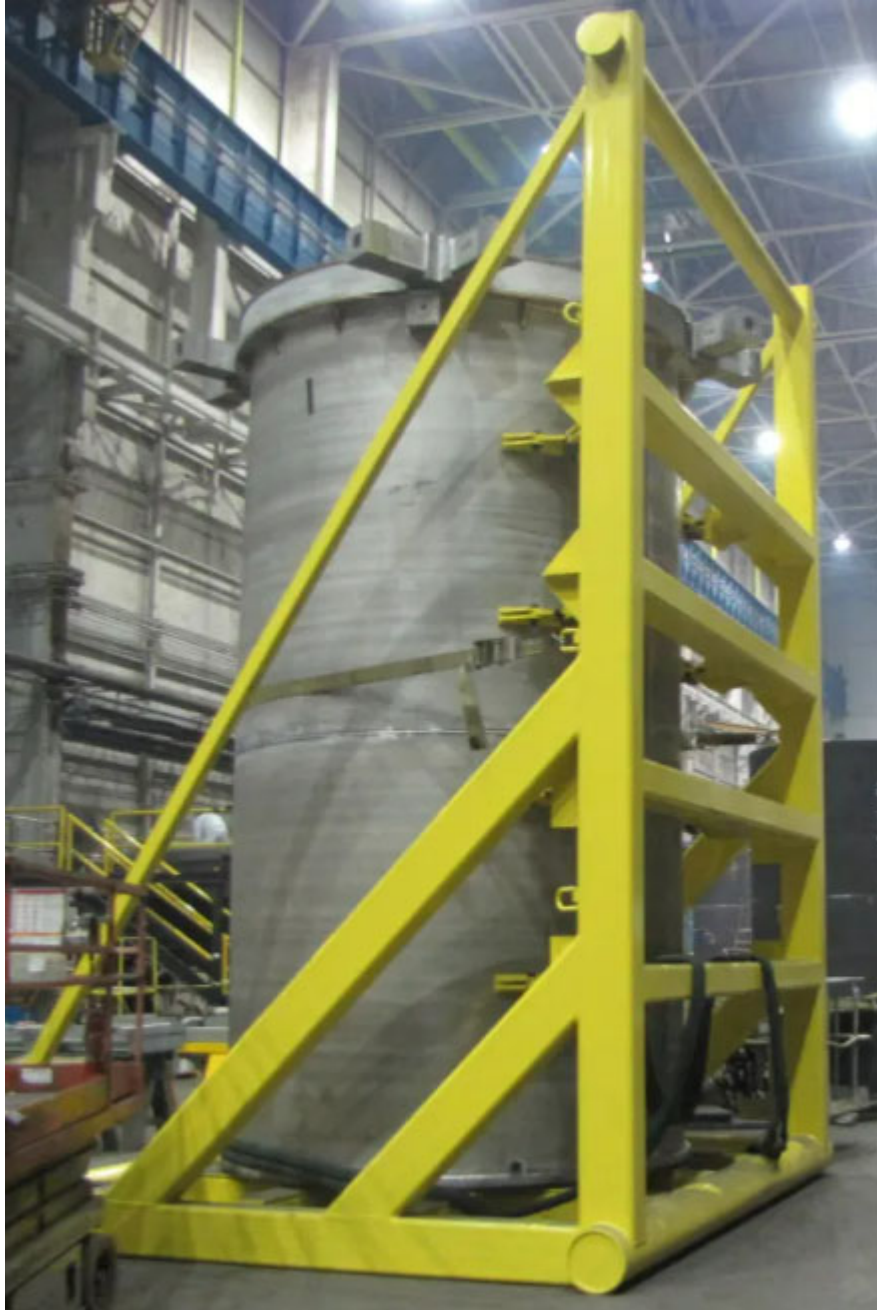
Figure 2-35: Example of Holtec Variable Elevation Cask Pedestal (Up-/Down-ENDER) [43]
