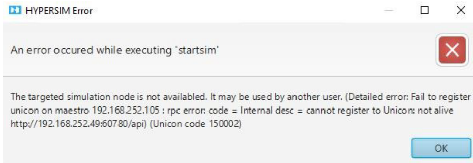
Figure 18: Screenshot of HYPERSIM error message indicating a failed simulation start due to bugs in the management of HYPERSIM TCP connections.
