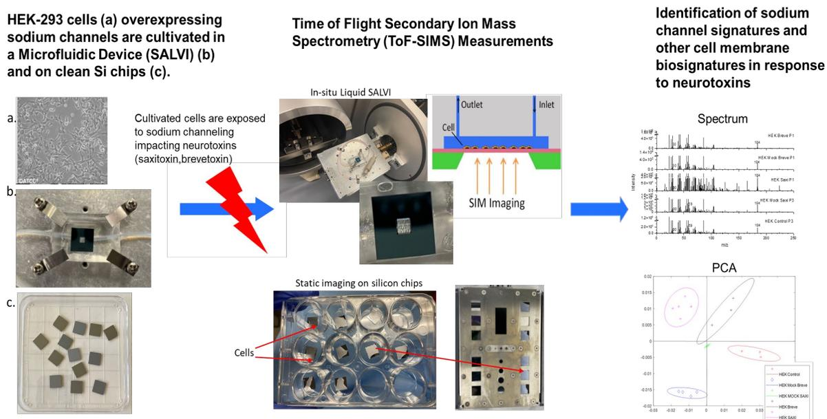
**Figure 1. Overview of scientific approach for chemical imaging for in situ detection of neurotoxins with static ToF-SIMS with dried cells and liquid in-situ ToF-SIMS analysis with a System for Analysis at the Liquid Vacuum Interface (SALVI).**
