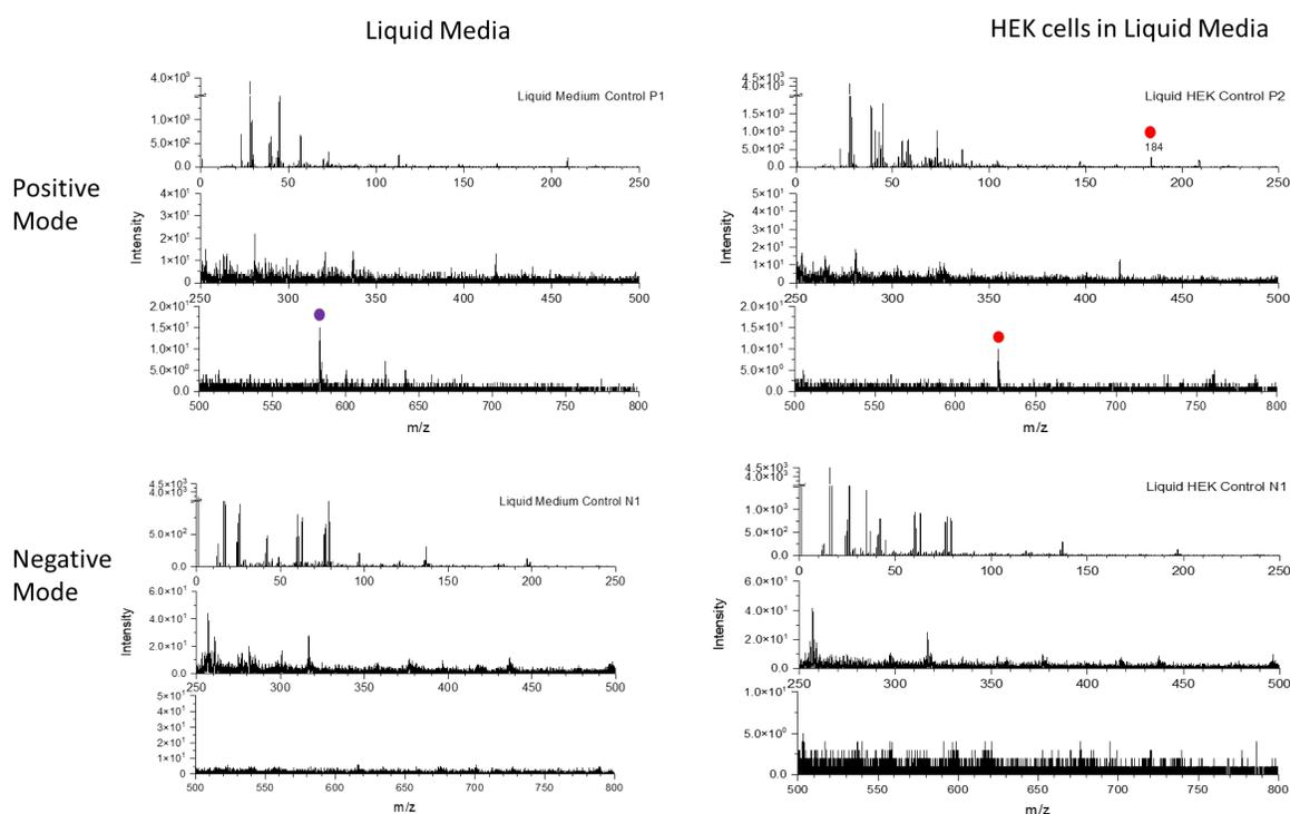
Figure 3. In situ ToF-SIMS of SALVI with liquid media or HEK cells. The data represents a single SALVI device for each treatment. The spectra from 20 – 800  $m/z$  from both positive and negative mode are shown. The red dots indicate unique spectra found in HEK cell SALVI and purple dot indicate unique spectra found in liquid media.
