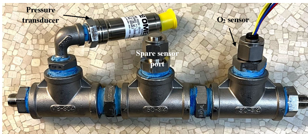
Figure 4. The gas sensing chamber with pressure transducer and oxygen sensor installed. The center port is empty and can be instrumented with an additional sensor per experiment needs.
