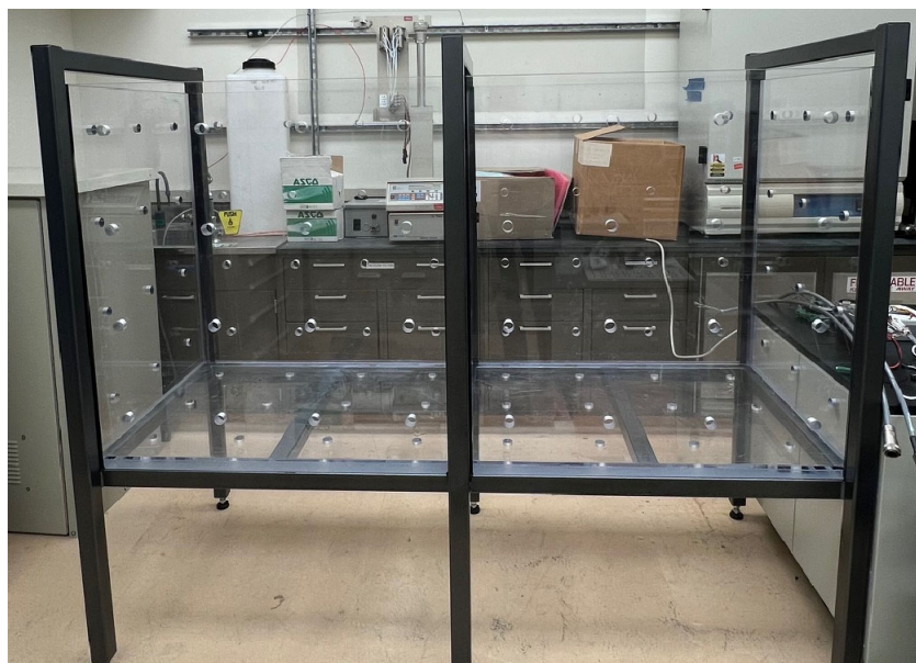
Figure 1. The assembled GIFT test cell, consisting of a plexiglass tank on a steel frame.
