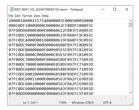
The CSV file begins with Sensor Fish Mini settings in the first two rows, while measurement data starts from the fourth row. The file comprises 9 columns: time, voltage, Acc\_x, Acc\_y, Acc\_z, Acc, Pressure, Gyro\_x, Gyro\_y, Gyro\_z, Gyro, and Temperature.
