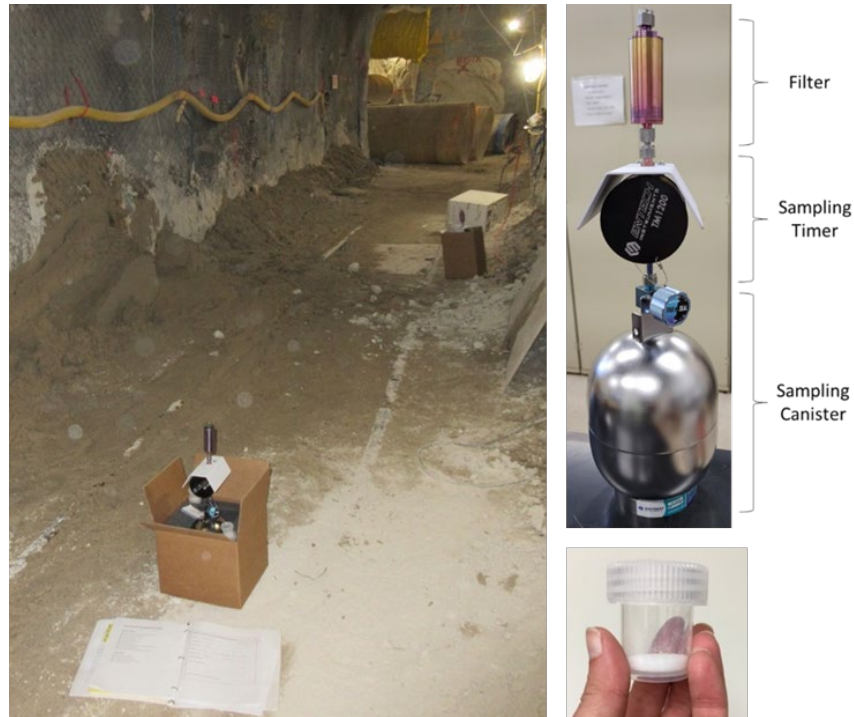
Figure 31. Photograph showing (left) the emplacement of a small volume gas sampler and liquid absorbents in the tunnel drift, (upper right) the small volume gas sampler system configuration, and (lower right) an example liquid absorbent sample.
