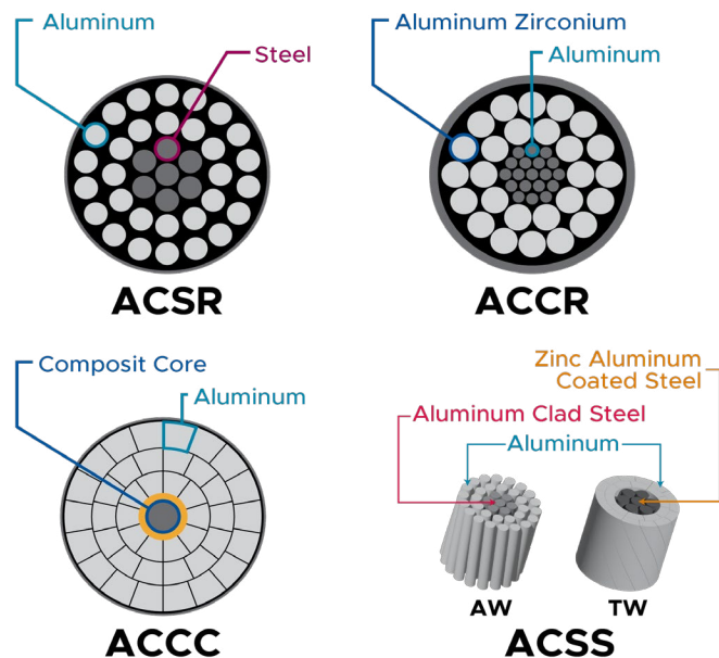
Figure 7. Cross-sections of transmission conductors. TOP LEFT: ACSR, TOP RIGHT: ACCR, BOTTOM LEFT: ACCC, BOTTOM RIGHT: ACSS, annealed wire and trapezoidal wire types.
