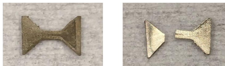
Figure 41: Neutron irradiated nanocrystalline nickel sample (2.6 dpa; KGT 246) before and after tensile testing.
