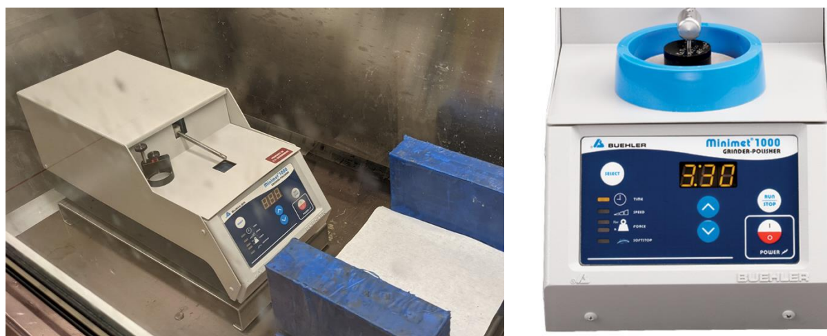
Figure 11: Buehler MiniMet 1000 utilized for neutron irradiated sample preparation.
