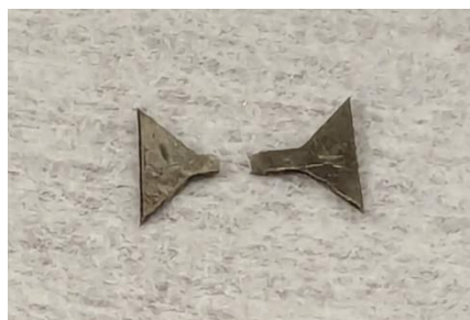
Figure 37: A representative neutron irradiated microcrystalline nickel sample (1.2 dpa; KGT 113) before and after tensile testing.
