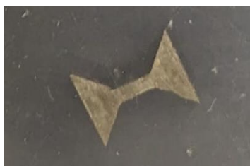
Figure 37: A representative neutron irradiated microcrystalline nickel sample (1.2 dpa; KGT 113) before and after tensile testing.
