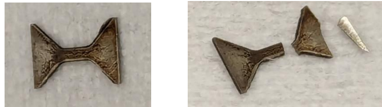
Figure 40: Neutron irradiated nanocrystalline nickel sample (1.2 dpa; KGT 112) before and after tensile testing
