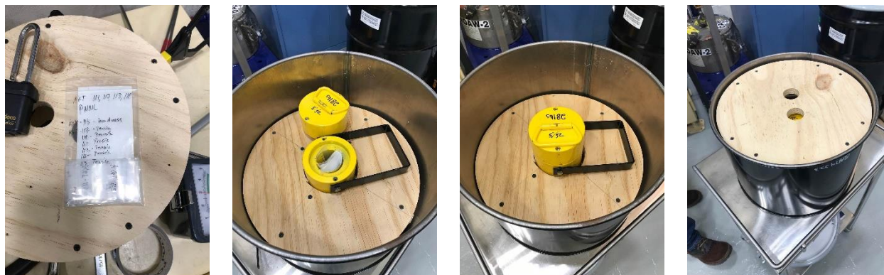
Figure 18: Photographs of irradiated nickel samples (placed individually inside Ziplock bags) packaged inside a pig that was placed inside a shipping drum.
