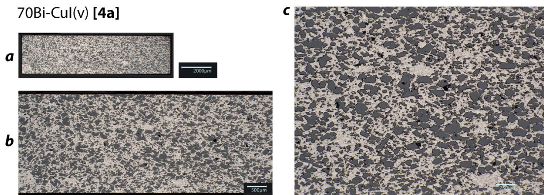
Figure 4-36. Cross-sectional optical micrographs of two-phase set-4 pellet of 70Bi-CuI(v) [4a] taken at (a) 20 \times , (b) 50 \times , and (c) 100 \times magnifications. This pellet was fired under vacuum at 203 ^{\circ} C for 20 h in the vacuum oven.
