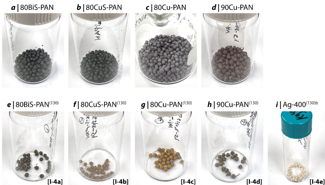
Figure 4-8. Pictures of iodine loading set-4 (a-d) before and (e-i) after iodine loading including (a) 80BiS-PAN, (b) 80CuS-PAN, (c) 80Cu-PAN, (d) 90Cu-PAN, (e) 80BiS-PAN (130) , (f) 80CuS-PAN (130) , (g) 80Cu-PAN (130) , (h) 90Cu-PAN (130) , and (i) Ag-400 (130) b. Details for iodine loading and sample designations shown in the figure are provided in Table 4-3.
