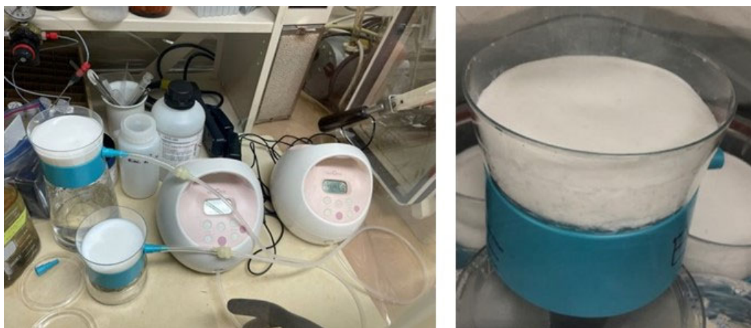
Figure E.3. Attempt #3: Rinsing and filtering the Sn(II)-PO 4 (left) and the resulting solid (right).
