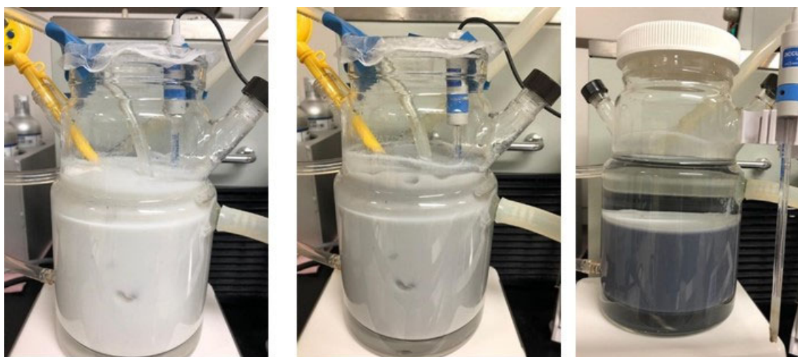
Figure E.1. \text{Sn(II)-PO}_4 synthesis attempt #1 at 2:09 p.m. (left), 2:40 p.m. (middle), and overnight (right). Photos show the progression to a gray color and the discolored and broken pH probe (notice discoloration and missing tip) on the right.
