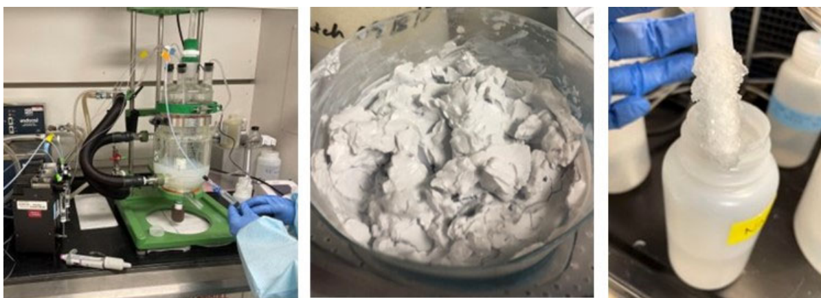
Figure E.2. Attempt #2: A ChemGlass reactor was used (left); the produced solid may have had a grayish tint (center); solid formation on the \text{N}_2 sparging line in the \text{Na}_2\text{HPO}_4 solution.
