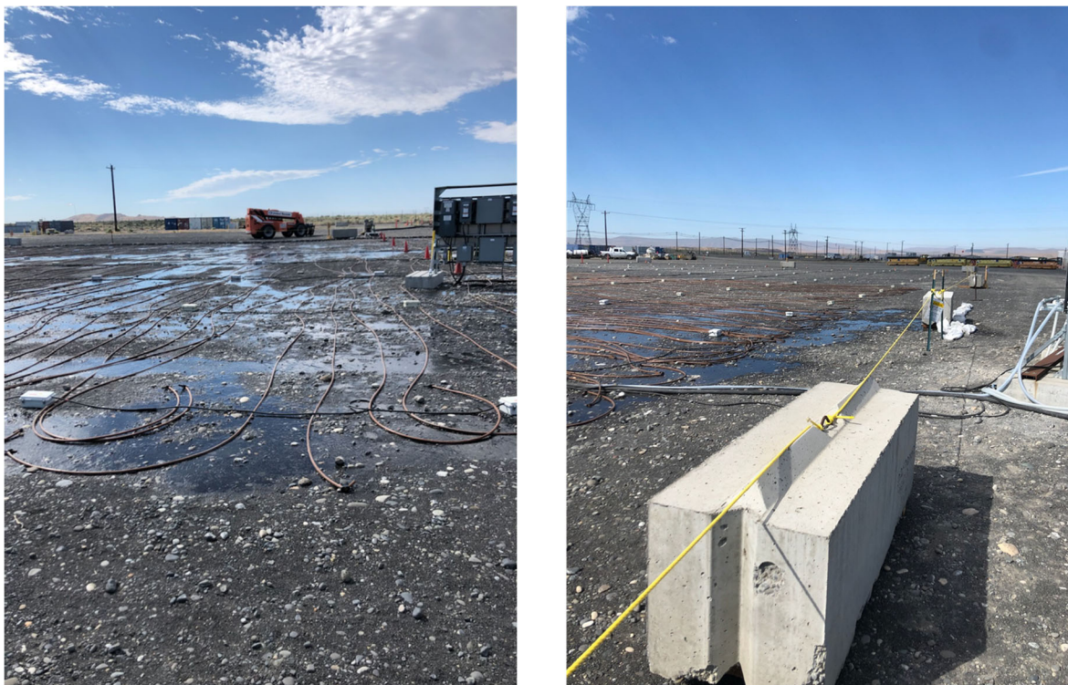
Figure 6. (left) Photograph taken during the first week of soil flushing, highlighting the distribution of flush water lines and shallow surface water ponding cause by slight variations in topography. (right) Photograph highlighting the ERT electrode array (white boxes connected by cables)
