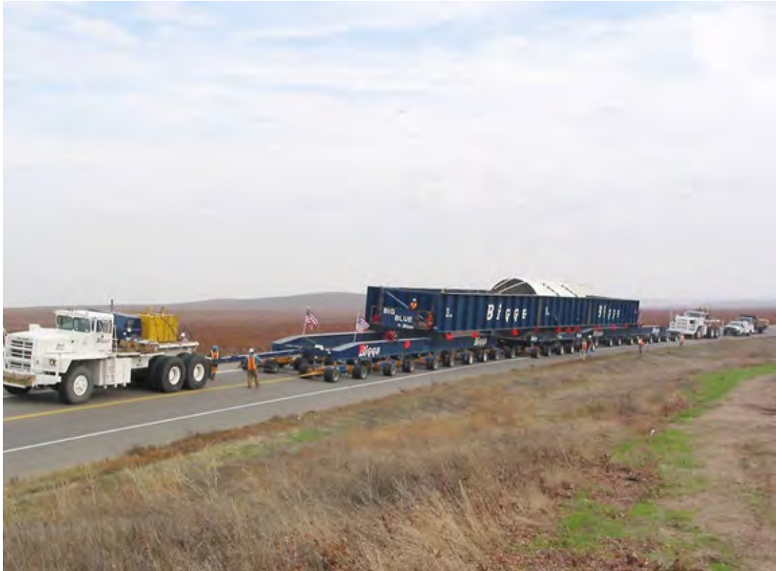
Figure 2-96. Rancho Seco Generator on Heavy Haul Truck Being Transported to the Port of Stockton, California (2002)
