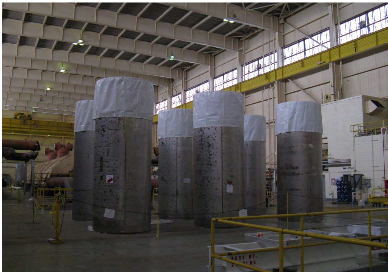
Figure 2-140. Spent Nuclear Fuel Transportable Storage Canisters Staged at Zion (2013)
