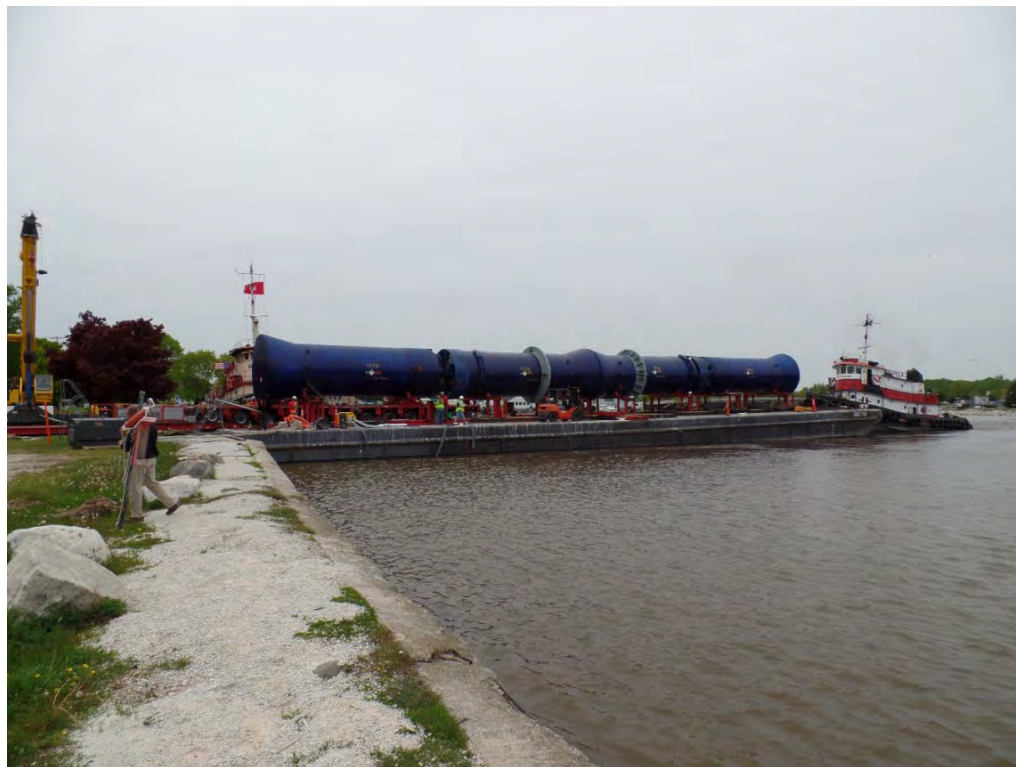
Figure 2-256. Barge with Four Steam Generators at Kewaunee Barge Transload Location (2014)
