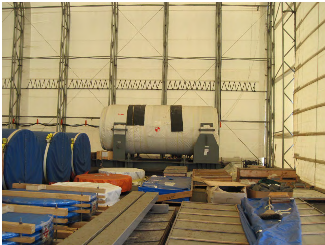
Figure 2-266. Transfer Cask for 32PTH2 Canisters (2015)
