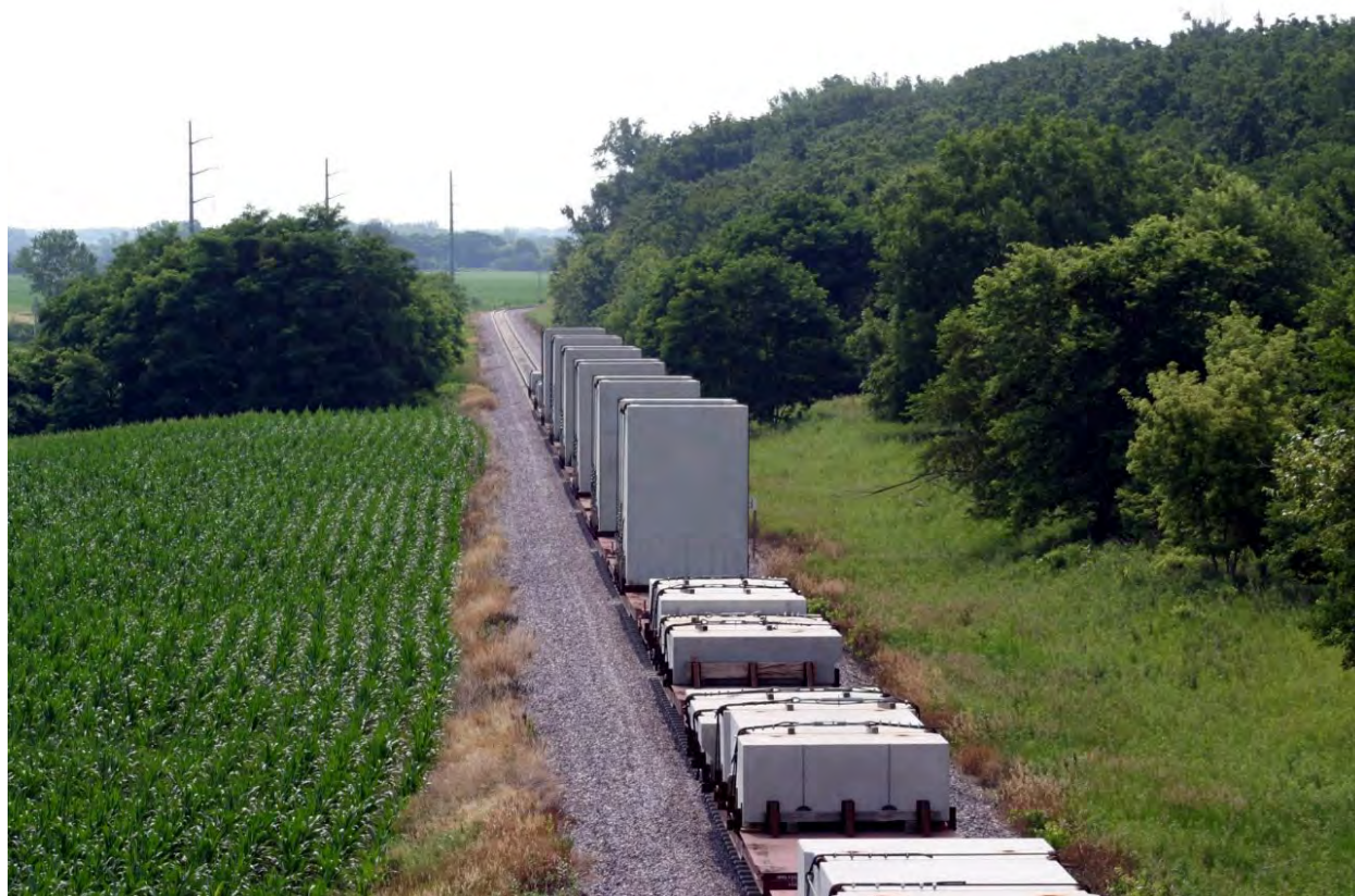
Figure 2-361. Horizontal Storage Modules Being Transported by Rail to Fort Calhoun
