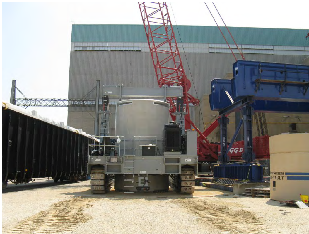
Figure 2-141. Transporter Used to Move Vertical Concrete Storage Casks (2013)
