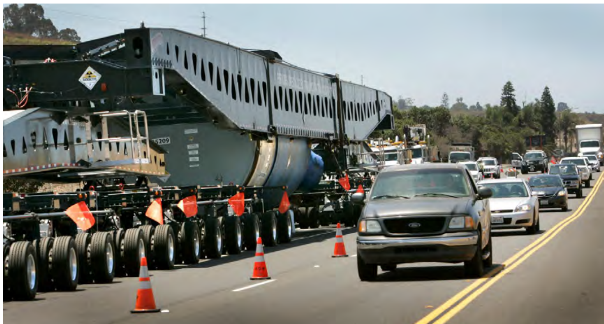
Figure 2-312. Old Steam Generator on Heavy Haul Truck Transporter (2011)
