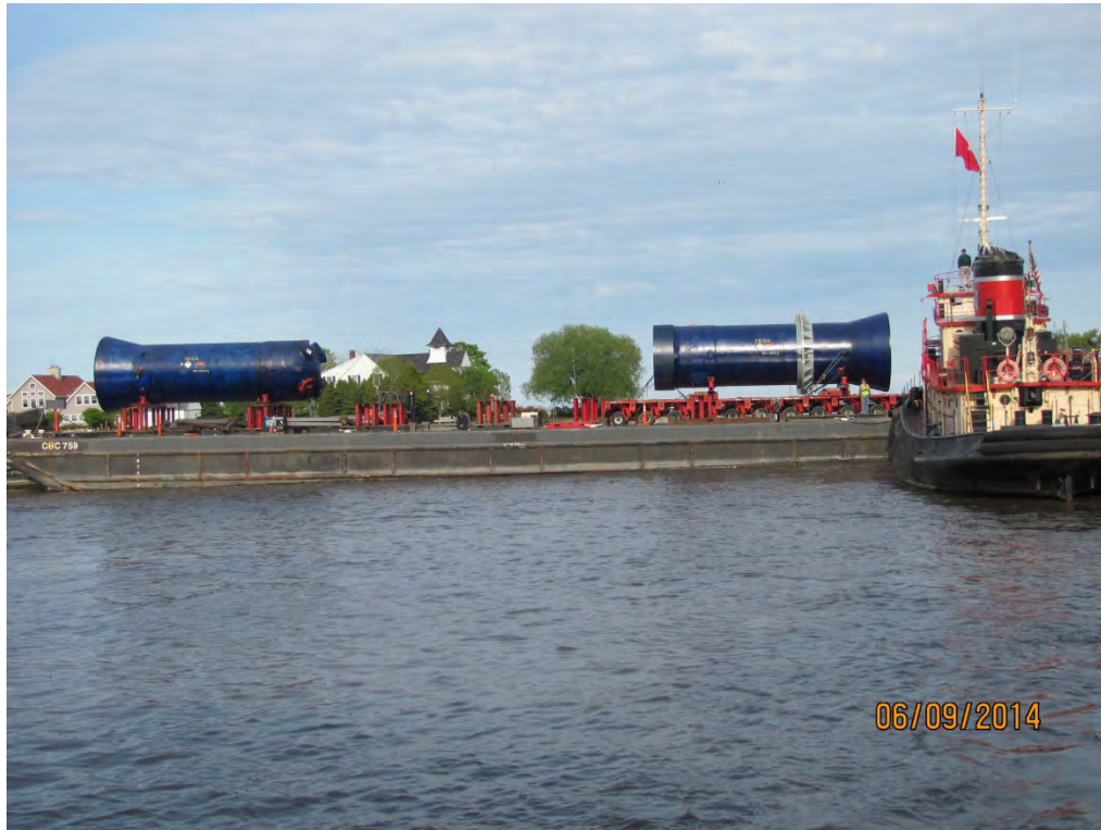
Figure 2-254. Barge with Two Steam Generators at Kewaunee Barge Transload Location (2014)
