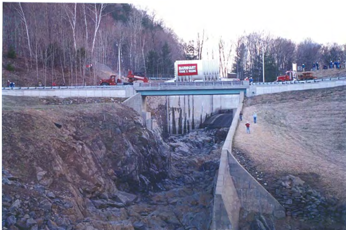
Figure 2-24. Yankee Rowe Reactor Pressure Vessel Crossing the Sherman Dam (1997)
