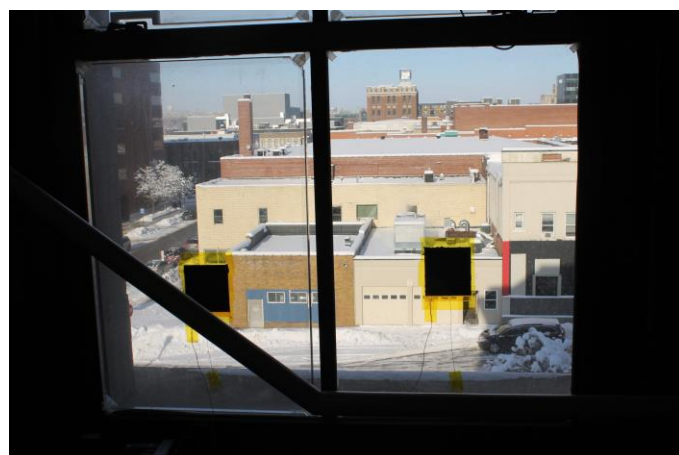
Figure 5. Window with heat flux sensors installed. The operable window sash had four glass lites. The insulation panel technology was installed on three of the four glass lites; both upper lites are outside the image frame, and the left lite is shown in this image. The insulation panel technology was not installed on the right lite so that a heat flux sensor could simultaneously measure the baseline IGU and the IGU that has the insulation panel technology installed.
