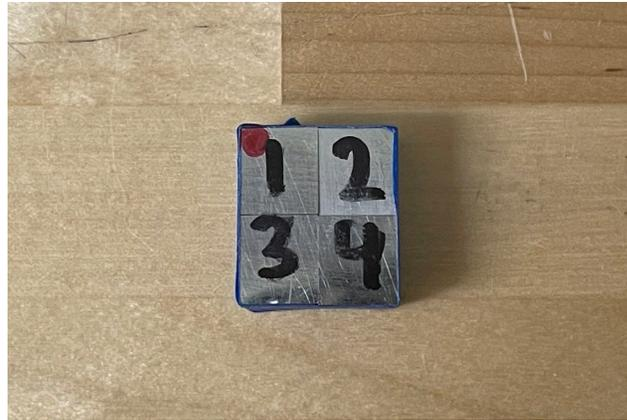
Figure 4. LPBF 316H SS cuboids after being cut using electrical discharge machining.
