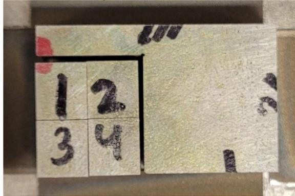
Figure 7. Wrought 316L cuboids after being cut using electrical discharge machining.
