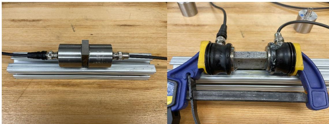
Figure 8. Through transmission configuration for longitudinal (left) and shear (right) measurements.
