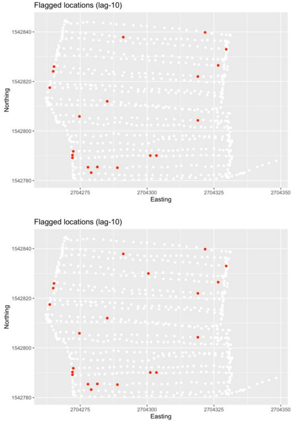
Figure 5.9. Flagged locations (red) indicate observations exceeding the critical level for the reference area 1 (top) and 2 (bottom) and lag- k ( k = 10 ) value, with easting on the x-axis and northing on the y-axis. The critical values used for each plot are listed in Table 2.
