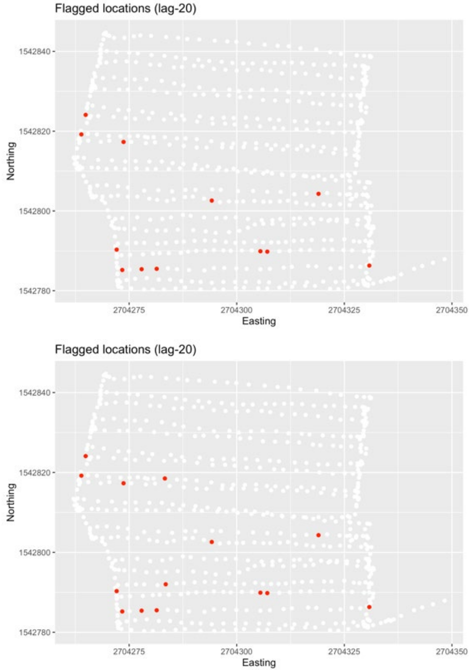
Figure 5.10. Flagged locations (red) indicate observations exceeding the critical level for the reference area 1 (top) and 2 (bottom) and lag- k ( k = 20 ) value, with easting on the x-axis and northing on the y-axis. The critical values used for each plot are listed in Table 2.
