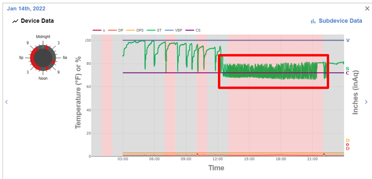
Figure 4-10. Supply-air Temperature is Deviating Significantly from Set Point
