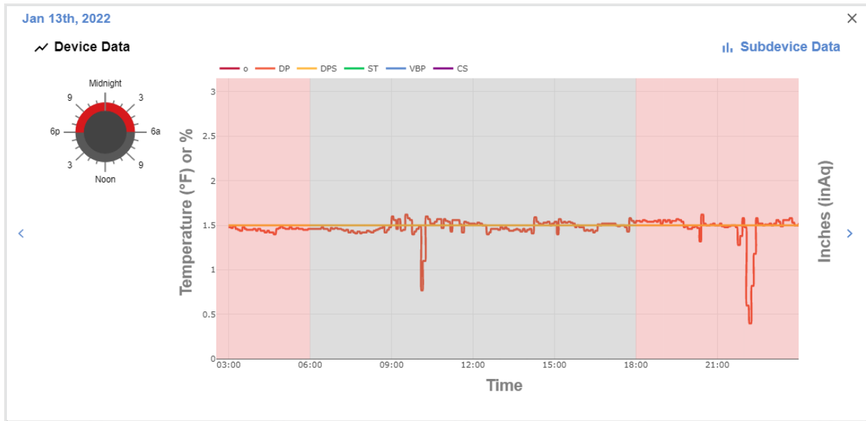
Figure 4-1. ERU-B1-NWING Operating Continuously During Unoccupied Hours
