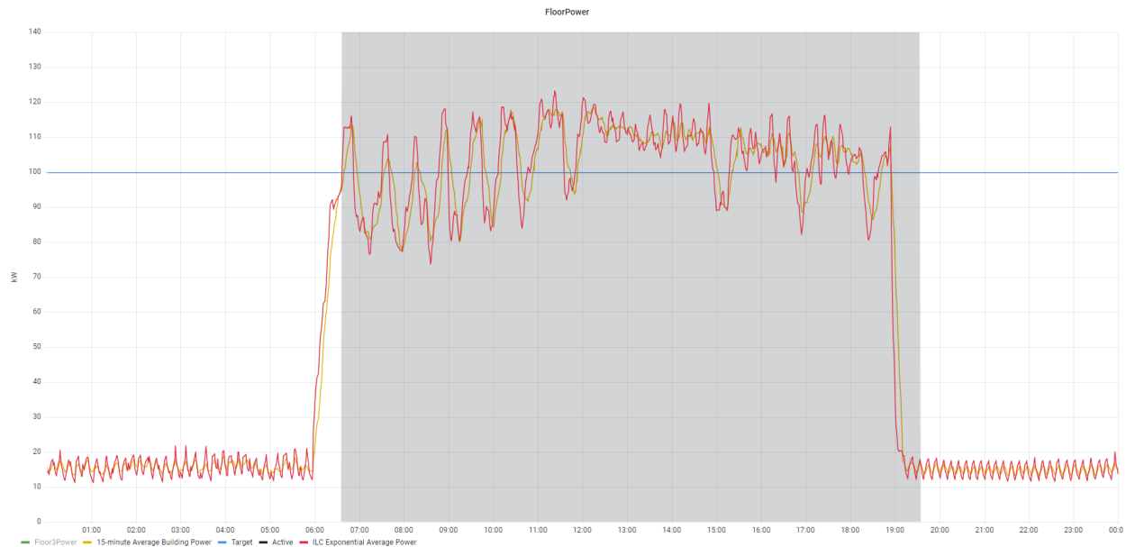
Figure 7-15: OJS Floor-3 Demand and ILC Target September 19 th , 2022
