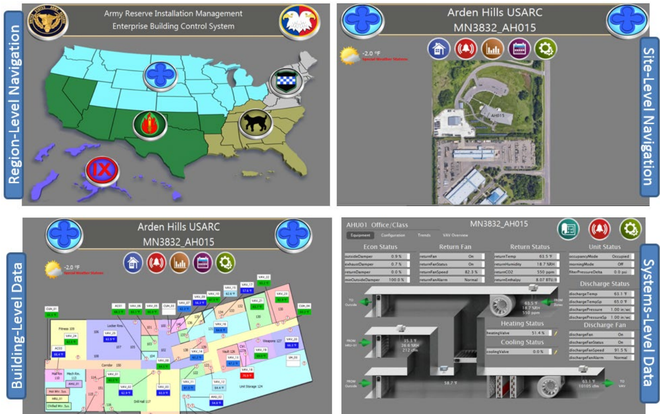
Figure 3. Enterprise Building Control System Interface
