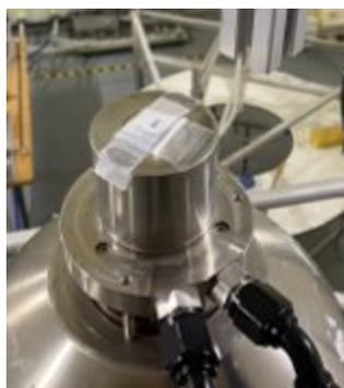
Figure 2-5. Image of In metal foil stack on the D-T Generator.
