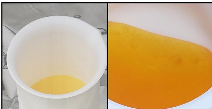
Figure 2-3, Irradiated indium oxide sample dissolving in aqua regia. The left image shows the actively dissolving sample, the right image shows the final aqua regia solution.
