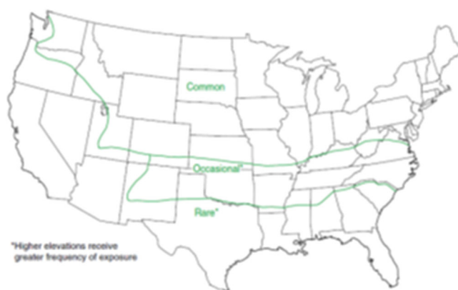
Figure 8 – Map showing the prevalence of freeze-thaw exposure on cement and concrete systems.
