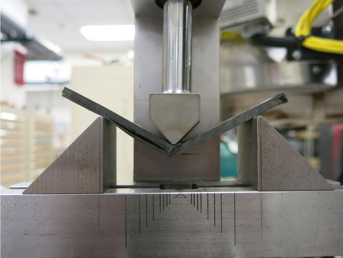
Figure 5. Preliminary Testing in 3-Point Bend Test Fixture without Slack Adapter to Maintain Constant Velocity
