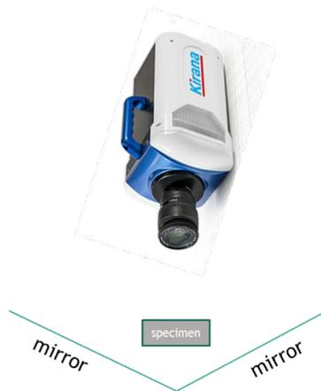
Figure 10. Illustration of a pair of mirrors applied to the tensile specimen for simultaneously tracking cracks at top and side surfaces.
