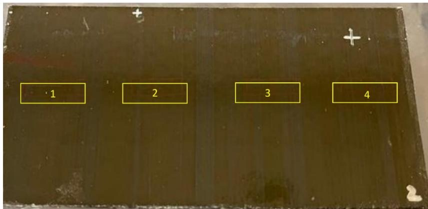
Figure 28: Picture showing where cross-sections were taken on half of panel 2 from set #2
