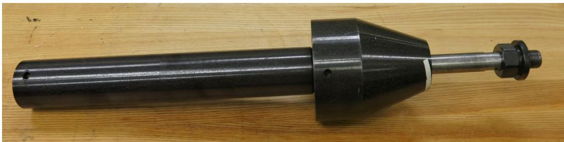
Figure 4. Slack Adapter Utilized to Allow Test Machine to Reach Targeted Speed before Engaging Specimen
