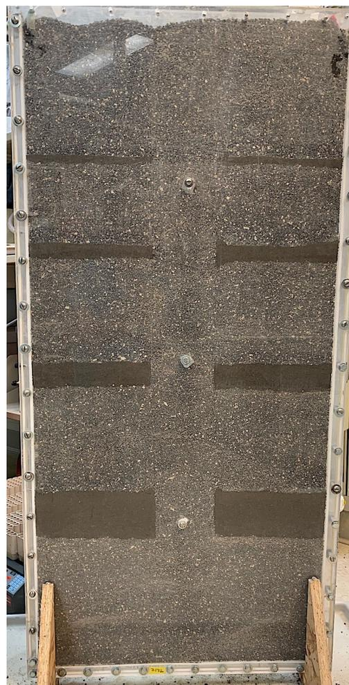
Figure 2.2. Infiltration column with low-conductivity rectangular inclusions. Artificial groundwater was dripped in the upper left and artificial groundwater with a surfactant was dripped into the sediment in the upper right.
