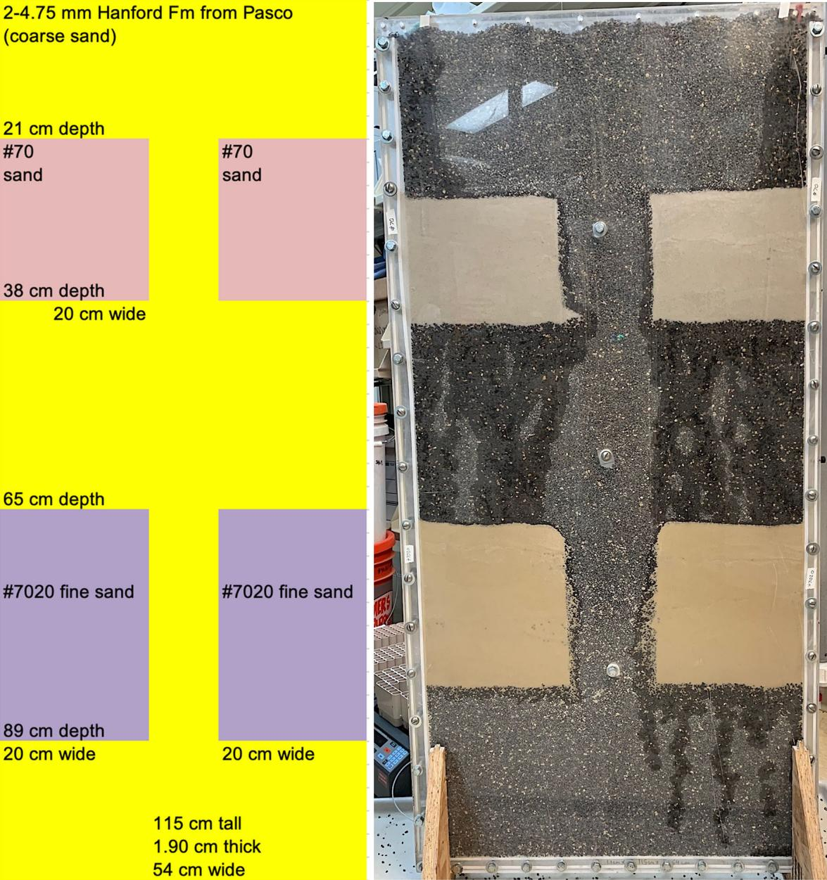
Figure E.2. 2-D infiltration experiment K2 with infiltration of artificial groundwater (left) and artificial groundwater with 400 mg/L surfactant (right) with fine sand low-K zones.
