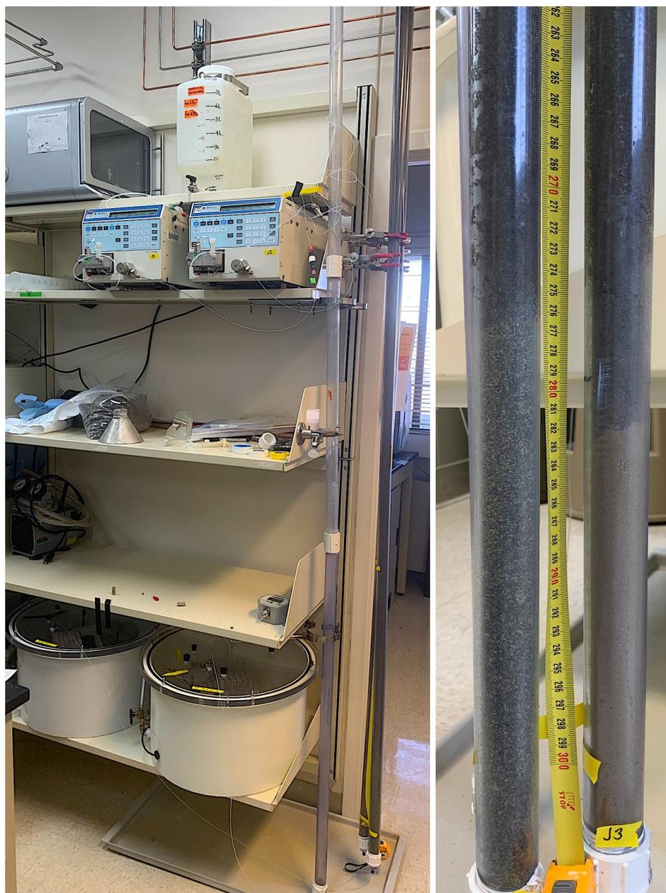
Figure 2.1. 10-ft high 1-D infiltration columns with effluent at bottom leading into fraction collectors located in vacuum chambers (left), and enlargement of the bottom of the column showing infiltration front (right).
