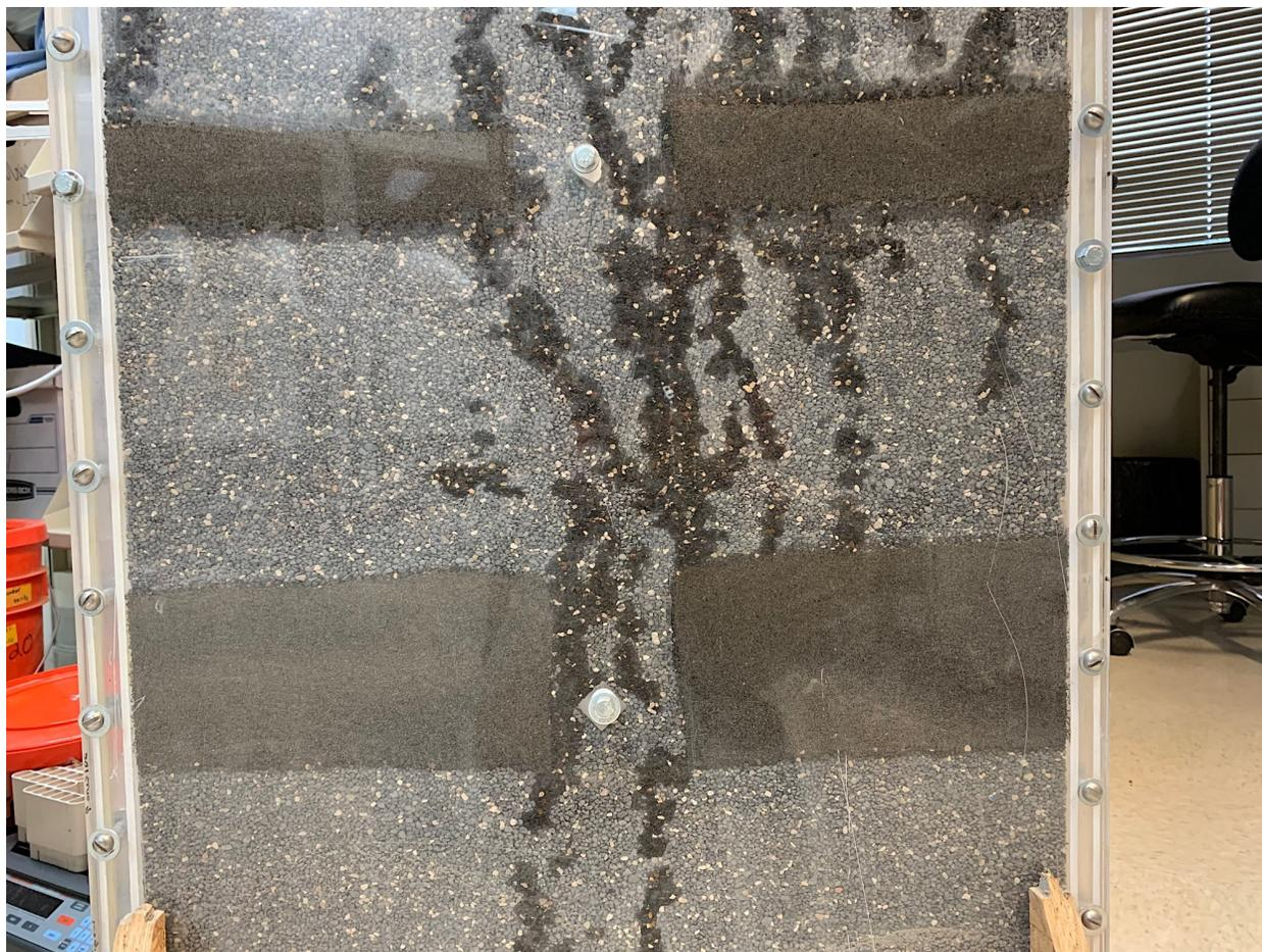
Figure E.5. Early time image of 2-D infiltration experiment K4 illustrating groundwater is flowing around the low-K zone (upper left) whereas the surfactant solution is flowing through the low-K zone (upper right).
