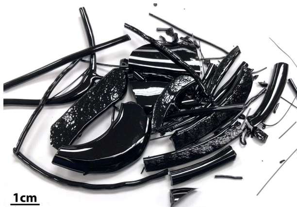
Figure 16. Picture of quenched glass after the vitrification process was completed for the CsCl sample (Run-2).
