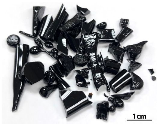
Figure 13. Picture of quenched glass after the vitrification process was completed for the KCl sample (Run-1).
