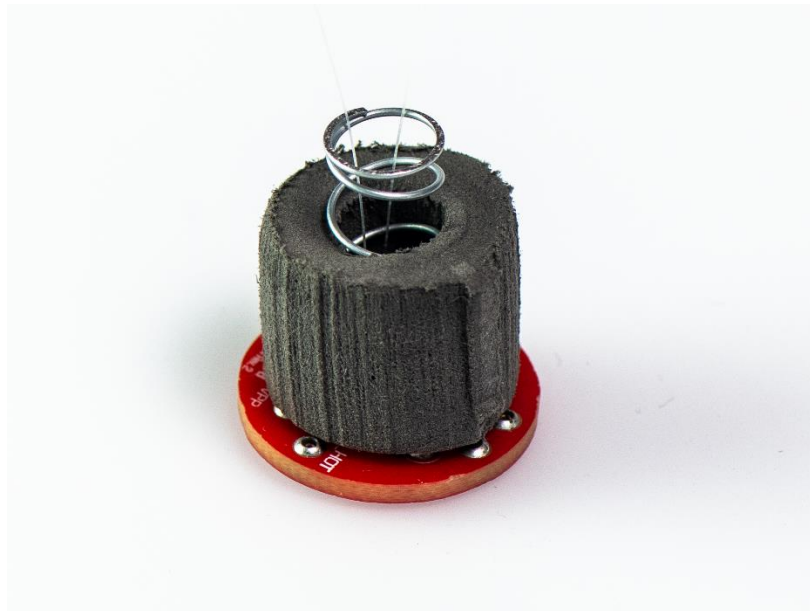
Figure A.10. Spring inserted in foam ring.
