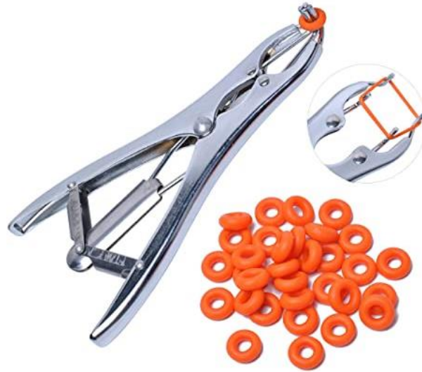
Figure A.16. An example of castration pliers used to open the end of the balloons to insert the silicone stoppers.
