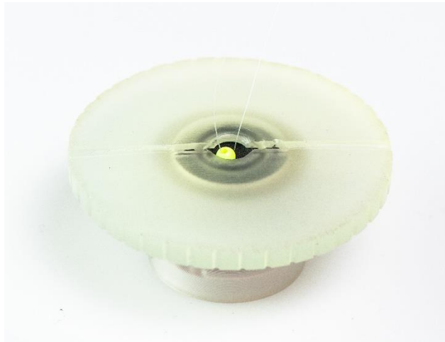
Figure A.13. Weight properly positioned in the weight cavity on the bottom side of the weight-tying tool.
