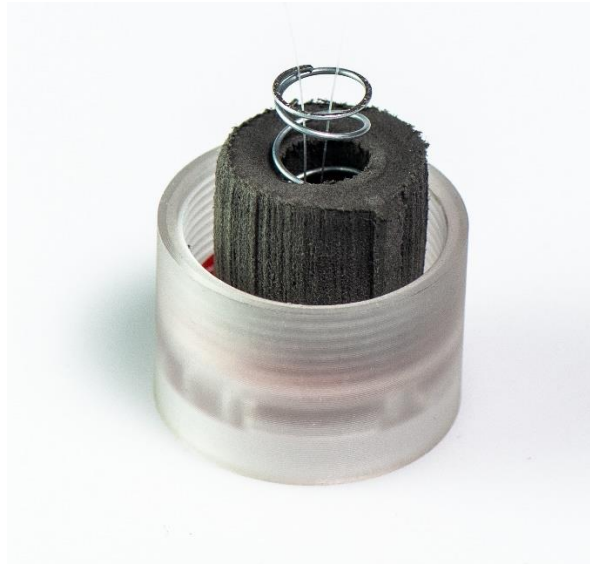
Figure A.11. The loose ends of the fishing line, installed in the recovery board, threaded through the spring that is installed in the foam ring.
