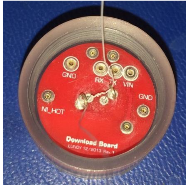
Figure A.9. Fishing line attached to the SF recovery board.
