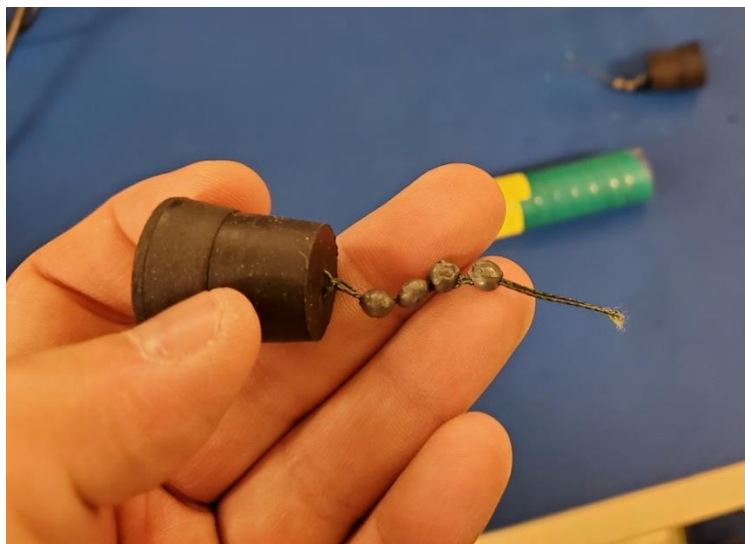
Figure A.3. Split shot fishing weights attached to fishing line to make the dummy Sensor Fish neutrally buoyant.
