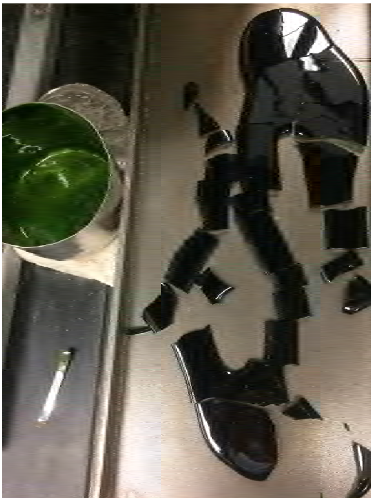
Figure 3.4. LIC-04_mod1 quenched glass after third melt at 1500 °C for 1 hour.
