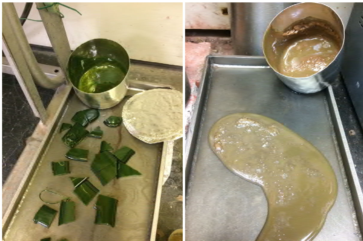
Figure 3.5. LIC-09 first melt at 1150 °C (left) and fourth/final melt at 1500 °C (right).
