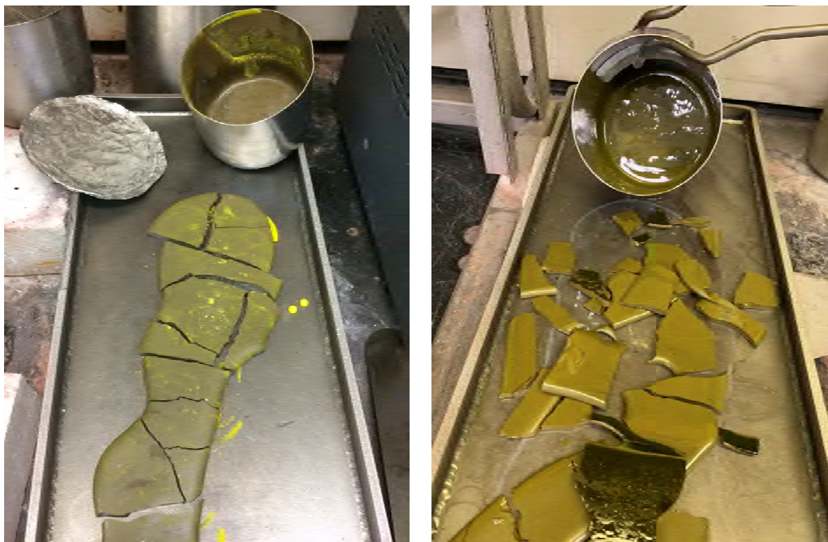
Figure 3.1. Images of LIC-02 after the first melt at 1200 °C (left) and the fourth and final melt at 1500 °C (right).
