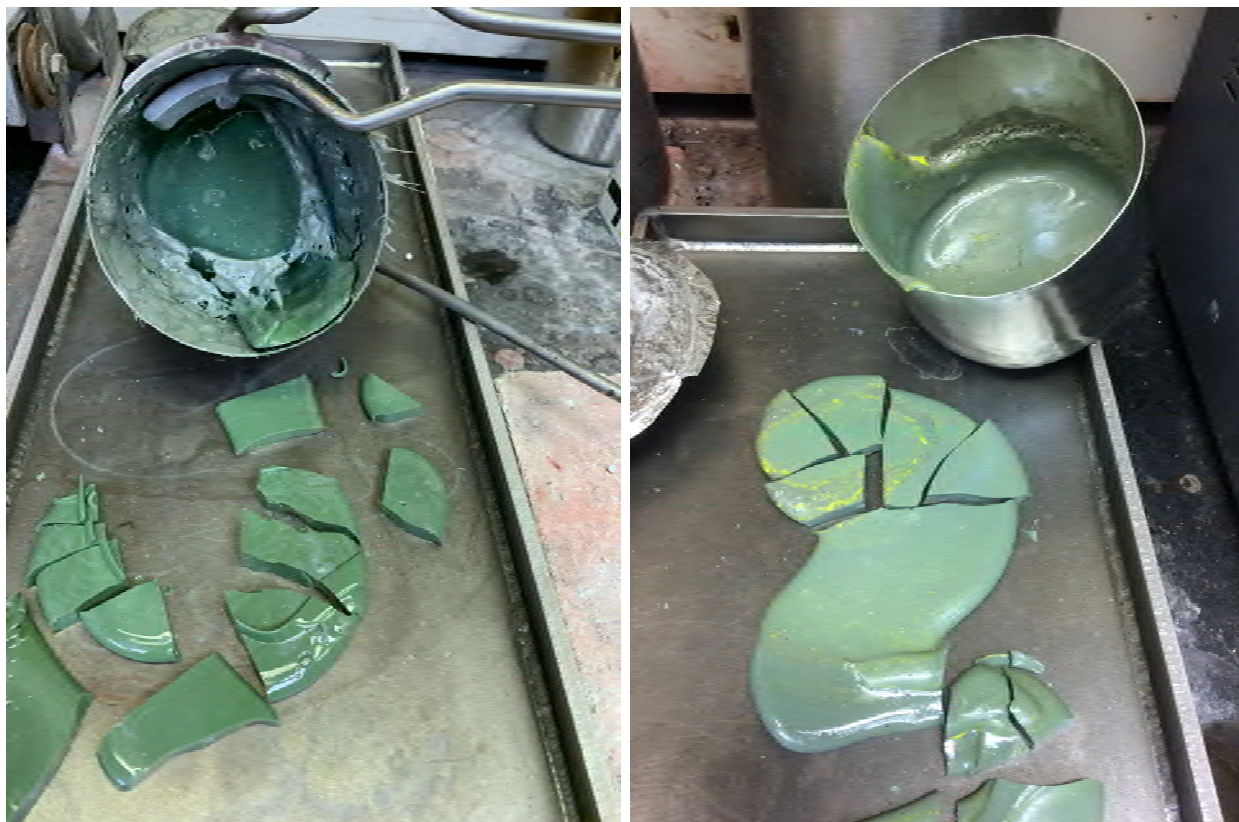
Figure 3.3. LIC-04 after the first melt at 1150 °C (left) and the fourth melt at 1350 °C (right).
