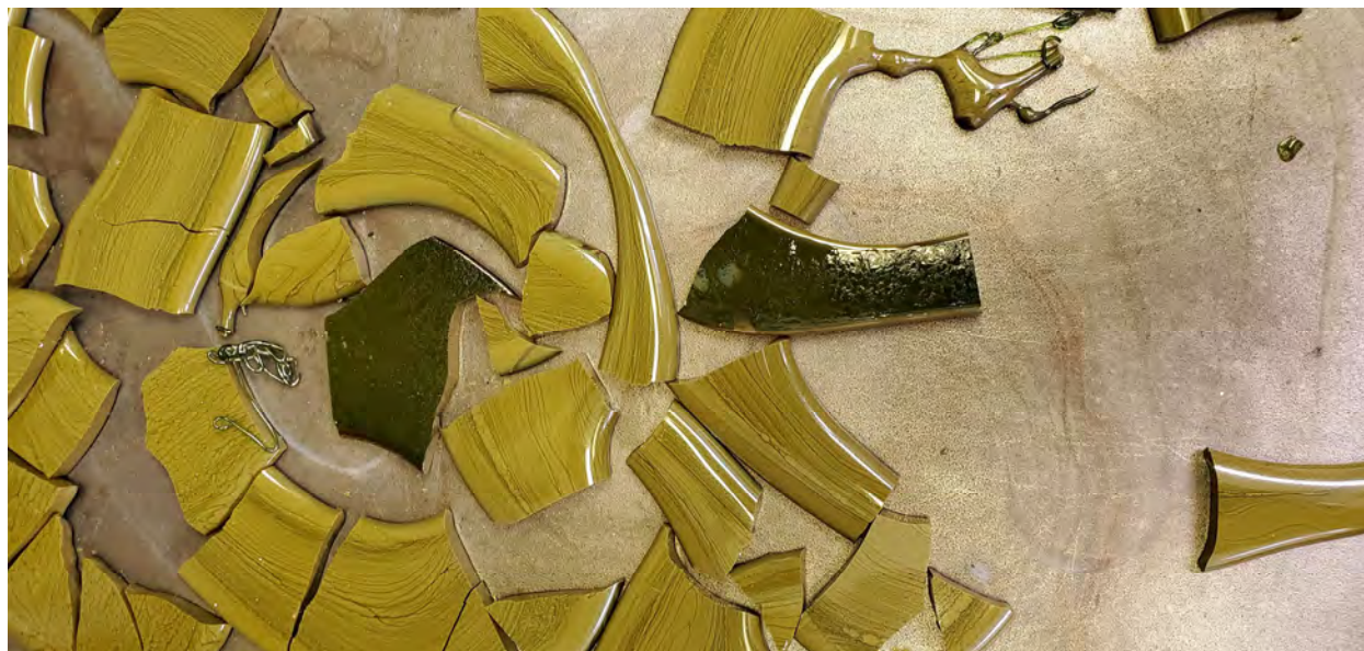
Figure 3.2. LIC-02_mod2 quenched glass after third melt at 1500 °C for 1 hour.
