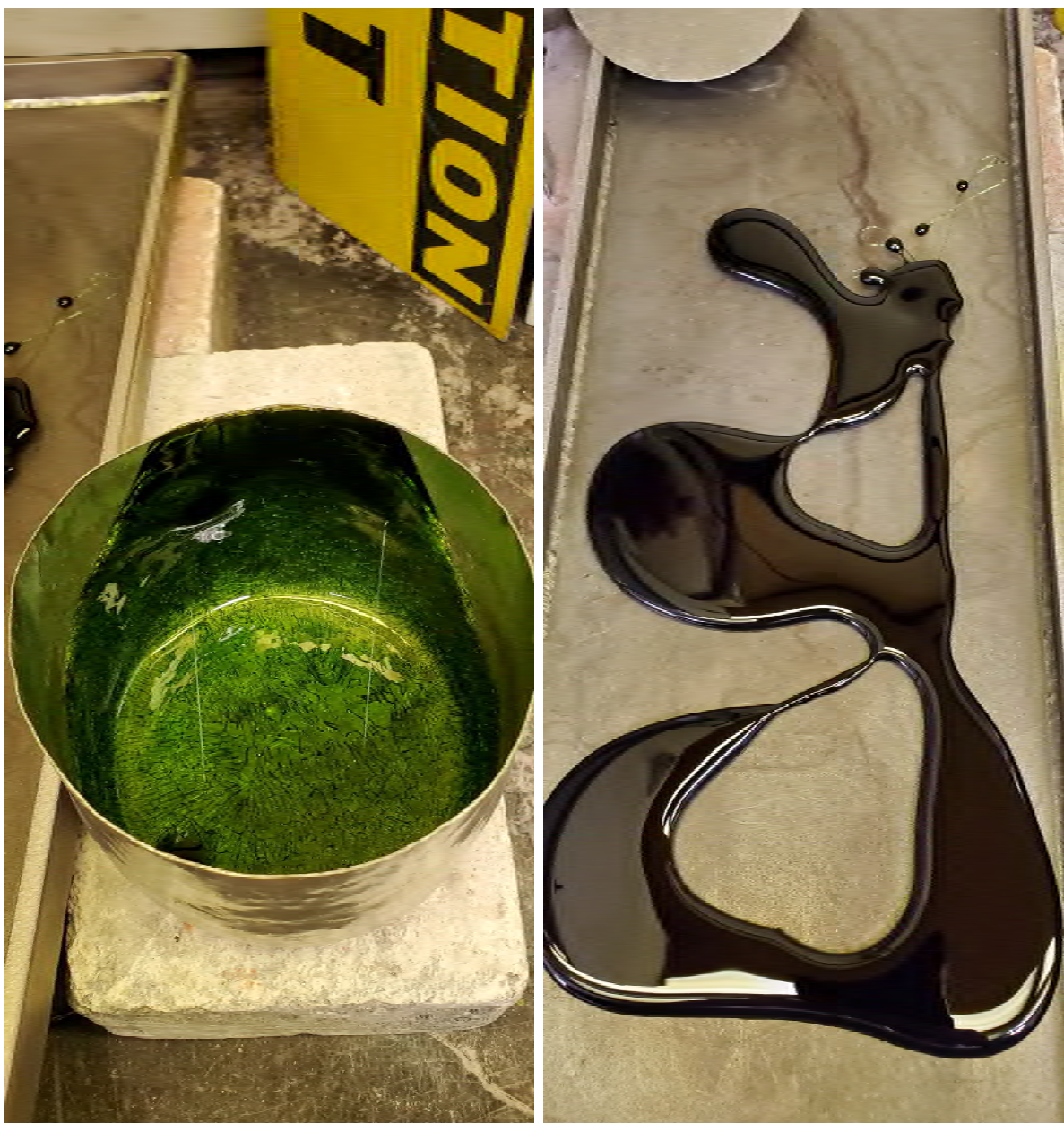
Figure 3.6. LIC-09_mod3 final melt crucible (left) and quenched glass (right) after pouring from 1450 °C.
