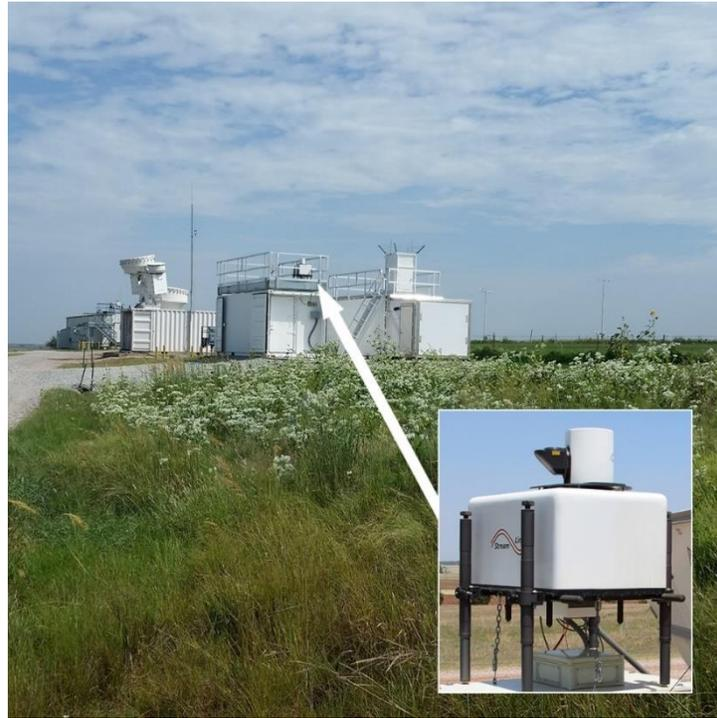
Figure 4. ARM Doppler lidar (inset) installed at the SGP central facility. (Image courtesy of the U.S. Department of Energy ARM user facility.)
