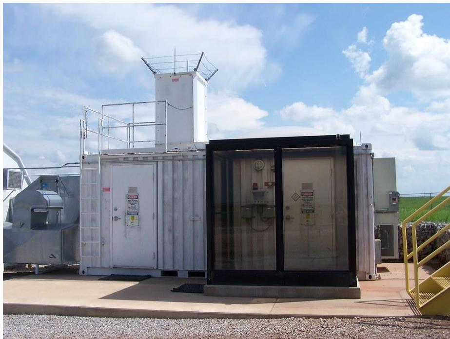
Figure 6. Raman lidar installed on top of a shipping container at the SGP central facility in 2007. (Image courtesy of the U.S. Department of Energy ARM user facility.)
