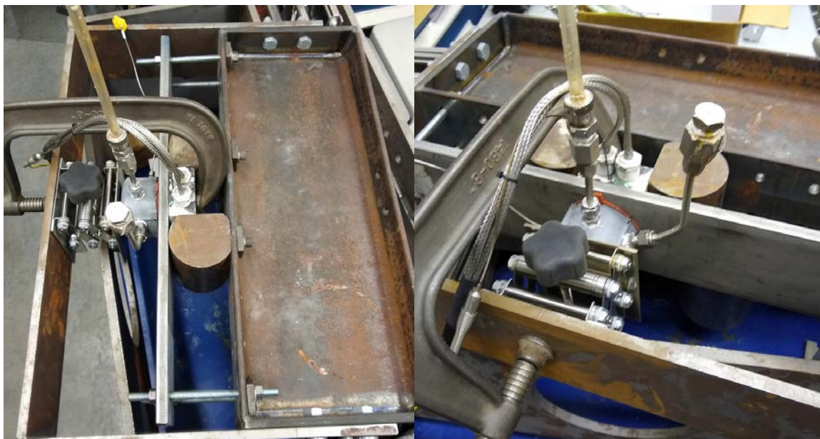
Figure 9. Specimen in chloride crack generation fixture showing the full setup.
