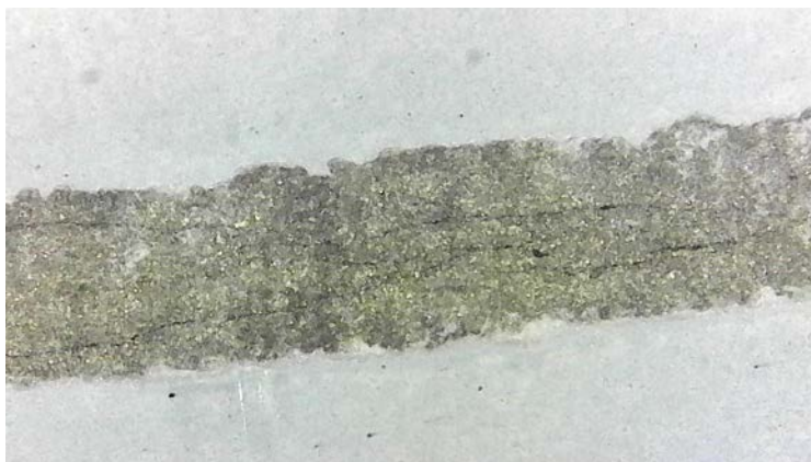
Figure 11. Micrograph of crack cross-section perpendicular to crack.
