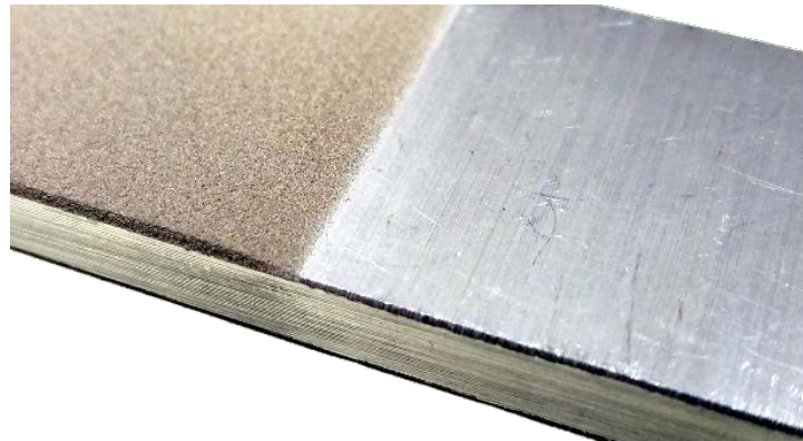
Figure 4. High-pressure cold spray coating of commercially pure nickel sprayed (left side) at PNNL.
