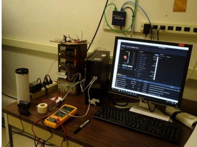
Figure 11. The PCB, DC motor testing station within the HEGF Control Room, containing the computer, power supplies, and PCB:DC motor control set.
