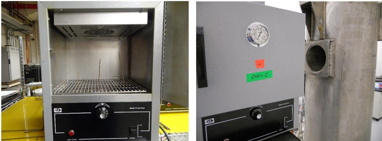
Figure 3. Left-Mini oven of ~0.6 ft.3 volume for testing temperatures from 72-200°F (22-93C), Right-mini oven placed in the gamma-ray field (30° port shown) of the HEGF Exposure Room for combined radiation-temperature tolerance testing.
