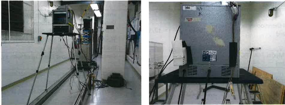
**Figure 2:** Shows dose rate measurement locations – in mini-oven at 415 cm source distance, attached to surface of oven, and at end of meterstick at 260 cm source distance.
