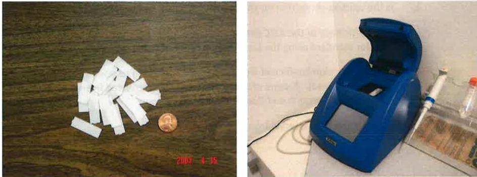
**Figure 3:** The Sunna LiF film dosimeters (Left), and the Turner Trilogy Fluorimeter used to read out the dosimeters (Right).
