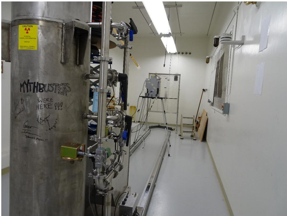
Figure 5. HEGF Exposure Room during setup prior to the start of irradiation. Foreground: gamma-ray irradiator; Background: mini oven on a pedestal positioned along the beam path.
