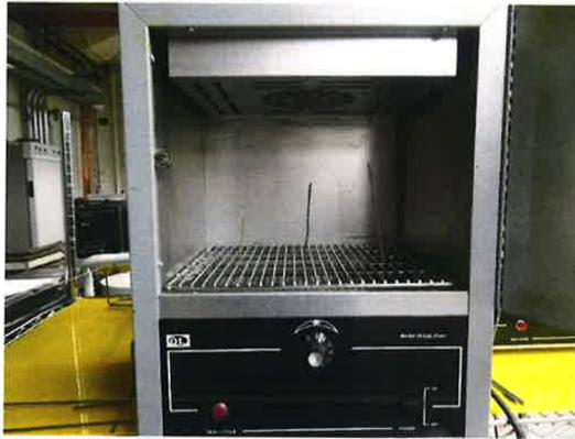
**Figure 5.** The interior of the Quincy Labs Model 10 mini-oven, showing the three thermocouples utilized for tight temperature control and monitoring. The center thermocouple is used to control the oven temperature within about 1 °C, and the left and right thermocouples are used to monitor the oven temperature at lower and upper positions.
