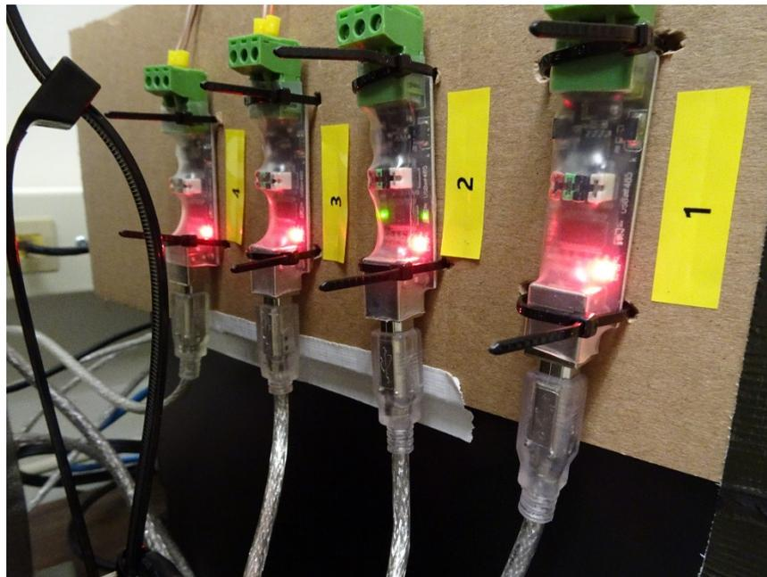
Figure 14. The communications interfaces between the computer in the HEGF Control Room and the PCB: DC motor pairs in the HEGF Exposure Room.
