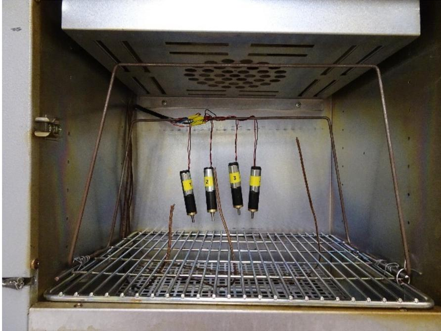
Figure 17. The four powered lone DC motors within the mini oven just prior to the start of irradiation at the 2 krad/hr dose rate.
