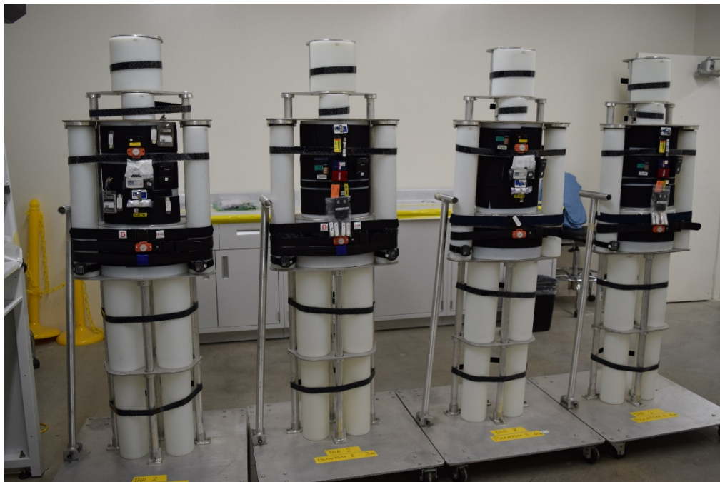
Pulse 2 Example of PNADs on Phantoms.
