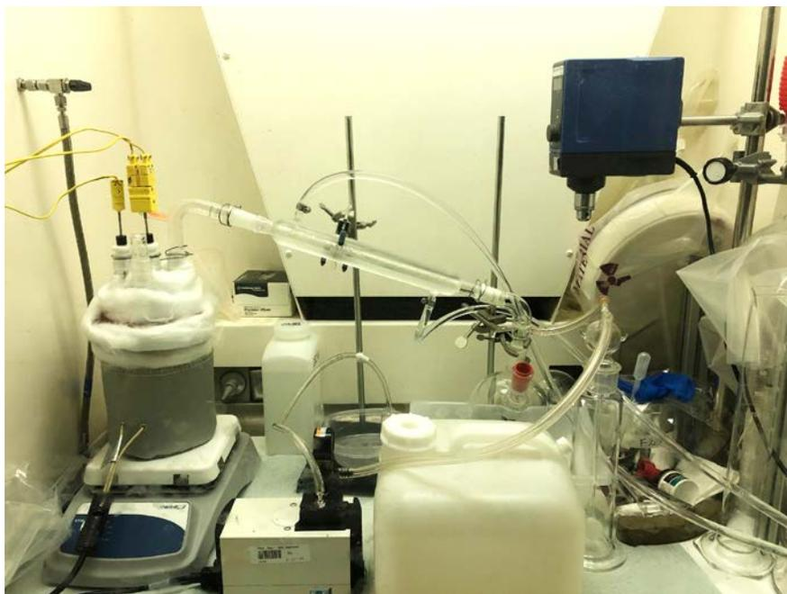
Figure 4.2. EMF evaporator test apparatus as arranged in a CA fume hood.
