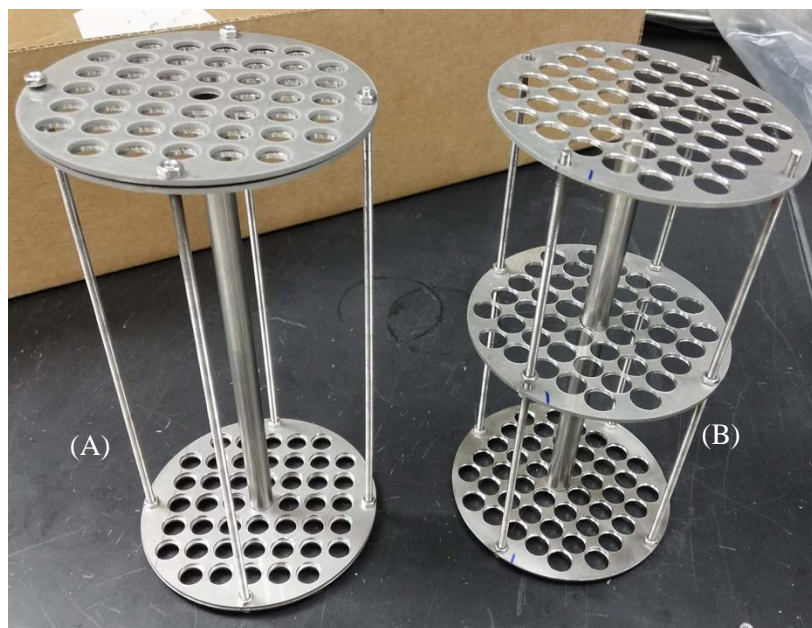
Figure 9. Photograph of Actual Cladding Tube Holders for Test D. The holder for PWR clad tubes is on the left (A) and BWR clad tubes is on the right (B).
