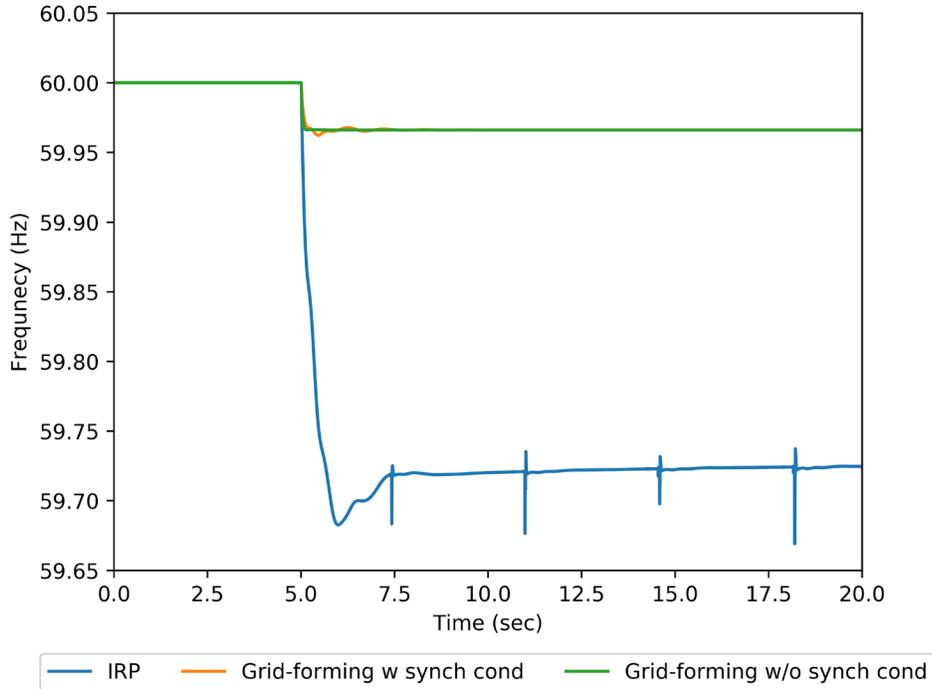
Figure 5-21: Frequency response of the system for the three Solar scenarios.
