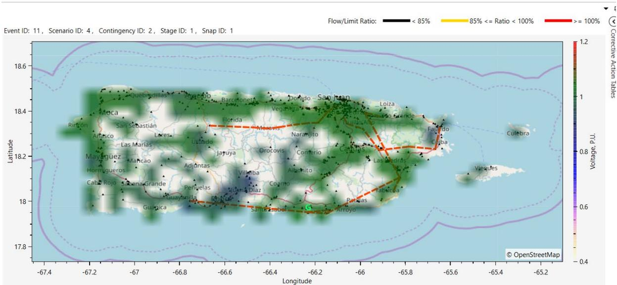
Figure 5-14: Voltage profile plotting for Contingency 1 in Hurricane Maria simulation with 2028 day peak case, additional protection models and inverter models (corrective actions applied to 100 kV & Above systems) – figure generated by DCAT Analytics
