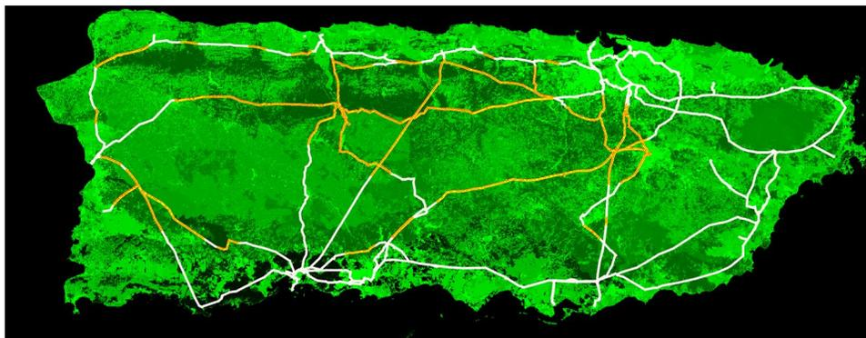
Figure 4-4: Vegetation impacted assets (in yellow) identified by overlaying electric grid GIS on 2001 USGS land cover shape file<sup>1</sup>
