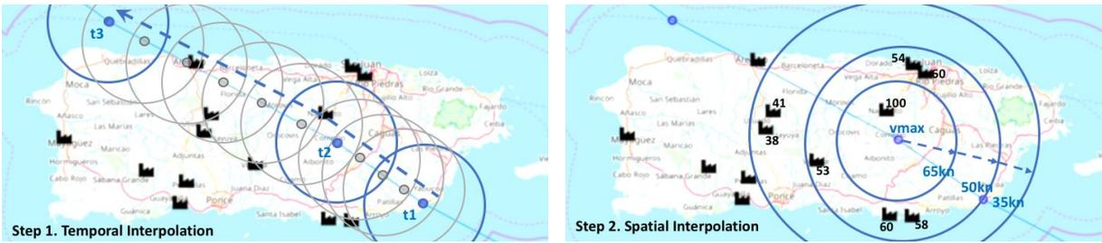
Figure 2-8: Graphic depicting the methodology of the Temporal Sequence Model, showing the interpolation over timestamps in step 1 and the spatial interpolation between wind field edges in step 2
