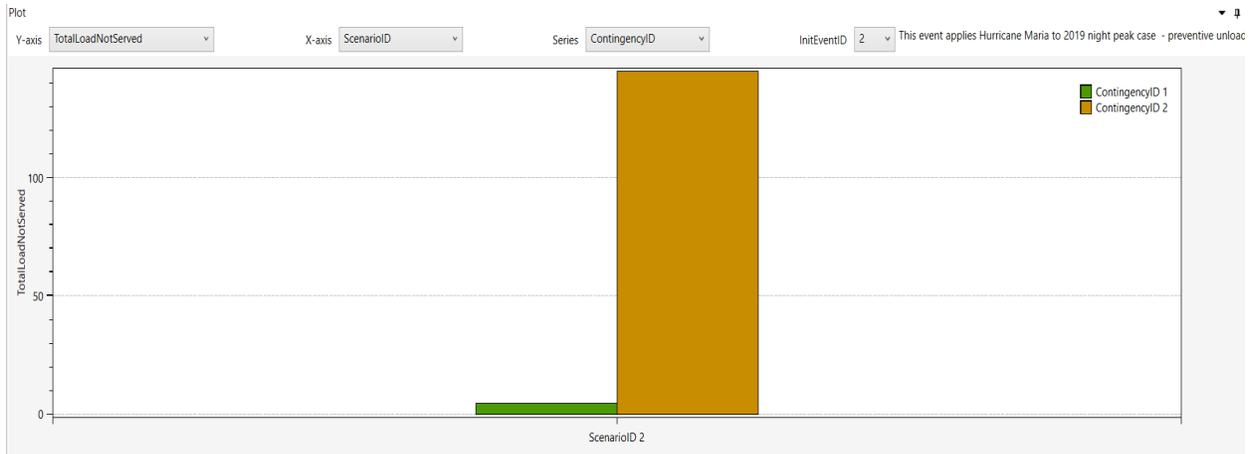
Figure 5-10: Total load not served in Hurricane Maria simulation with 2019 night peak preventive unloading case (corrective actions applied to 100 kV & Above systems) – figure generated by DCAT Analytics
