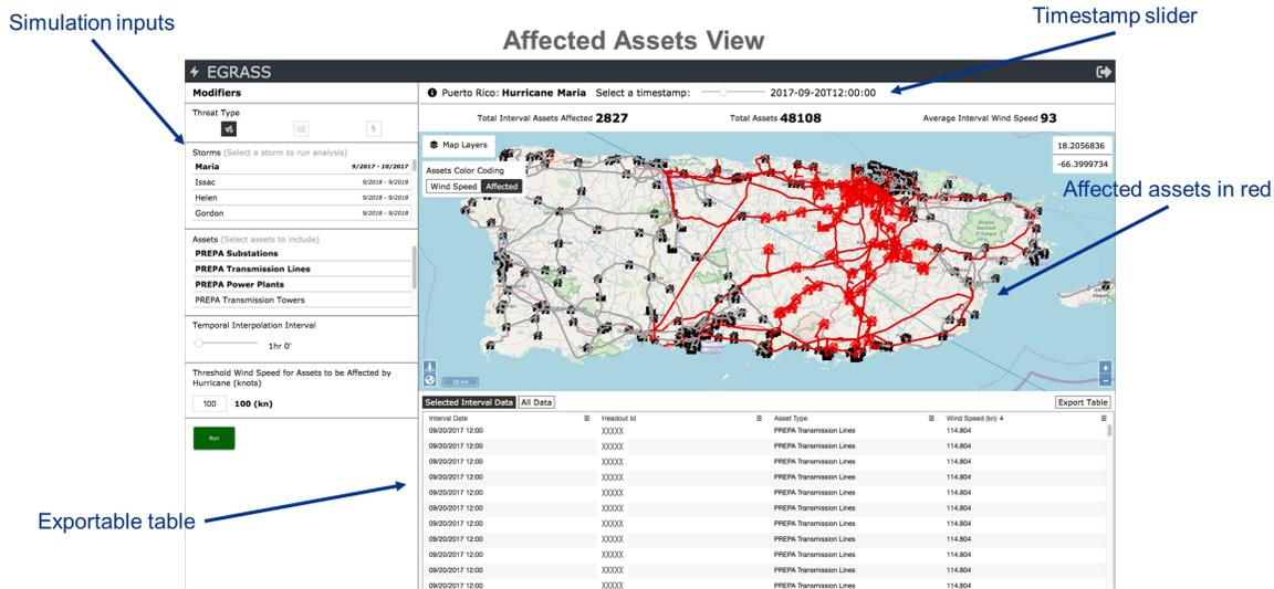
Figure 2-9: The temporal sequencing model user interface with the affected assets view
