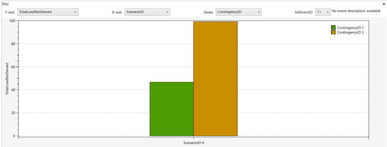
Figure 5-13: Total load not served in Hurricane Maria simulation with 2028 day peak case, additional protection models and inverter models (corrective actions applied to 100 kV & Above systems) – figure generated by DCAT Analytics
