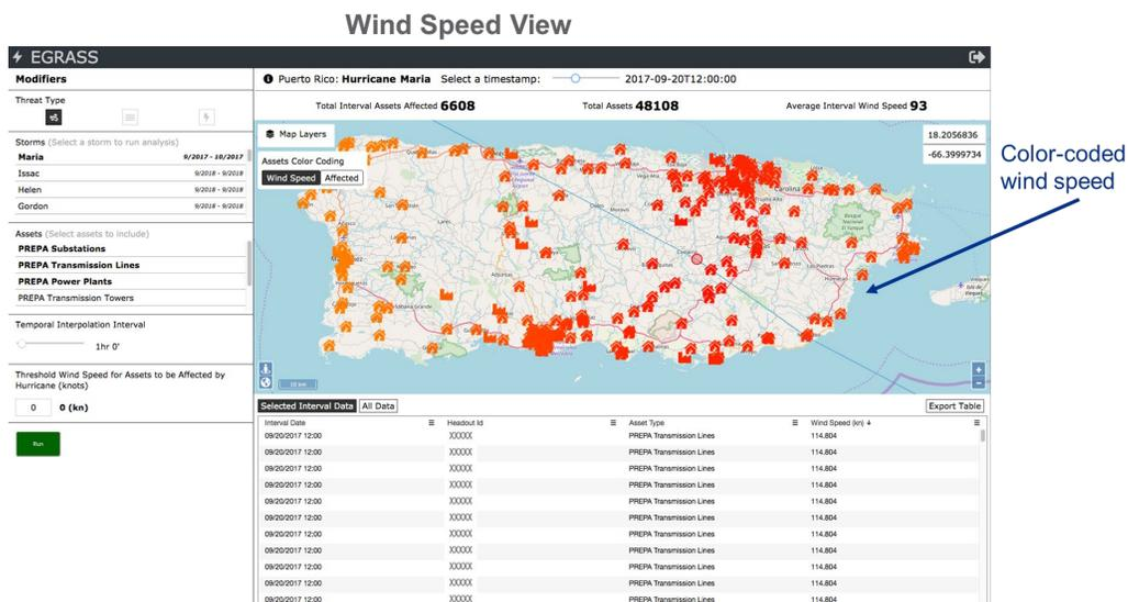
Figure 2-10: The temporal sequencing model user interface with the wind speed view
