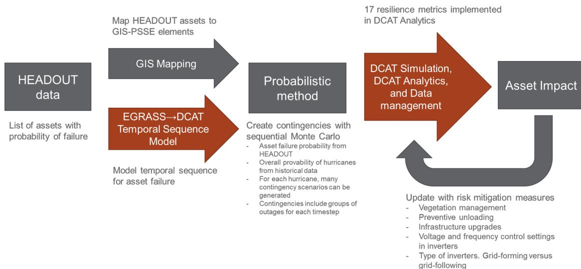
Figure 1-1: Risk-Based Dynamic Contingency Analysis Framework and Interaction of HEADOUT, EGRASS and DCAT tools
