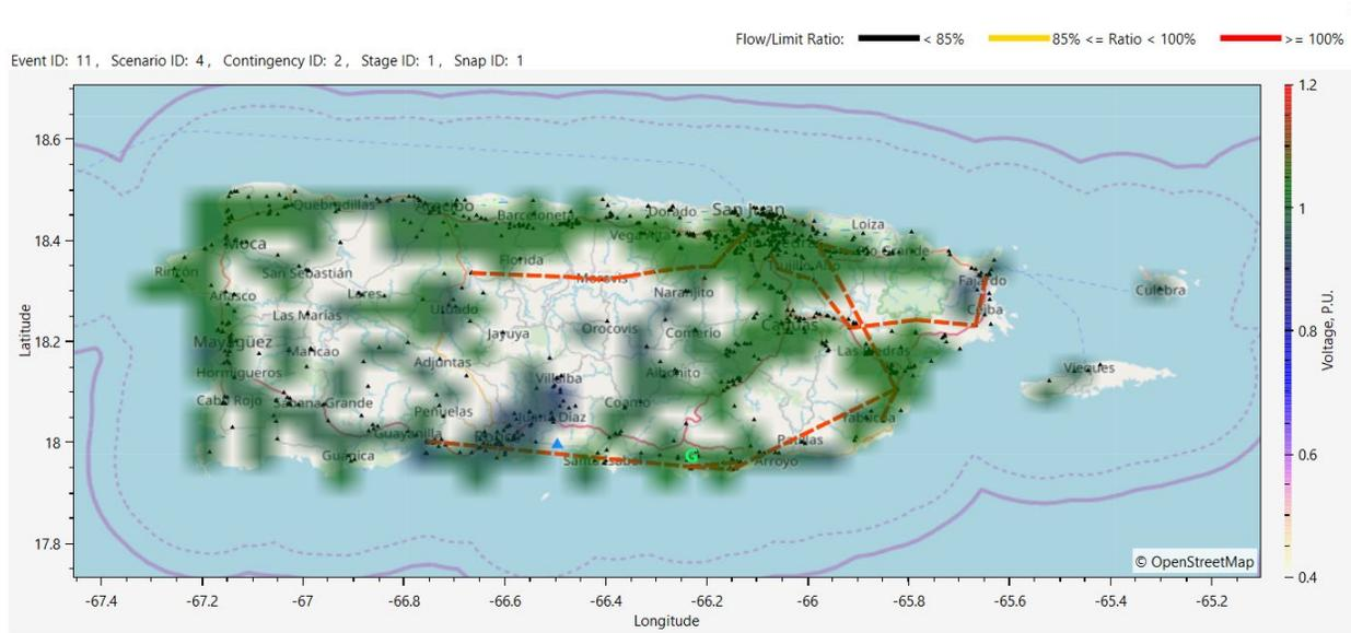
Figure 5-15: Voltage profile plotting for Contingency 2 in Hurricane Maria simulation with 2028 day peak case, additional protection models and inverter models (corrective actions applied to 100 kV & Above systems) – figure generated by DCAT Analytics
