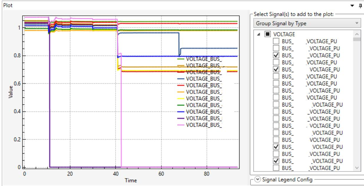
Figure 5-9: Dynamic evolution of voltages in p.u. for Contingency 2 in Hurricane Maria simulation with 2019 night peak case (corrective actions applied to 100 kV & Above systems) – figure generated by DCAT Analytics
