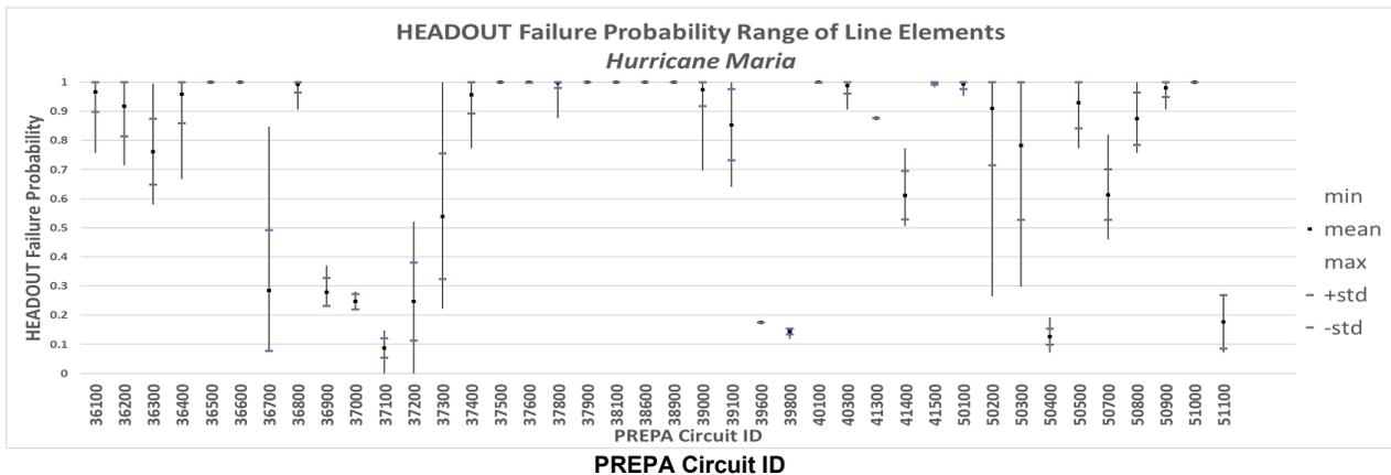
Figure 4-5: Range of HEADOUT failure probabilities associated with each 230kV and 115kV PREPA Circuit ID for Hurricane Maria
