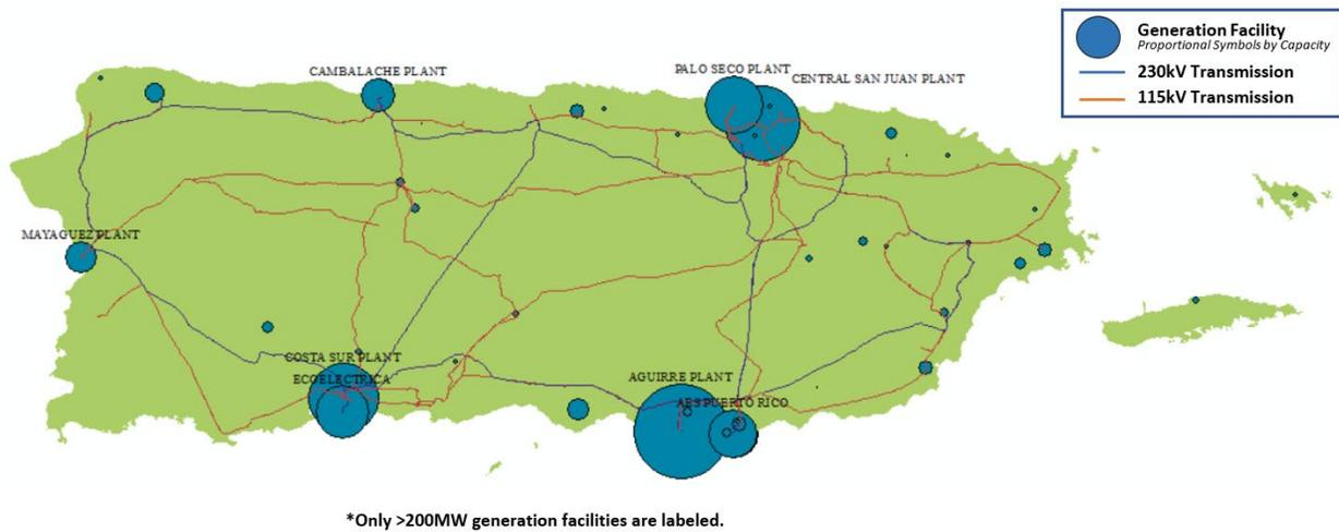
Figure 4-1: Transmission and generation facilities in Puerto Rico (figure based on publicly available GIS information<sup>1</sup>).
