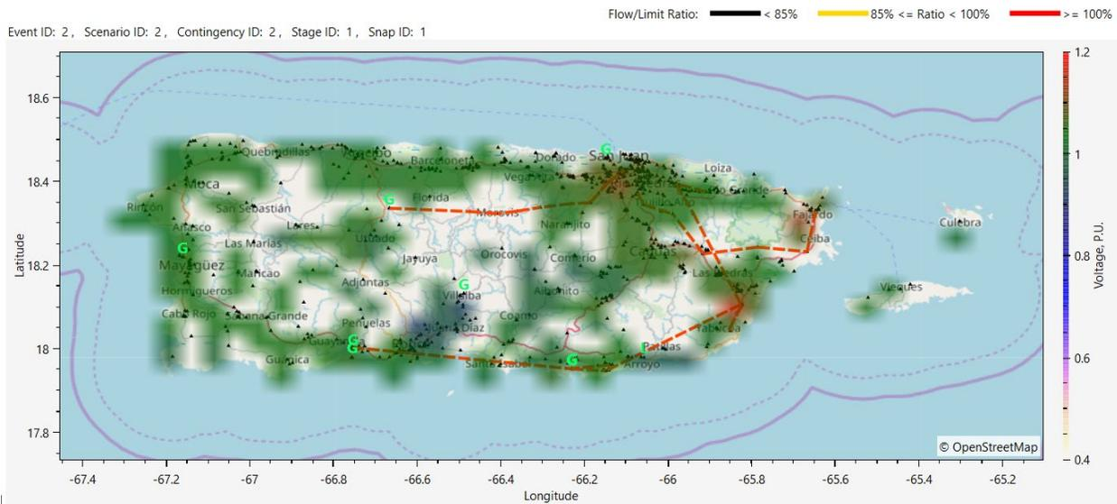
Figure 5-12: Voltage profile plotting for Contingency 2 in Hurricane Maria simulation with 2019 night peak preventive unloading case (corrective actions applied to 100 kV & Above systems) – figure generated by DCAT Analytics
