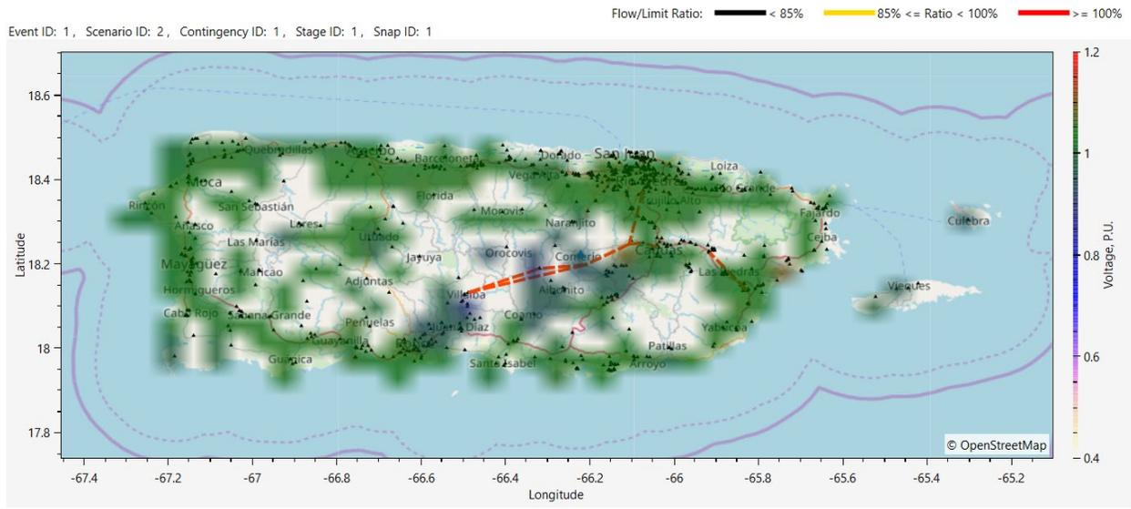
Figure 5-7: Voltage profile plotting for Contingency 1 in Hurricane Maria simulation with 2019 night peak case (corrective actions applied to 100 kV & Above systems) – figure generated by DCAT Analytics
