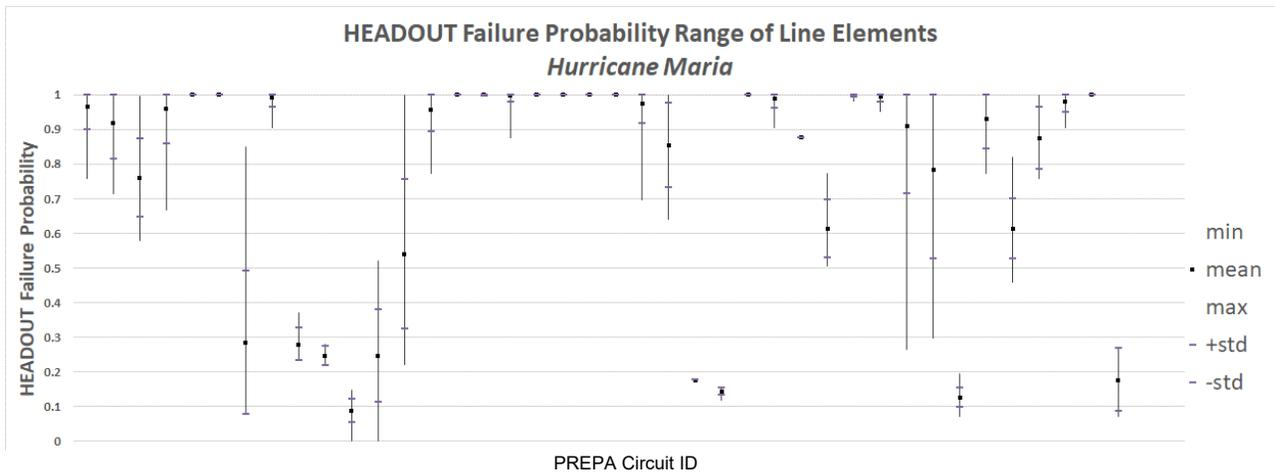
Figure A-1 HEADOUT failure probability range of line elements for Hurricane Maria.
