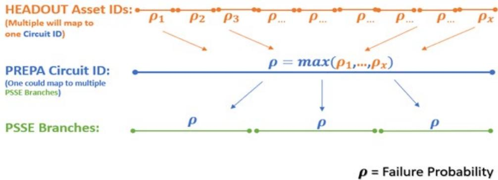
Figure 2-5: HEADOUT transmission line and transmission tower asset failure probability mapping to PSS®E branches
