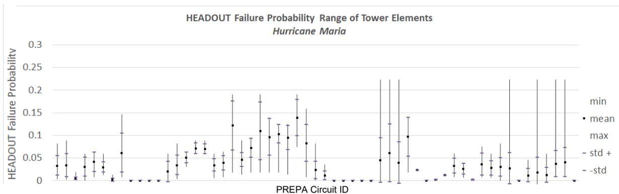
Figure A-2 HEADOUT failure probability range of tower elements for Hurricane Maria.
