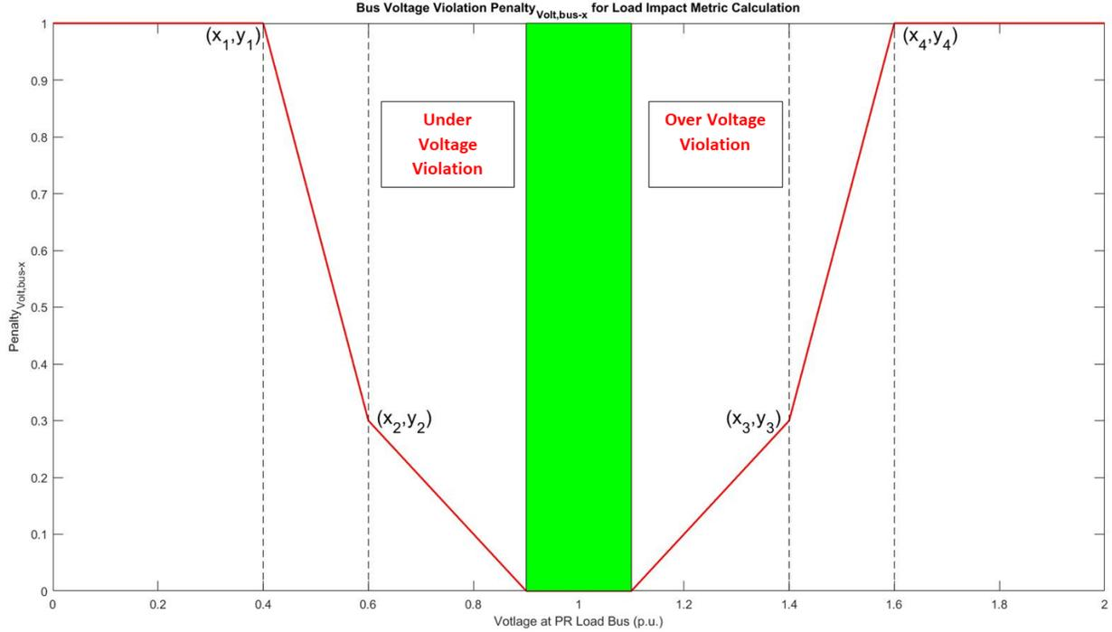
Figure 2-15: An illustration of load impact metric calculation.
