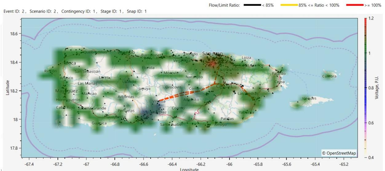
Figure 5-11: Voltage profile plotting for Contingency 1 in Hurricane Maria simulation with 2019 night peak preventive unloading case (corrective actions applied to 100 kV & Above systems) – figure generated by DCAT Analytics
