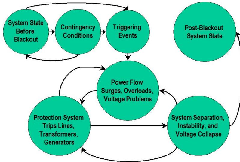
Figure 1-5: Generic cascade development scheme for DCAT, extracted from [7]
