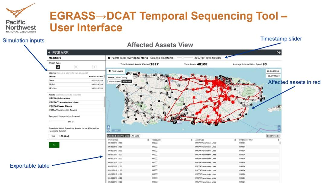
Figure 1-2: EGRASS adapted to provide temporal sequence of hurricane-related outages
