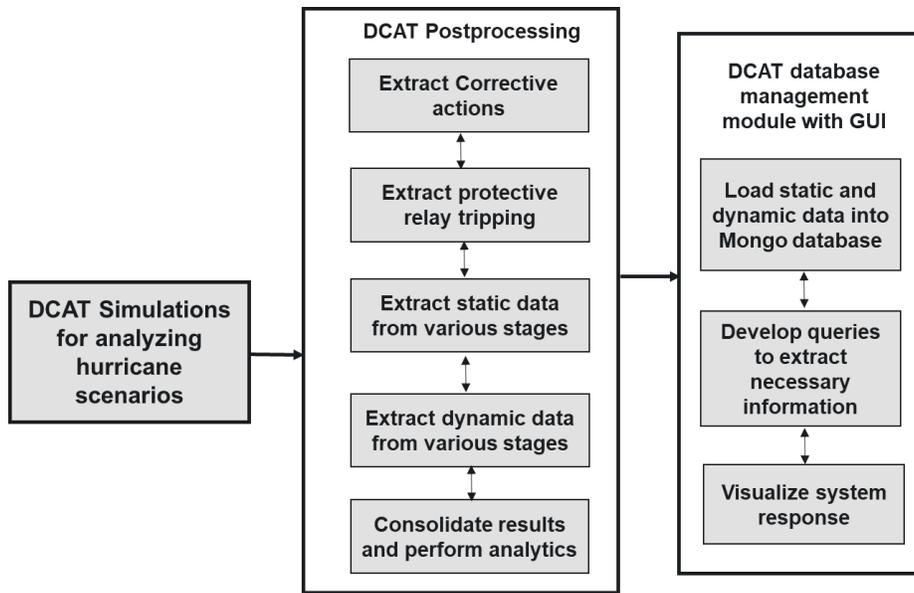
Figure 2-22. Complete automation capability for analyzing hurricane scenarios
