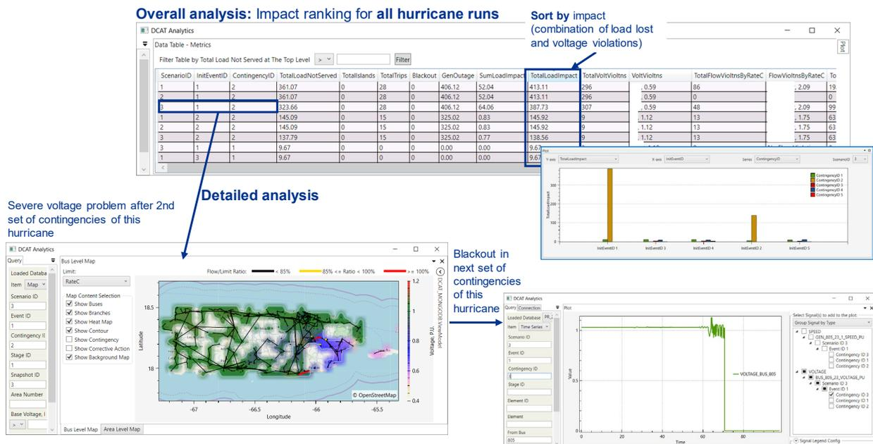
Figure 2-16: DCAT Automation, Analytics, and Data Management interface adapted and applied to hurricane contingencies and to Puerto Rico
