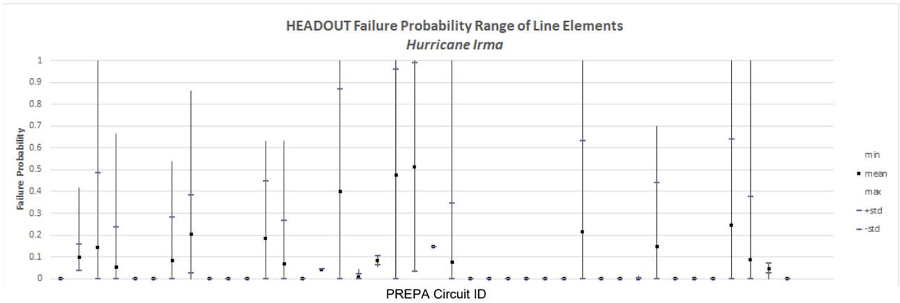
Figure A-3 HEADOUT failure probability range of line elements for Hurricane Irma
