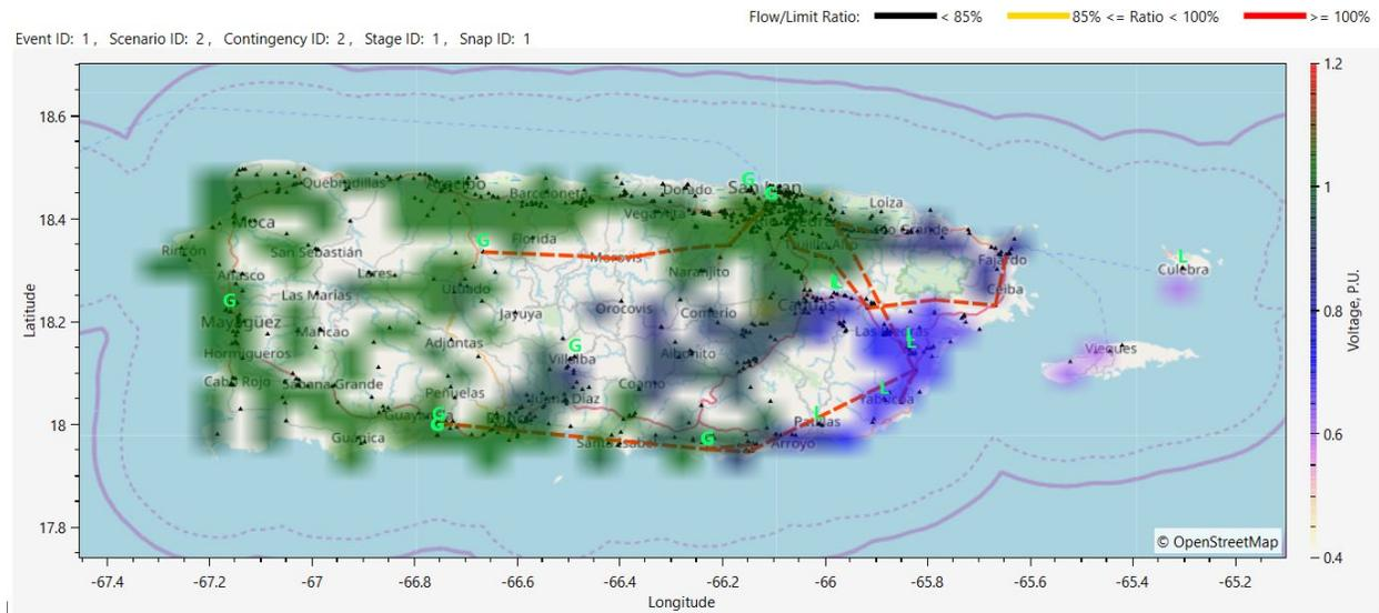
Figure 5-8: Voltage profile plotting for Contingency 2 in Hurricane Maria simulation with 2019 night peak case (corrective actions applied to 100 kV & Above systems) – figure generated by DCAT Analytics
