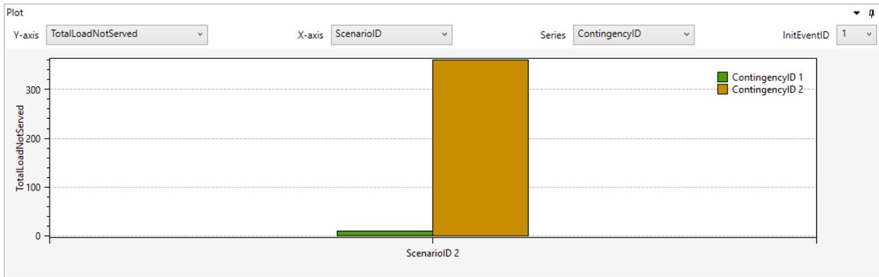
Figure 5-6: Total load not served in Hurricane Maria simulation with 2019 night peak case (corrective actions applied to 100 kV & Above systems) – figure generated by DCAT Analytics
