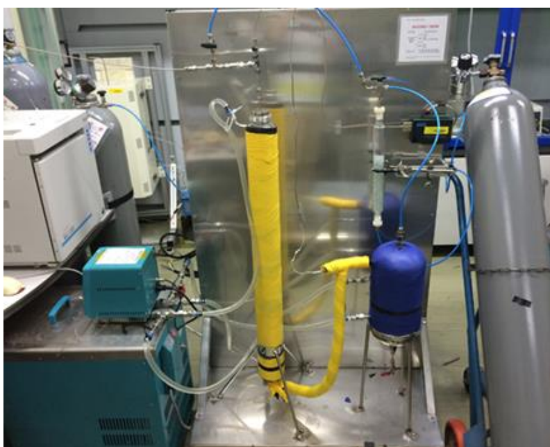
Figure 3. KAERI liquid cooled adsorbent testbed.
