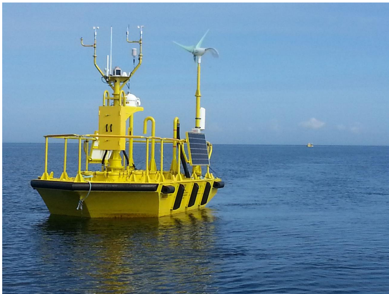
Figure 1.1. One of two AXYS WindSentinel buoys operated by PNNL for DOE.
