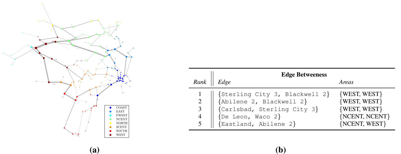
Figure 4.2. (a) Subgraph of the Texas 2000 network induced by edges with betweenness centrality score in at least the 90th percentile, (b) top 5 ranked edges according to edge-betweenness
