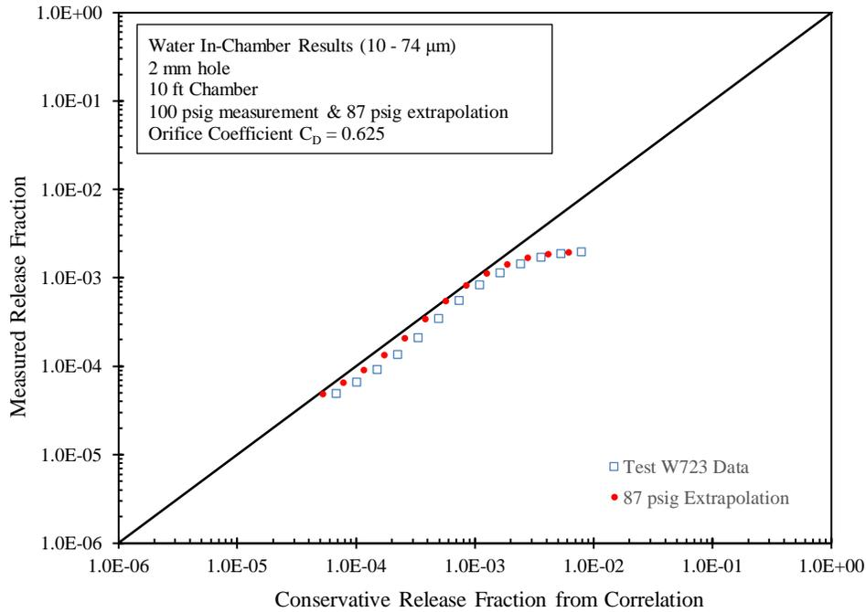
Figure 4.2. Extrapolation of 100-psig test data to 87-psig and 100-psig test data (Test W723 of Daniel et al. 2013) in comparison to the conservative  $R_C$  correlation with an orifice coefficient of  $C_D = 0.625$ .
