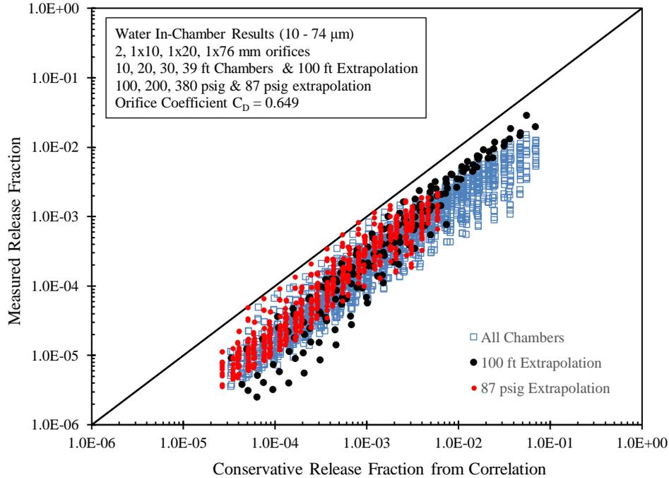
Figure 4.4. Measured release fractions and extrapolations in comparison to the conservative  $R_C$  correlation with an orifice coefficient of  $C_D = 0.649$ .
