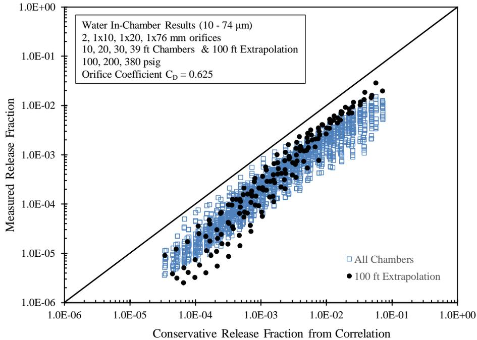
Figure 4.1. Measured release fractions compared to the conservative  $R_C$  correlation with an orifice coefficient of  $C_D = 0.625$ .
