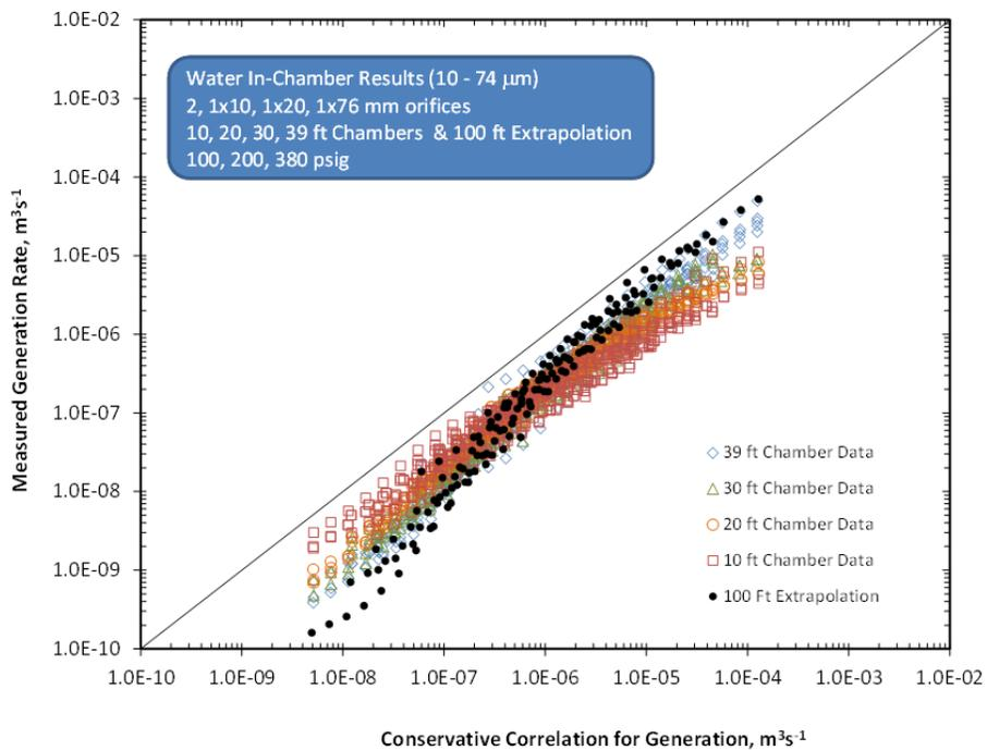
Figure 1.3. Results of previous study (Figure 10.20 of Daniel et al. 2013) showing a comparison of measured generation rates for individual tests and the 100-ft extrapolations with the conservative generation rate correlation  $GR_C$ .
