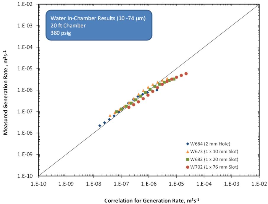
Figure 1.2. Results from the previous study (Figure 10.15 of Daniel et al. 2013) comparing individual test results for measured generation rates with a generation rate correlation given by a best fit correlation of the test data.
