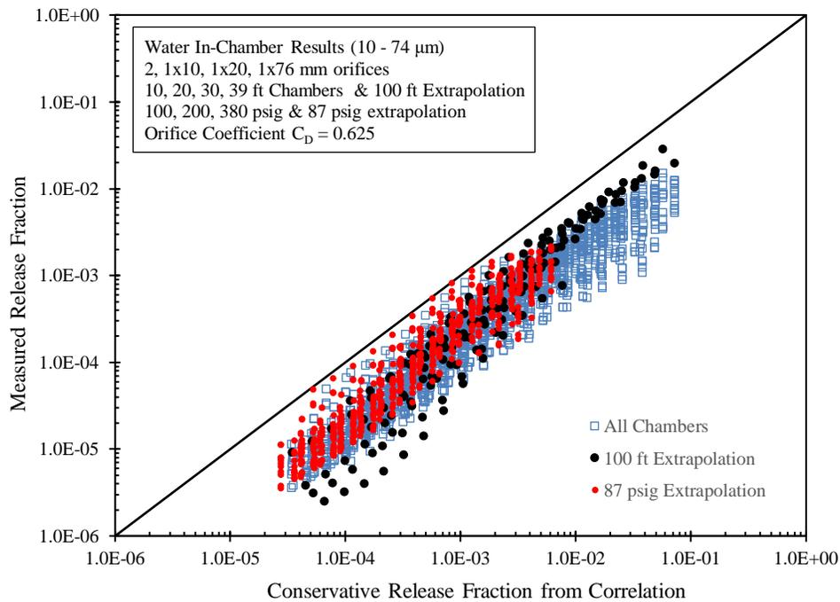
Figure 4.3. Measured release fractions and extrapolations in comparison to the conservative  $R_C$  correlation with an orifice coefficient of  $C_D = 0.625$ .
