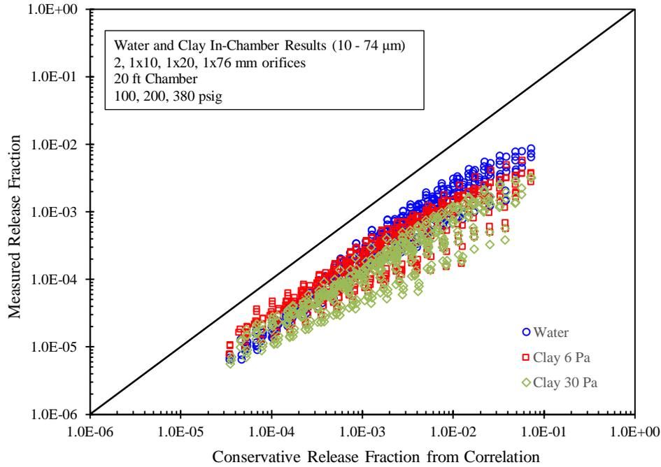
Figure 4.6. Measured release fractions for non-Newtonian slurries (6- and 30-Pa clays) compared with the conservative release fraction correlation  $R_C$ .
