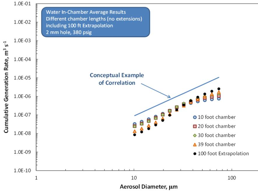
Figure 1.1. Results from the previous study (Figure 10.13 of Daniel et al. 2013) showing examples of test data and an extrapolation to a 100-ft chamber and a conceptual correlation that bounds the highest generation rate of all chamber sizes and the 100-ft chamber extrapolation for a 2-mm hole at 380 psig.
