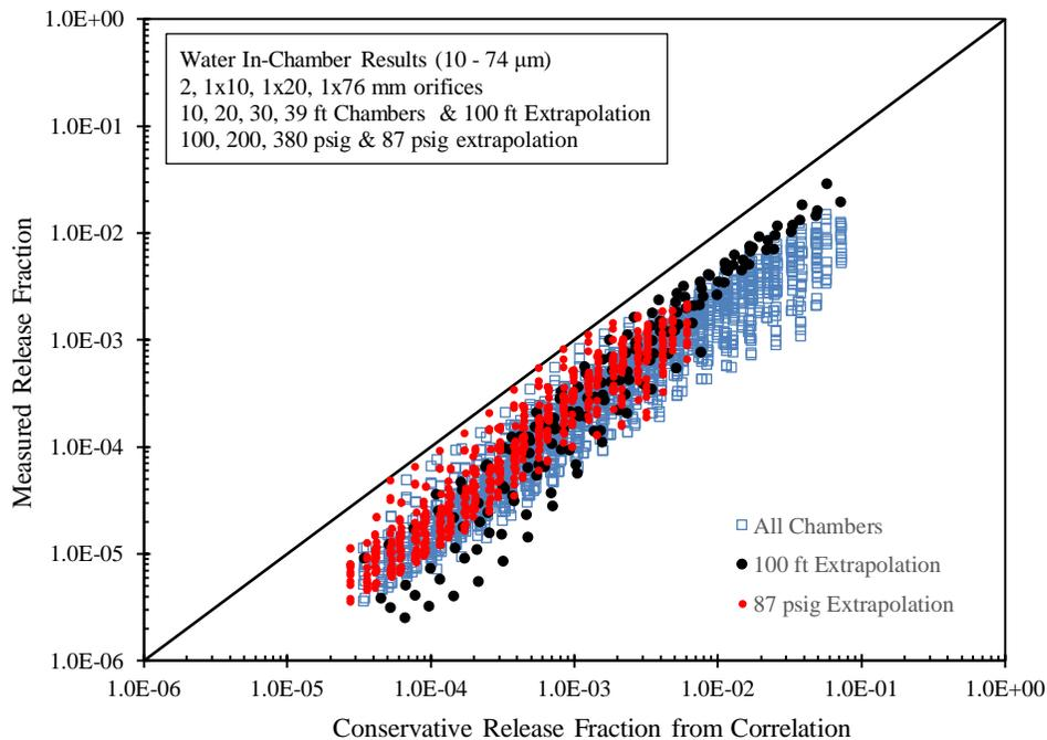
Figure 4.5. Comparison of all measured release fractions and extrapolations of test data to the final conservative  $R_C$  correlation.
