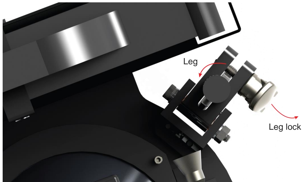
Figure 7. Detector leg removal, viewed from top of instrument looking downward.
