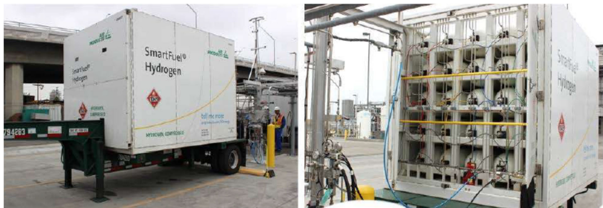
Figure 1. Exemplar CT-250 hydrogen tube trailer (from NTSB report)
