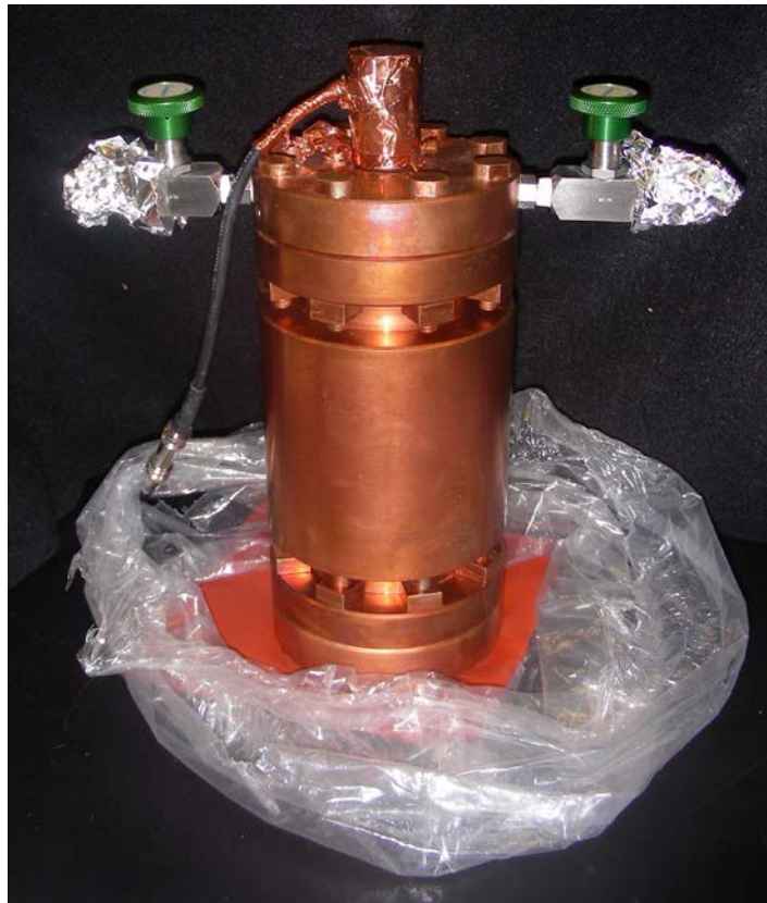
Figure 2. Large-Volume Prototype Proportional Counter (~0.64 L volume)
